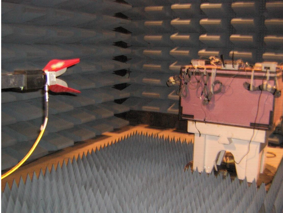
Figure 3: Radiated Emissions (above 1GHz) Test Setup
