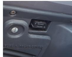
2. Attach the device to the vehicle's diagnostic port.
