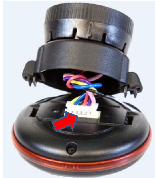
Part 1 and 2 are unlocked. Unplug the white connector
