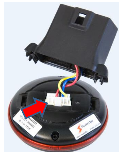
Plug the white connector on the module. Attention to the correct position
