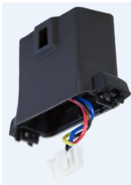
Plug the white connector on the module. Attention to the correct position
