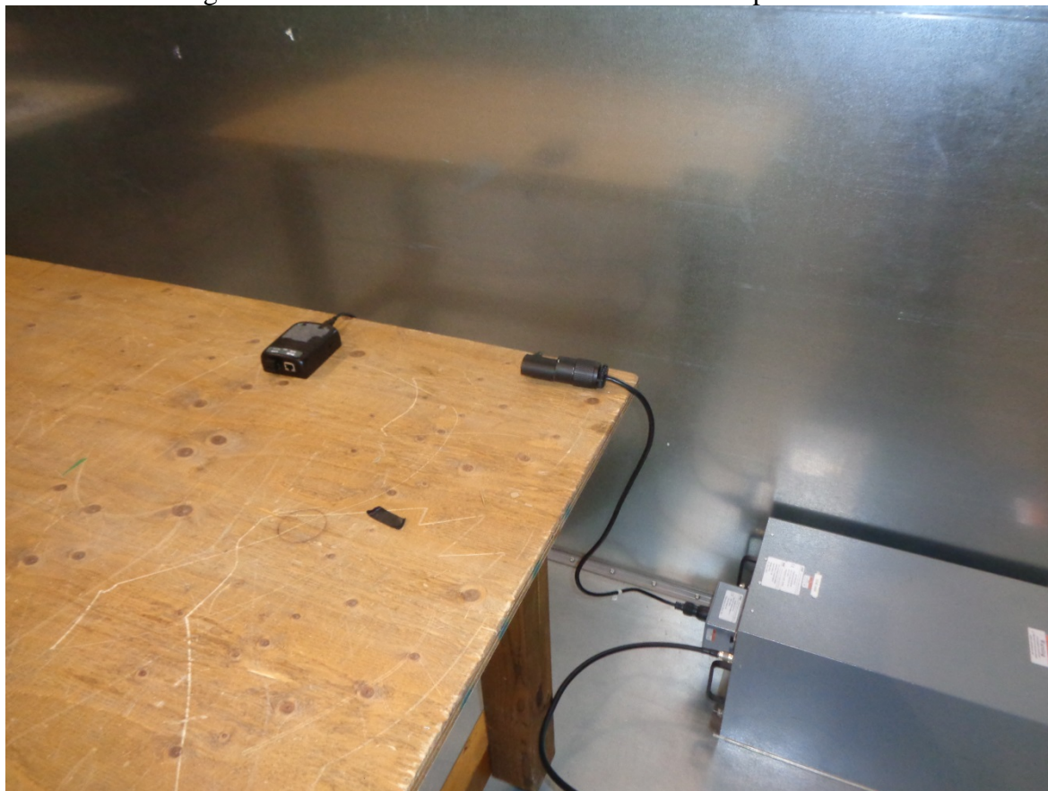
Figure 5 – Power Line Conducted Emissions Setup – Photo 2
