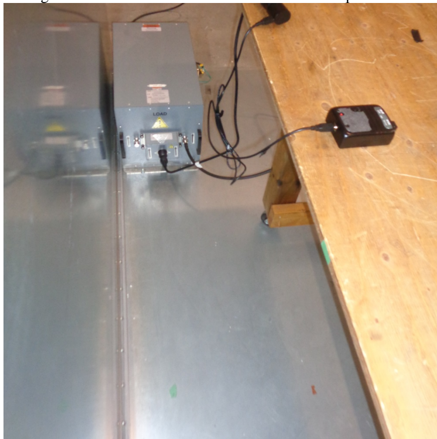
Figure 4 – Power Line Conducted Emissions Setup – Photo 1
