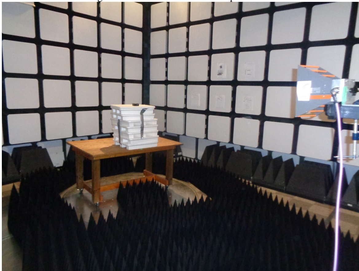
Figure 3 – Radiated Emissions Setup – Photo 3
