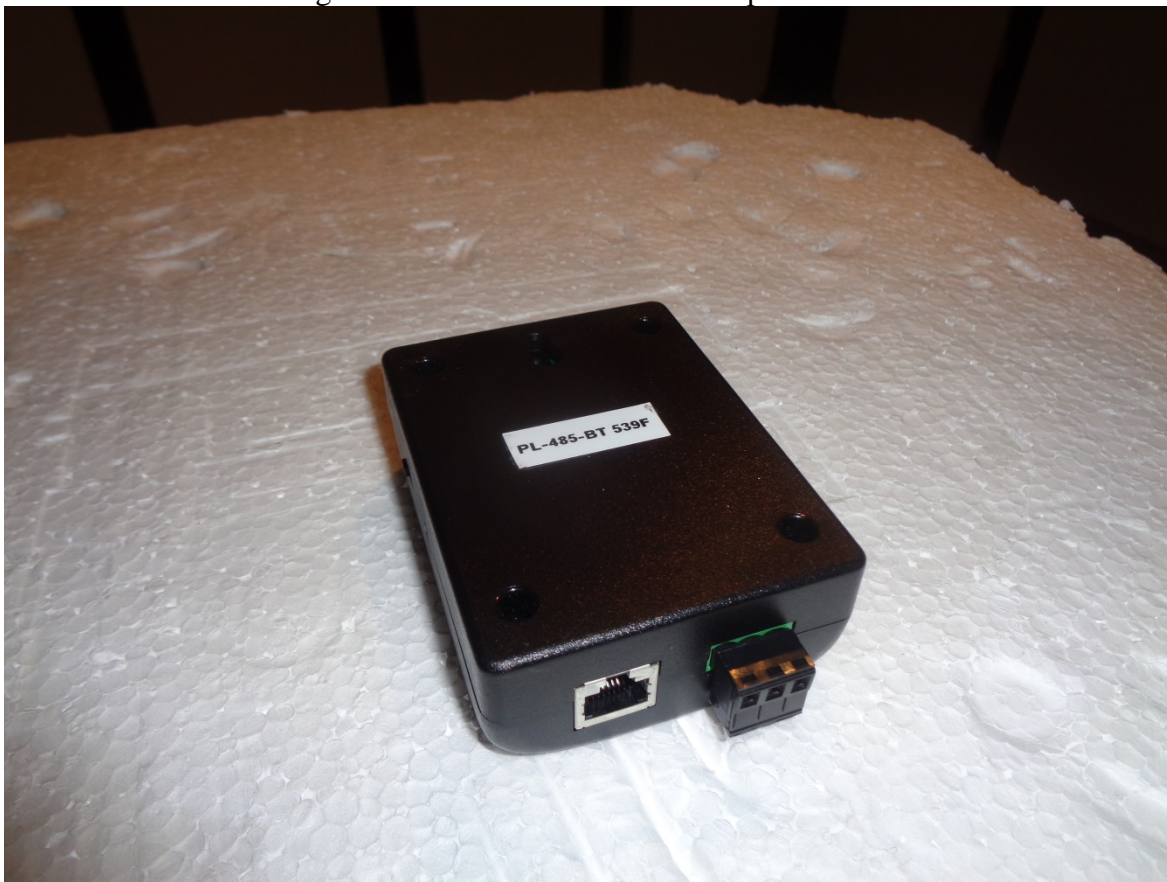
Figure 2 – Radiated Emissions Setup – Photo 2
