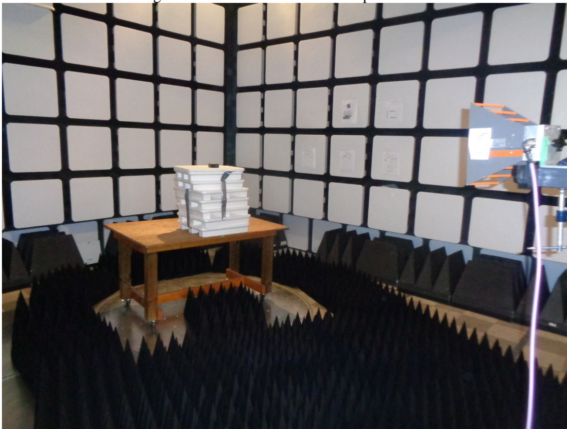
Figure 3 – Radiated Emissions Setup – Photo 3
