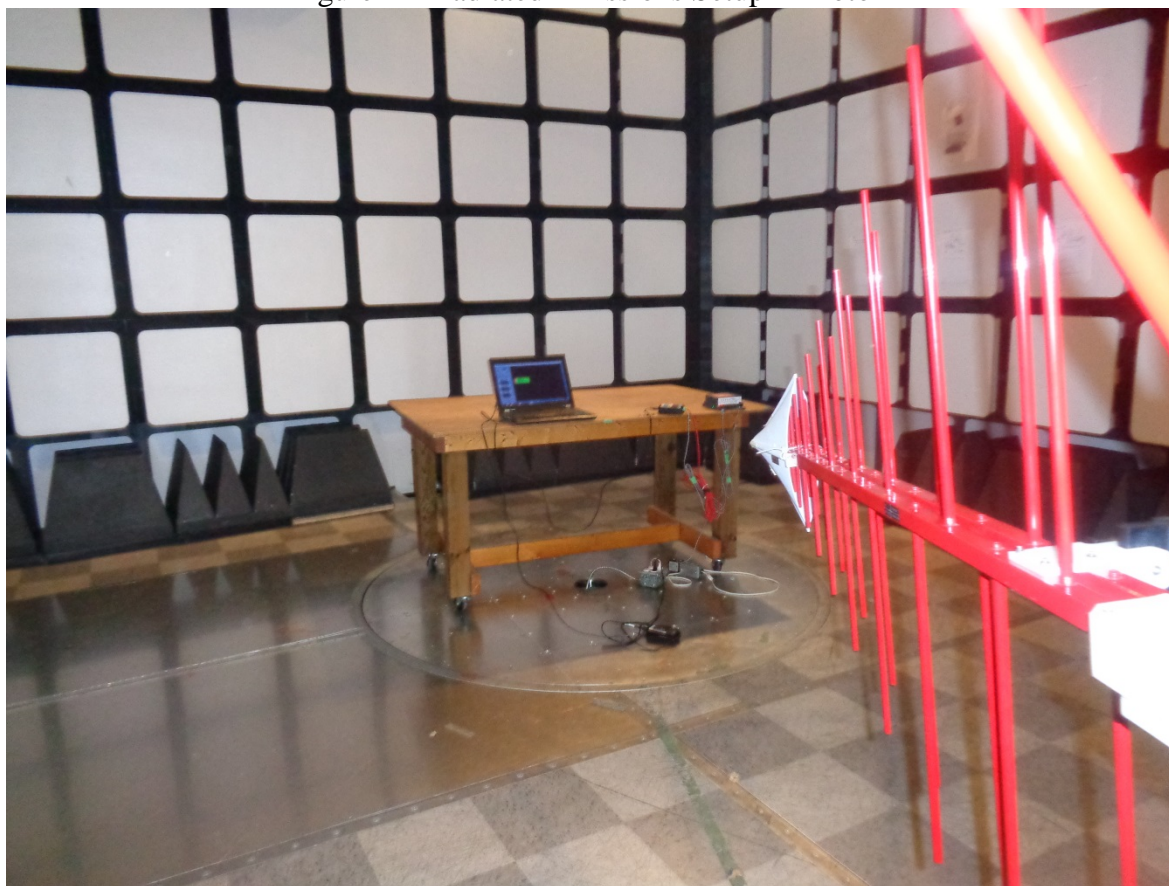
Figure 1 – Radiated Emissions Setup – Photo 1
