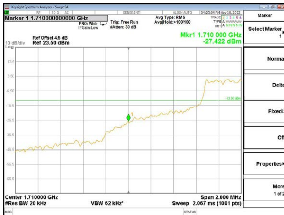
Band4-Low Channel-10MHz Bandwidth-5RB-16QAM
