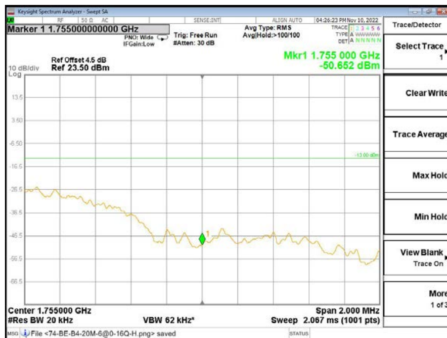
Band4-High Channel-20MHz Bandwidth-6RB-QPSK
