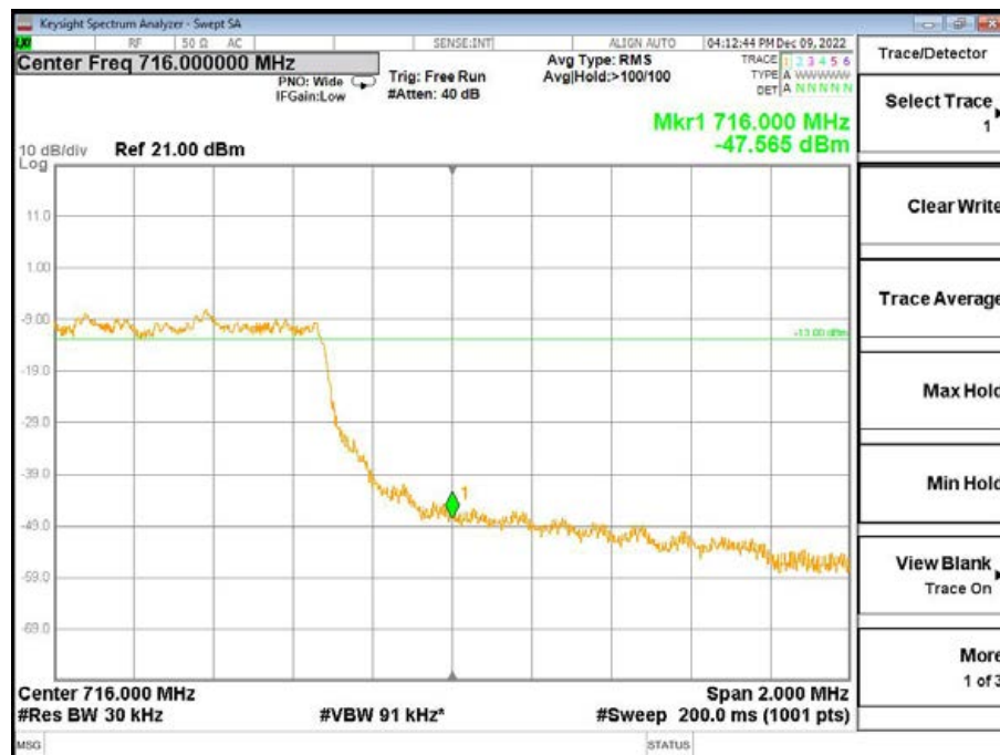
High Channel-3MHz Bandwidth-6RB-QPSK
