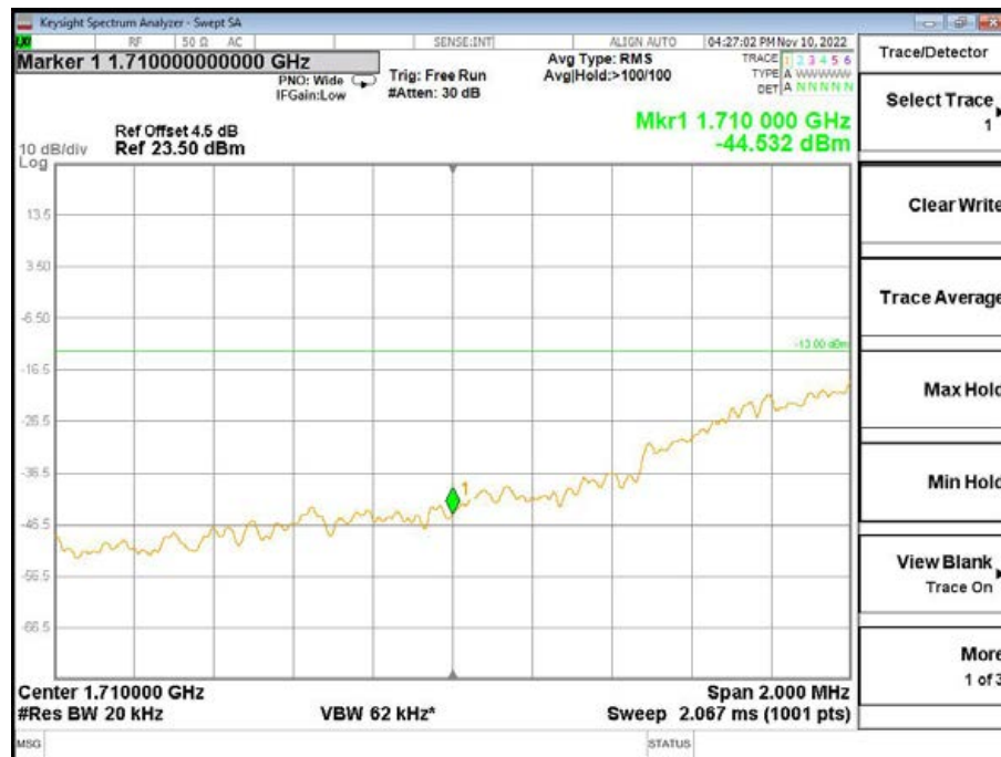
Band4-Low Channel-20MHz Bandwidth-5RB-16QAM
