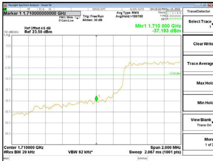
Band4-Low Channel-3MHz Bandwidth-6RB-QPSK
