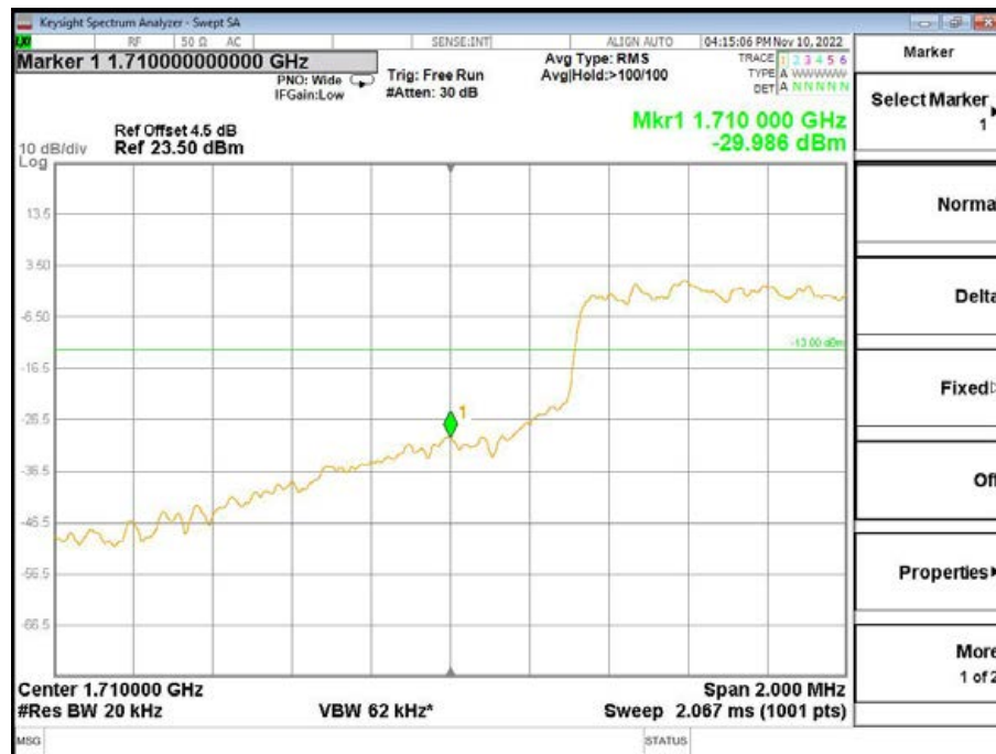
Band4-Low Channel-3MHz Bandwidth-5RB-16QAM
