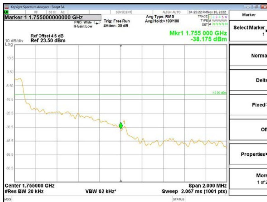
Band4-High Channel-15MHz Bandwidth-6RB-QPSK
