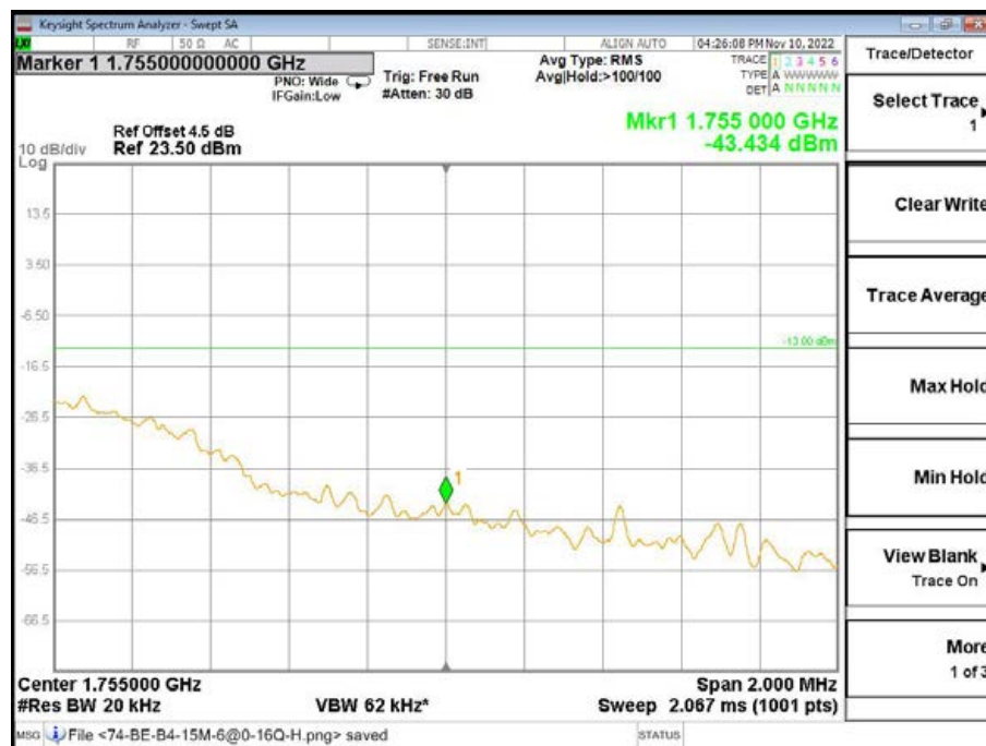
Band4-High Channel-20MHz Bandwidth-5RB-16QAM
