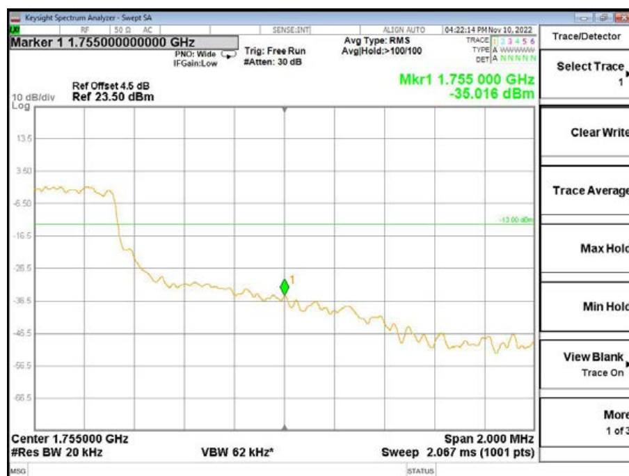
Band4-High Channel-10MHz Bandwidth-6RB-QPSK
