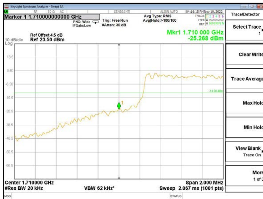
Band4-Low Channel-5MHz Bandwidth-5RB-16QAM
