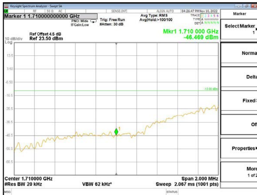
Band4-Low Channel-20MHz Bandwidth-6RB-QPSK
