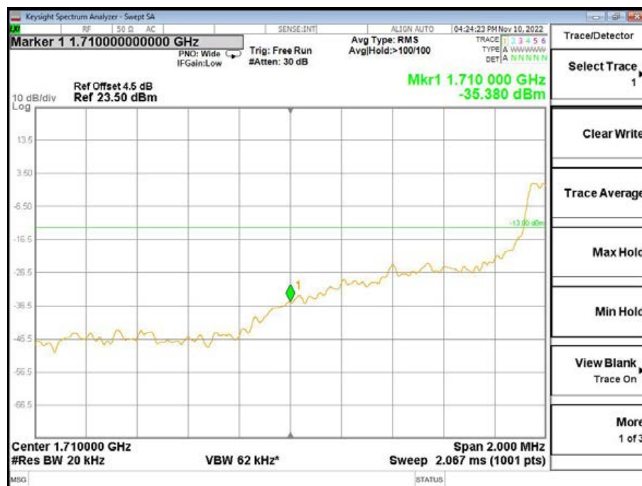
Band4-Low Channel-15MHz Bandwidth-6RB-QPSK
