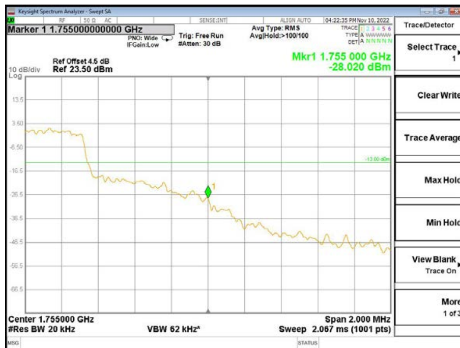
Band4-High Channel-10MHz Bandwidth-5RB-16QAM
