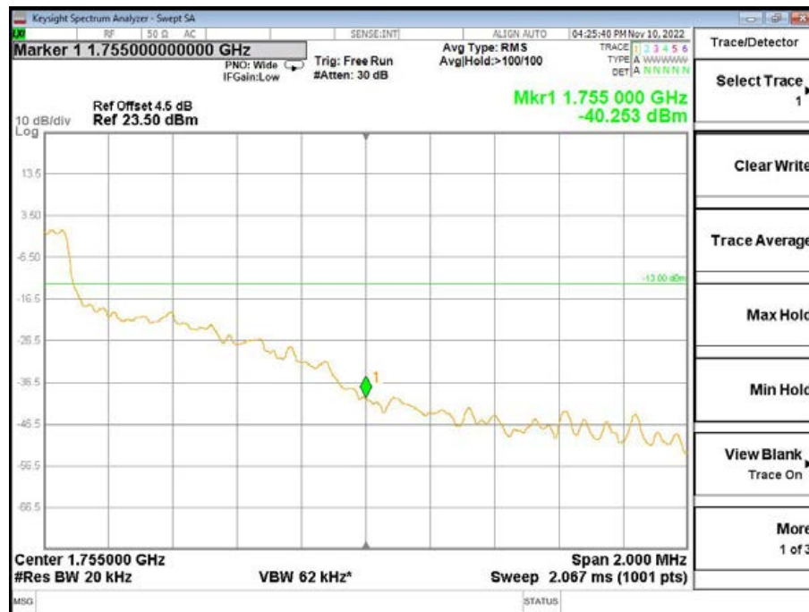
Band4-High Channel-15MHz Bandwidth-5RB-16QAM
