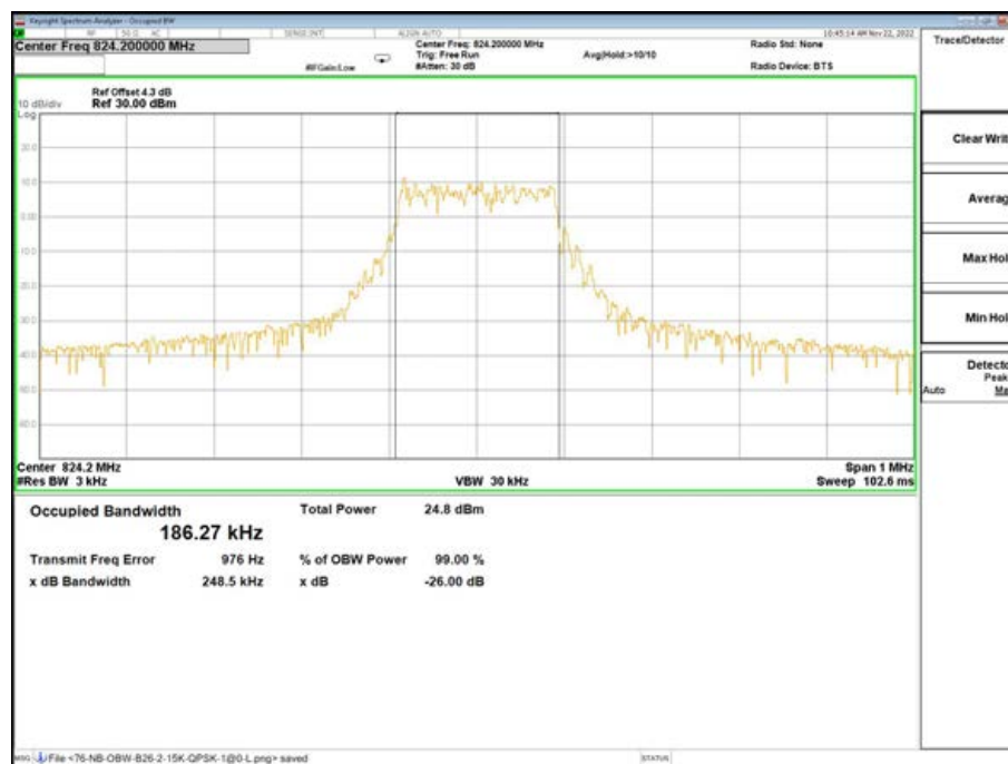
Band26-26dB/99% OBW-26792 Channel-QPSK-12@0-15K
