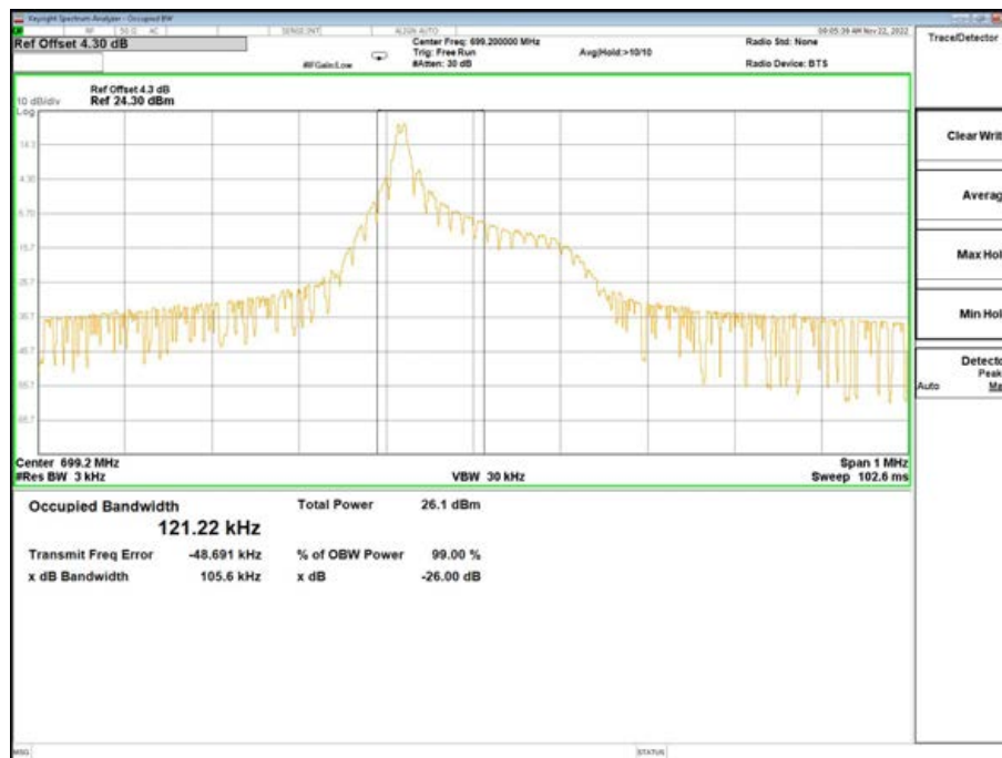
Band12-26dB/99% OBW-23012 Channel-BPSK-1@0-15K
