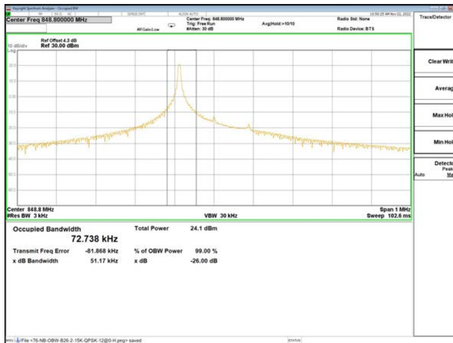
Band26-26dB/99% OBW-27038 Channel-BPSK-1@0-3.75K
