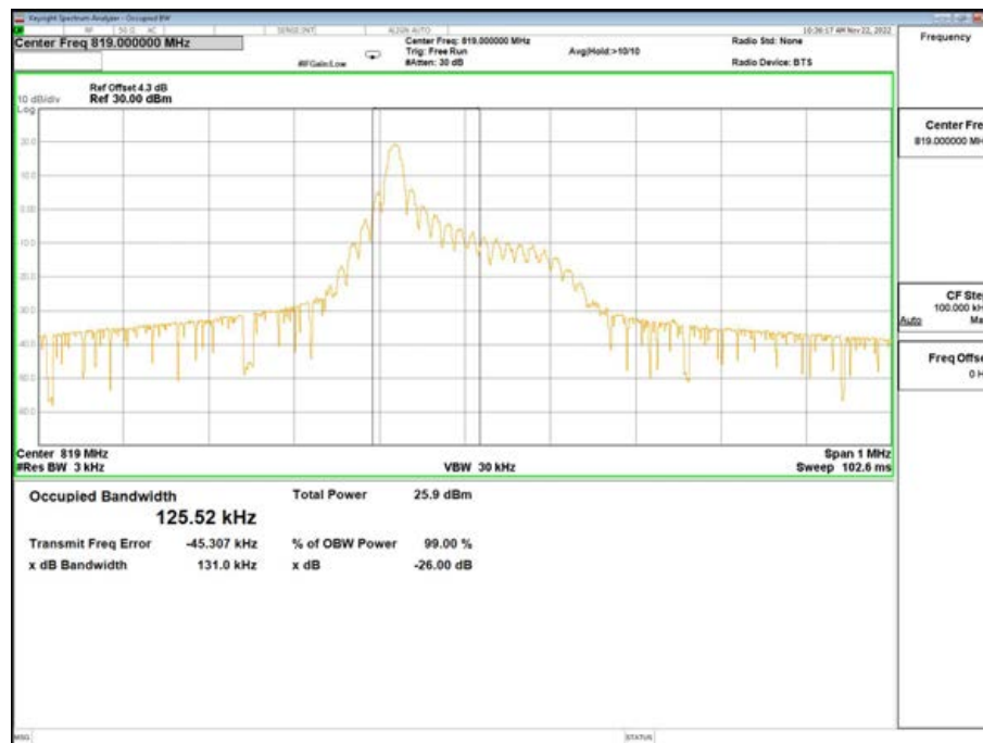
Band26-26dB/99% OBW-26740 Channel-QPSK-1@0-15K
