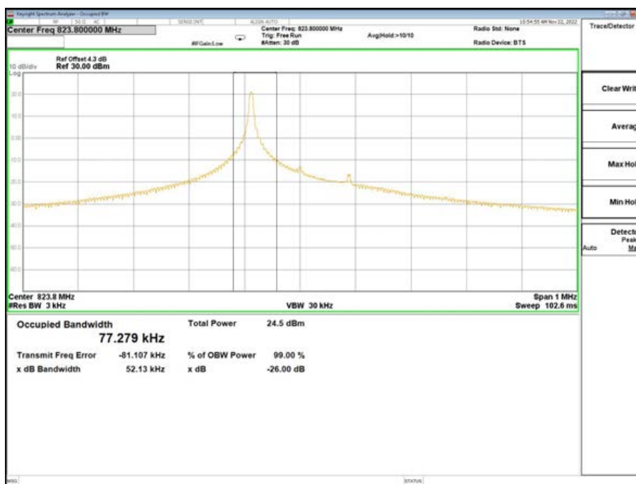
Band26-26dB/99% OBW-26788 Channel-BPSK-1@0-3.75K
