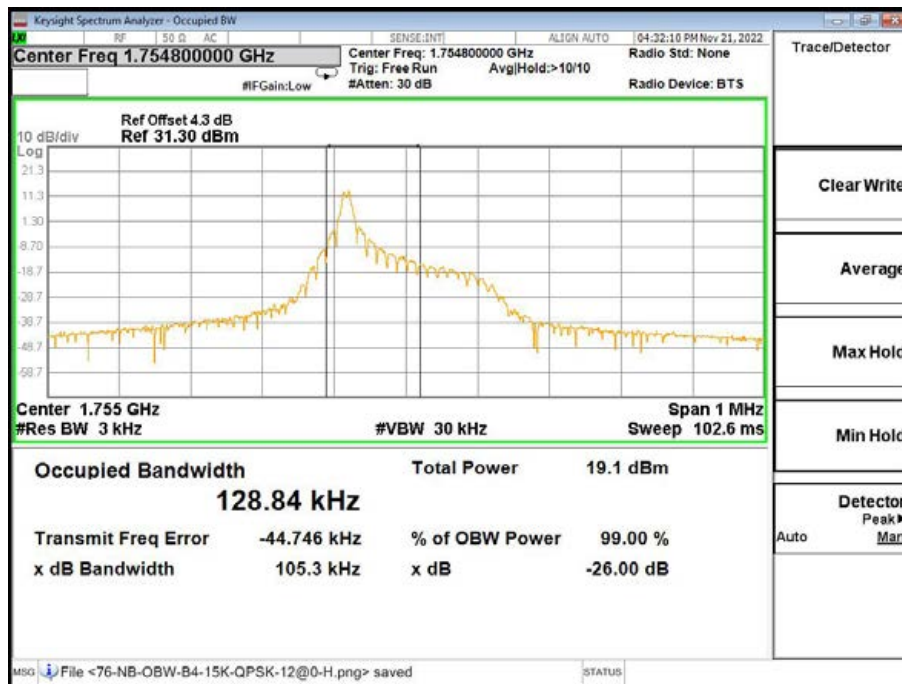
Band4-26dB/99% OBW-20398 Channel-BPSK-1@0-15K
