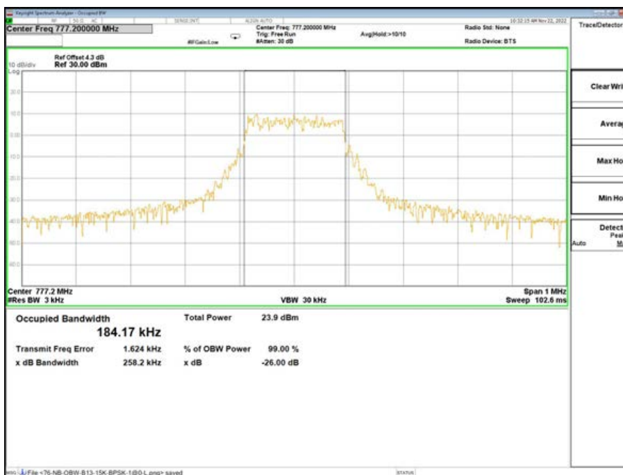
Band13-26dB/99% OBW-23182 Channel-QPSK-12@0-15K
