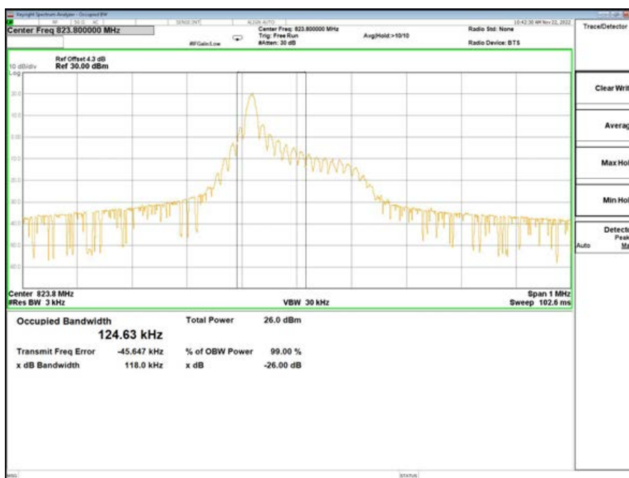
Band26-26dB/99% OBW-26788 Channel-QPSK-1@0-15K
