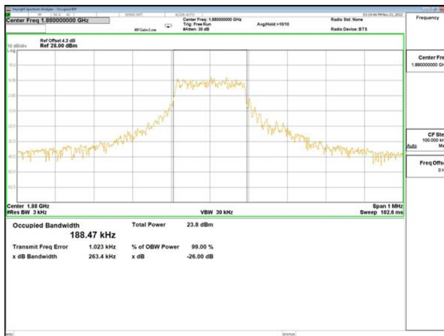
Band2-26dB/99% OBW-18900 Channel-QPSK-12@0-15K
