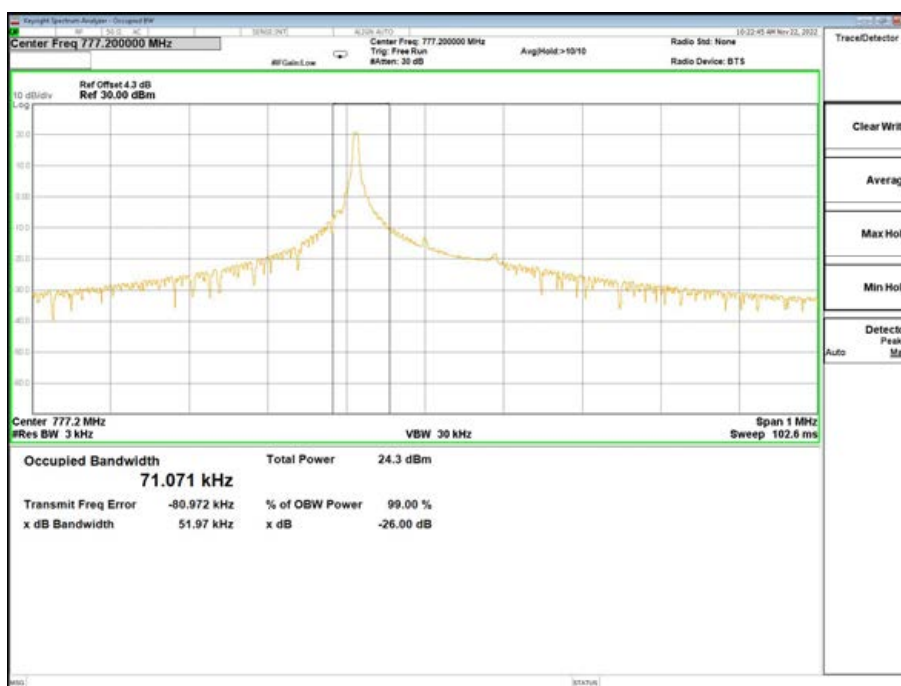
Band13-26dB/99% OBW-23182 Channel-BPSK-1@0-3.75K
