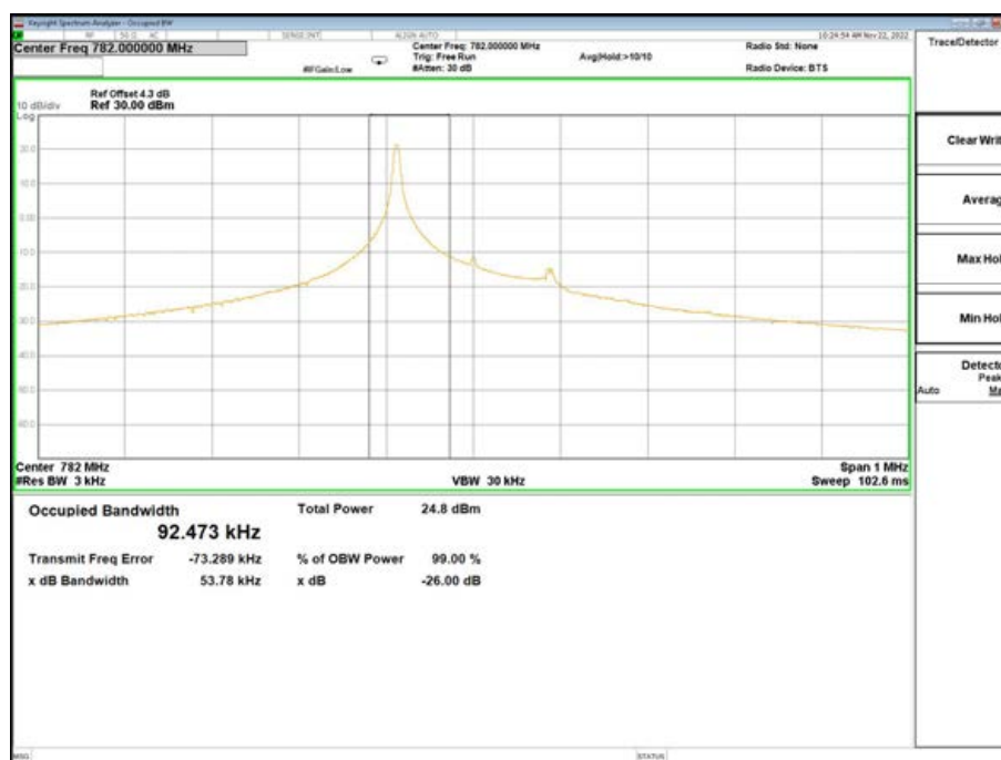
Band13-26dB/99% OBW-23230 Channel-QPSK-1@0-3.75K
