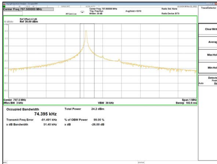
Band12-26dB/99% OBW-23095 Channel-BPSK-1@0-3.75K
