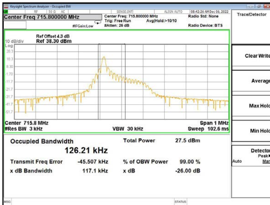
Band12-26dB/99% OBW-23178 Channel-QPSK-1@0-15K
