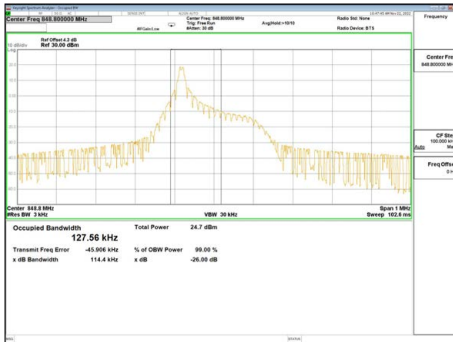
Band26-26dB/99% OBW-27038 Channel-BPSK-1@0-15K
