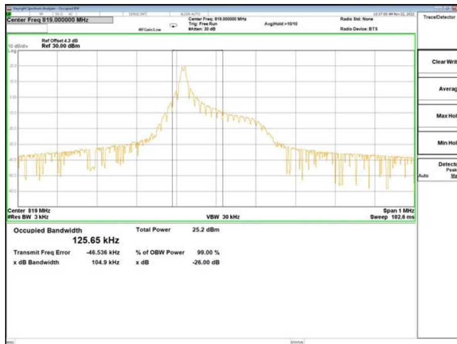
Band26-26dB/99% OBW-26740 Channel-BPSK-1@0-15K
