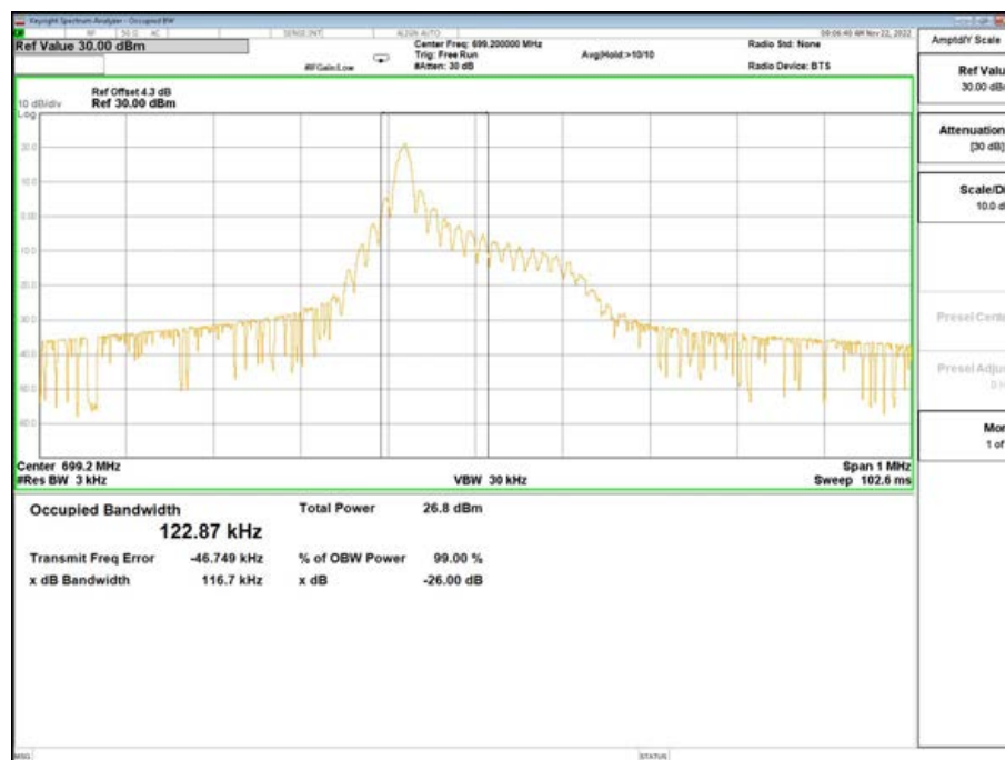
Band12-26dB/99% OBW-23012 Channel-QPSK-1@0-15K
