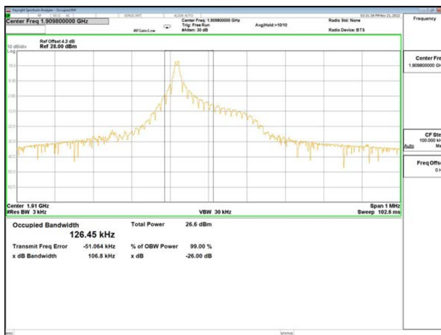
Band2-26dB/99% OBW-19198 Channel-QPSK-1@0-15K
