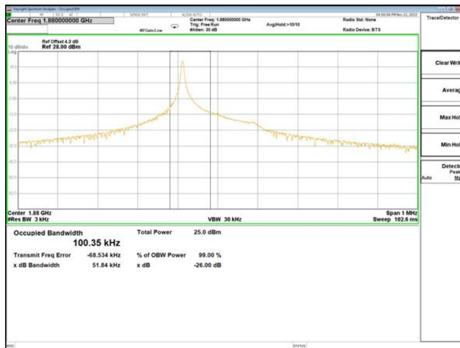
Band2-26dB/99% OBW-18900 Channel-QPSK-1@0-3.75K
