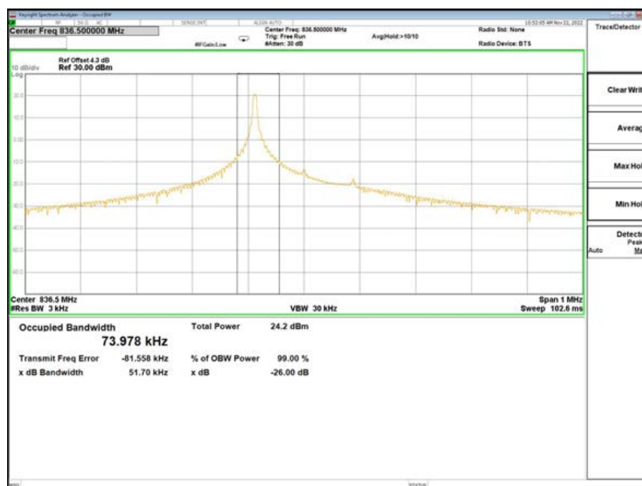
Band26-26dB/99% OBW-26915 Channel-BPSK-1@0-3.75K
