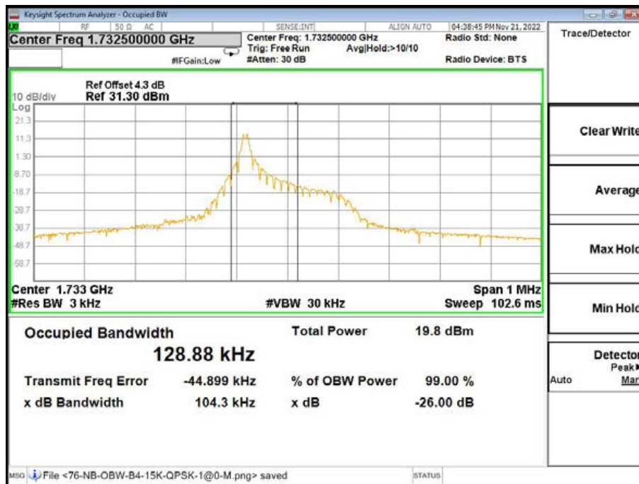
Band4-26dB/99% OBW-20175 Channel-BPSK-1@0-15K
