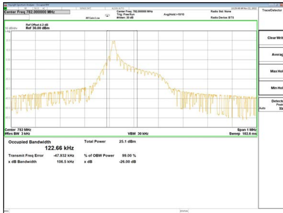
Band13-26dB/99% OBW-23230 Channel-BPSK-1@0-15K
