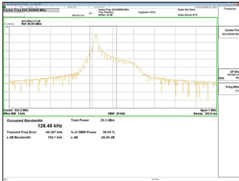
Band26-26dB/99% OBW-26792 Channel-BPSK-1@0-15K
