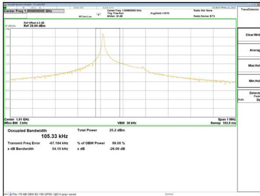
Band2-26dB/99% OBW-19198 Channel-QPSK-1@0-3.75K
