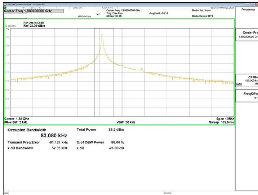
Band2-26dB/99% OBW-18900 Channel-BPSK -1@0-3.75K
