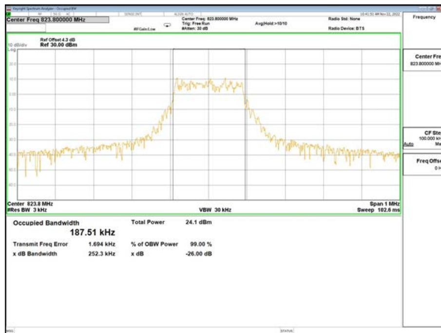
Band26-26dB/99% OBW-26788 Channel-QPSK-12@0-15K
