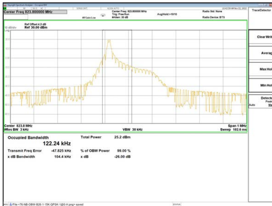
Band26-26dB/99% OBW-26788 Channel-BPSK-1@0-15K
