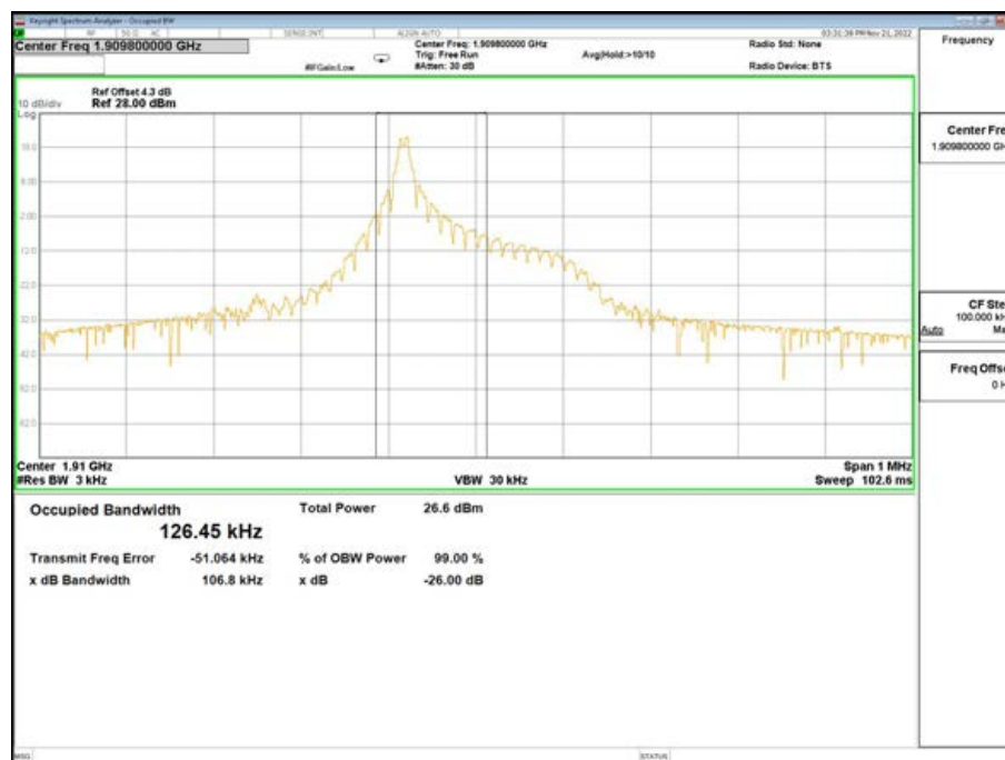
Band2-26dB/99% OBW-19198 Channel-BPSK-1@0-15K
