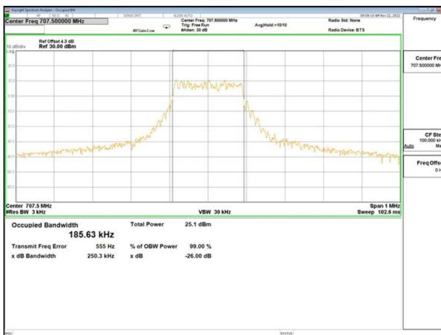
Band12-26dB/99% OBW-23095 Channel-QPSK-12@0-15
