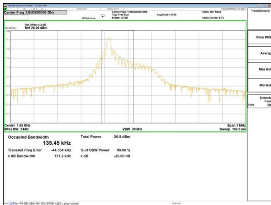
Band2-26dB/99% OBW-18602 Channel-QPSK-1@0-15K
