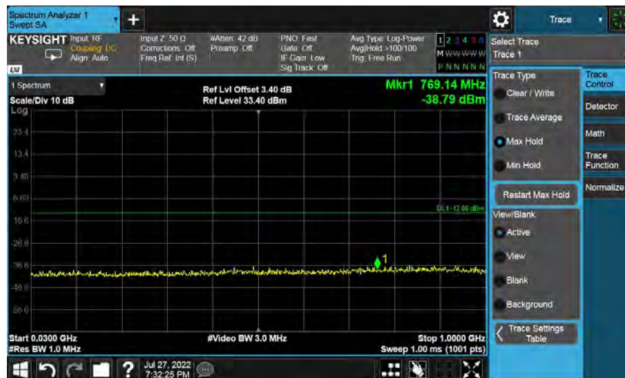
Band2-Low Channel-3MHz Bandwidth-30MHz to 1GHz
