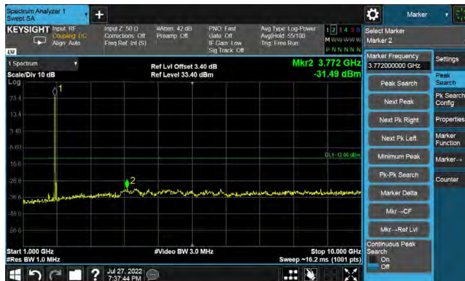
Band2-Low Channel-5MHz Bandwidth-1GHz to 10GHz
