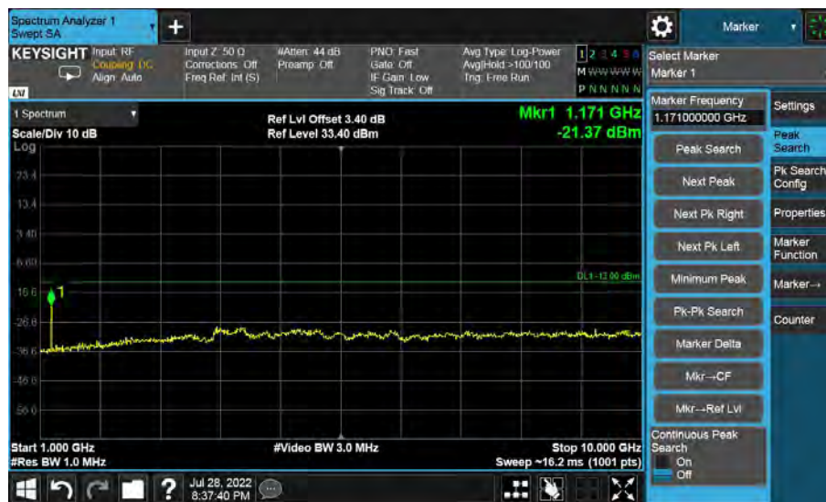
Low Channel-10MHz Bandwidth-1GHz to 10GHz
