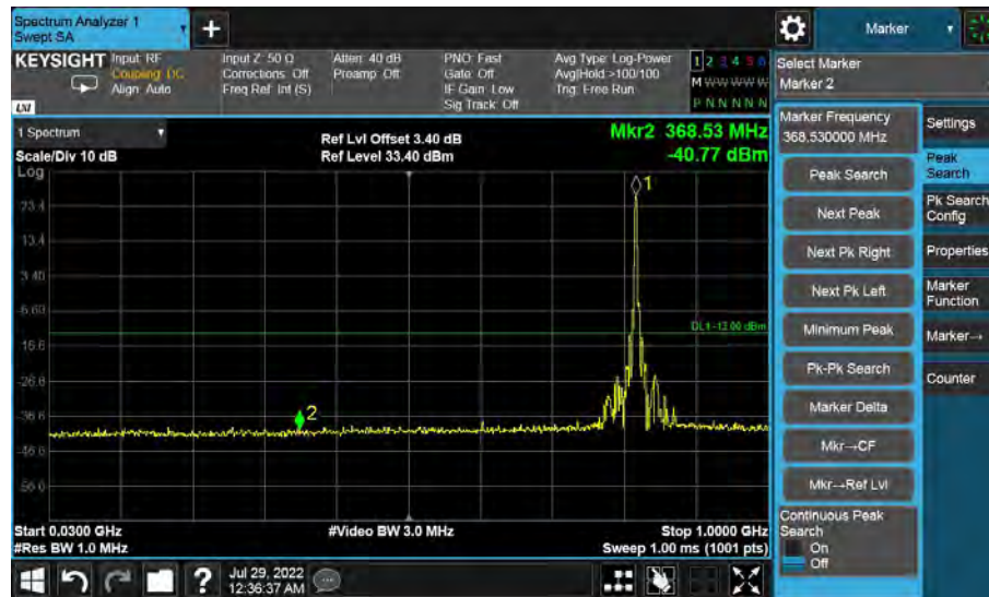
High Channel-3MHz Bandwidth-30MHz to 1GHz
