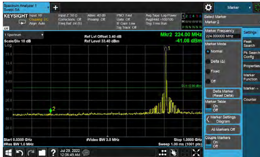
Low Channel-5MHz Bandwidth-30MHz to 1GHz
