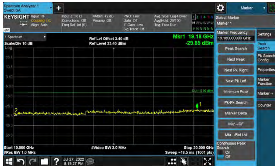
Band2-Middle Channel-5MHz Bandwidth-10GHz to 20GHz
