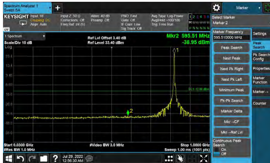
Low Channel-3MHz Bandwidth-30MHz to 1GHz
