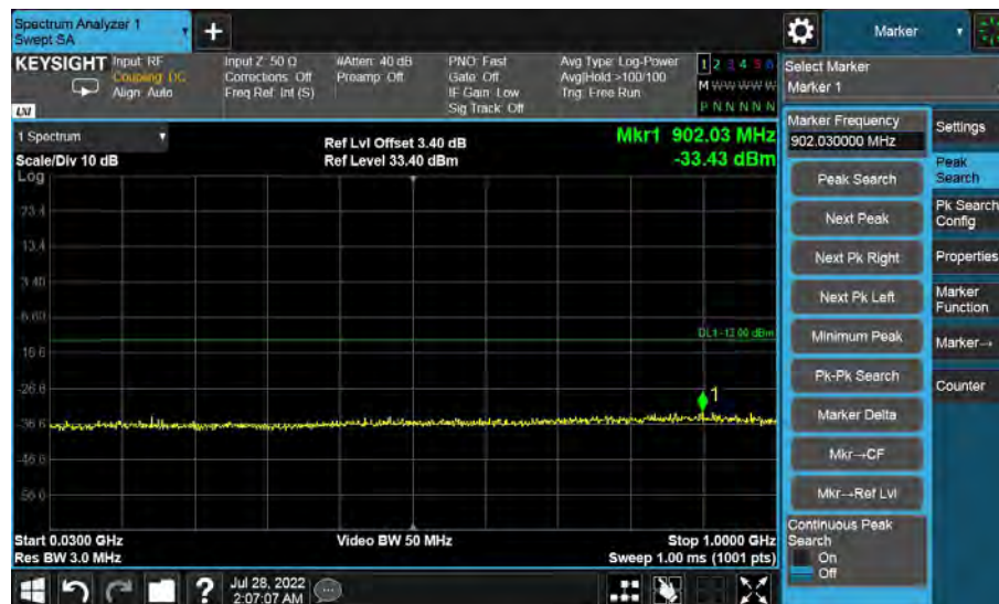
Band4-High Channel-10MHz Bandwidth-30MHz to 1GHz
