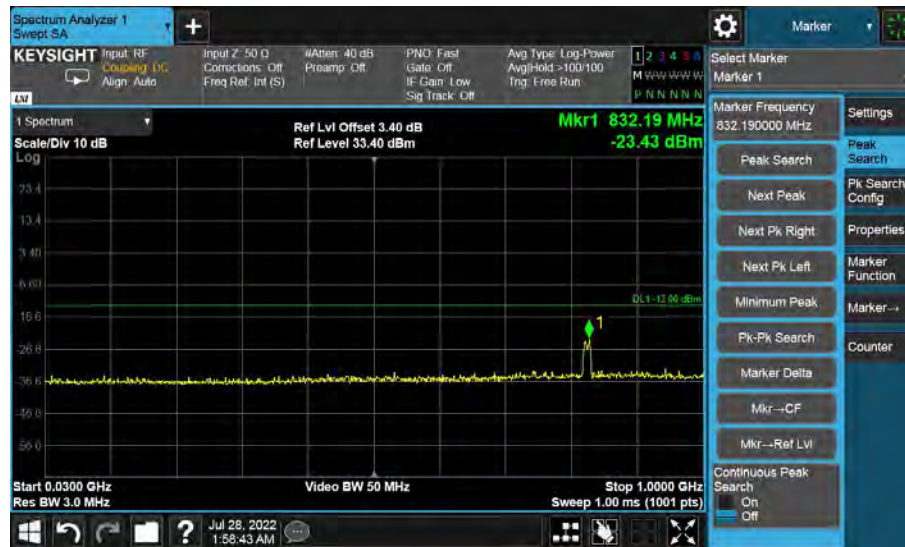
Band4-High Channel-5MHz Bandwidth-30MHz to 1GHz
