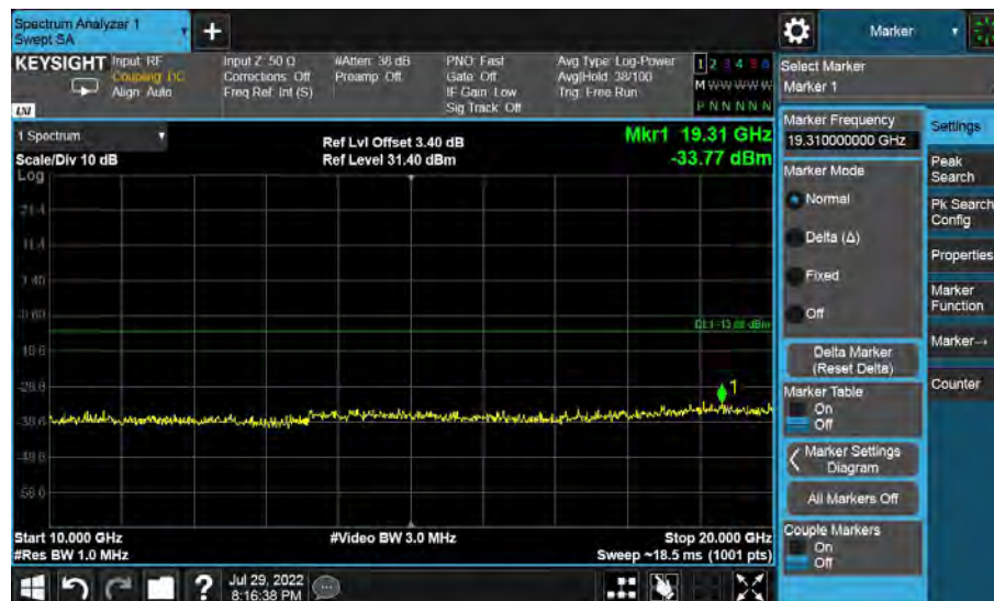
10GHz to 20GHz, High Channel, Subcarrier (15kHz), BPSK, 1@0
