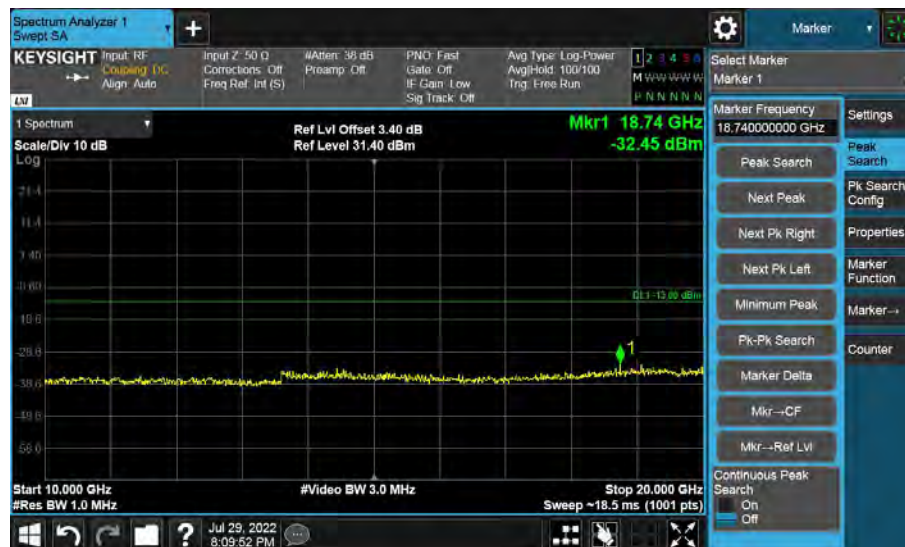
10GHz to 20GHz, Low Channel, Subcarrier (15kHz), QPSK, 1@0
