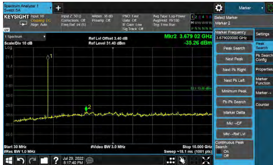
30MHz to 10GHz, High Channel, Subcarrier (15kHz), QPSK, 1@0
