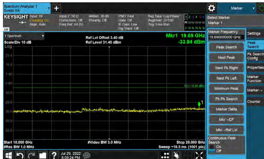
10GHz to 20GHz, Low Channel, Subcarrier (15kHz), BPSK, 1@0
