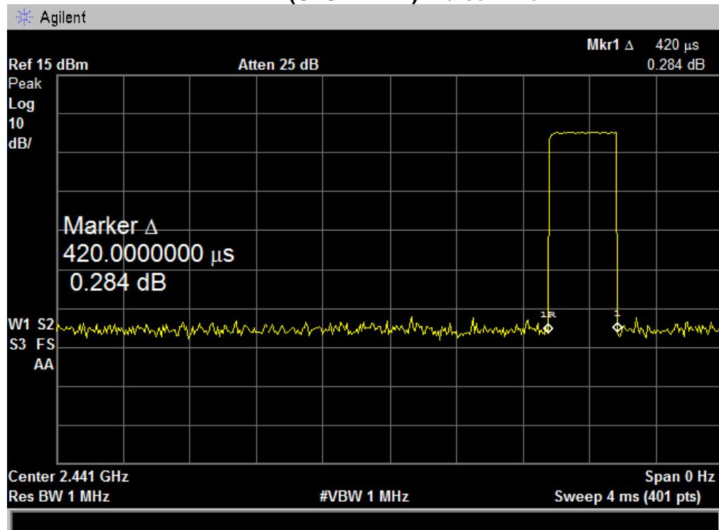
**2441 MHz (GFSK 1DH3)- Pulse Time**
