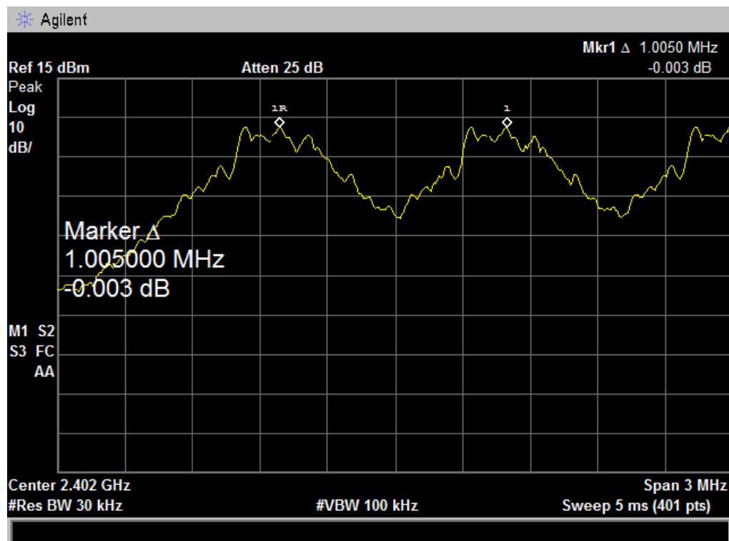
**2441 MHz(GFSK)-Channel Separation**
