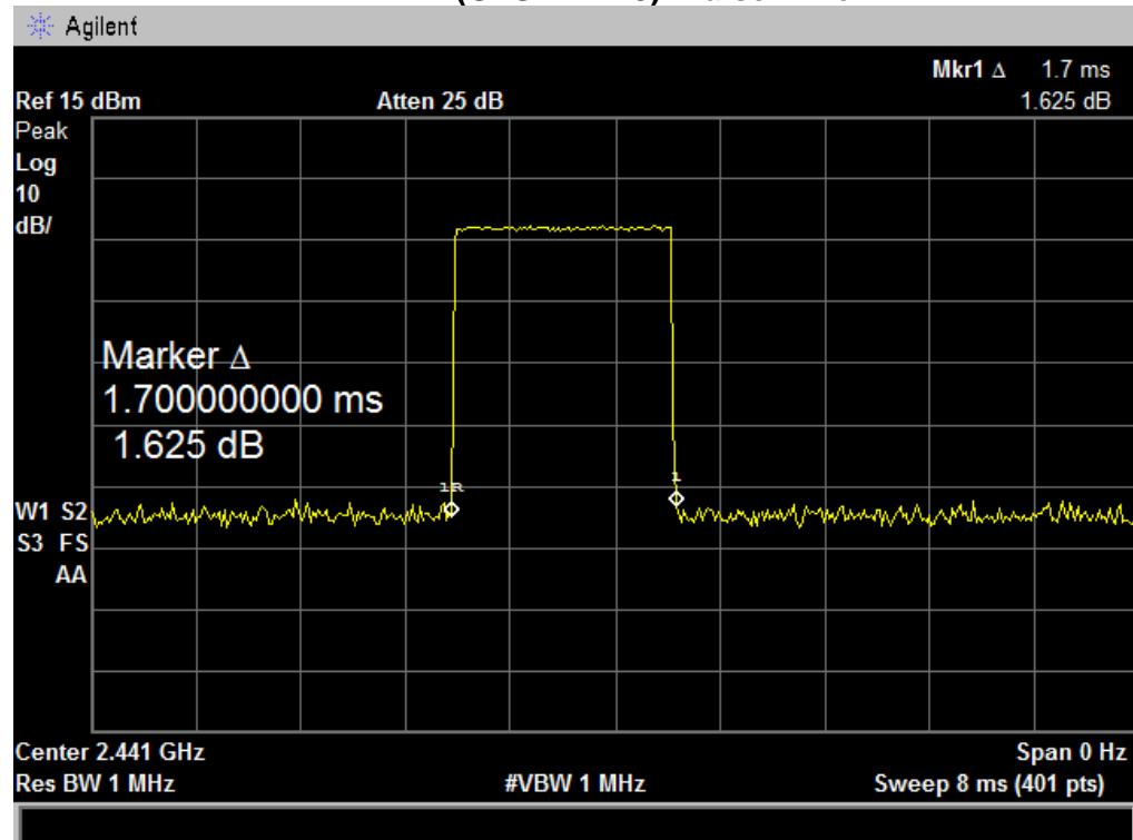
**2441 MHz (GFSK 1DH5)- Pulse Time**
