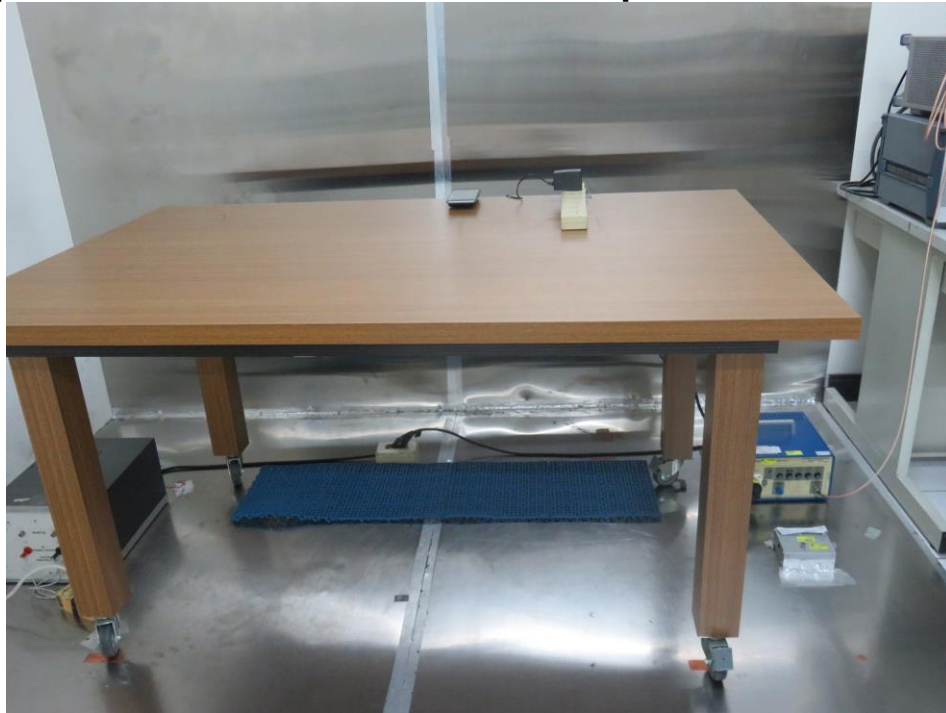
Photograph –Conducted Emission Test Setup
