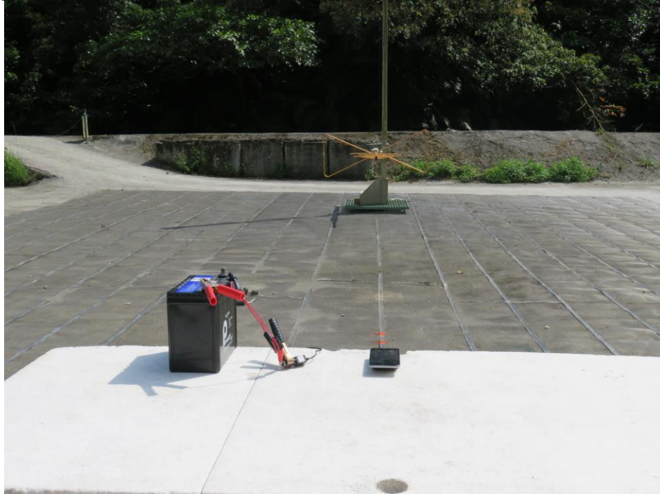
Photograph – Radiated Emission Test Setup- Below 1G
