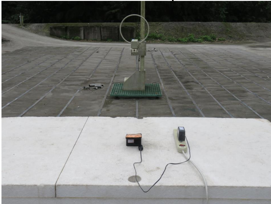
Photograph – Radiated Emission Test Setup
