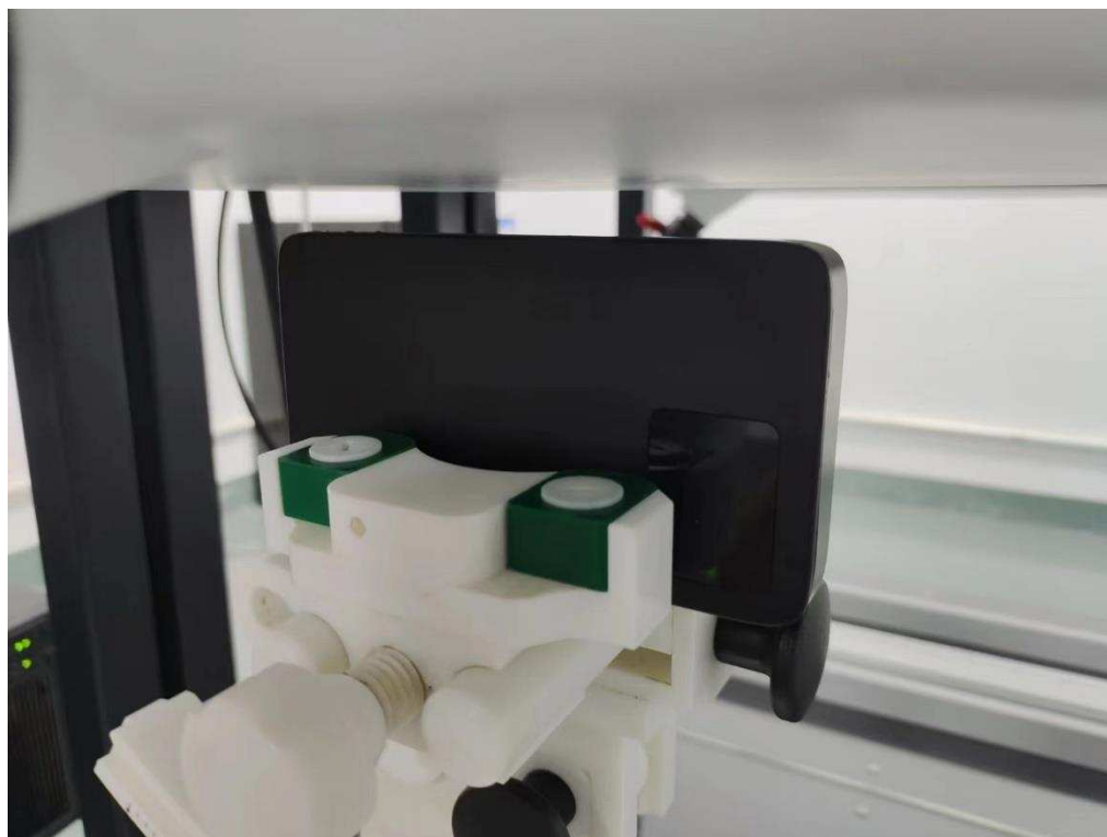
Body Left side (separation distance is 10mm)
