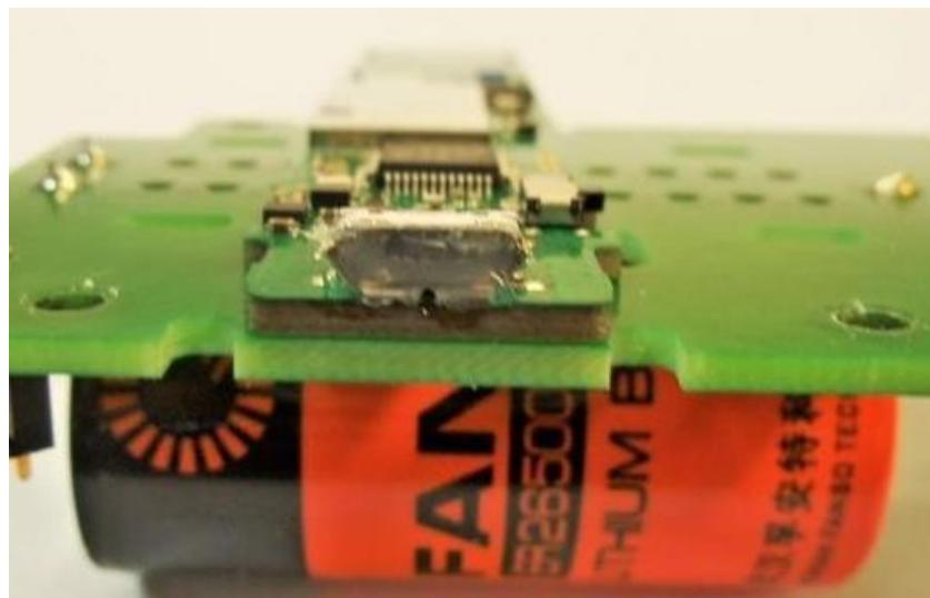
Jumper soldered on top
