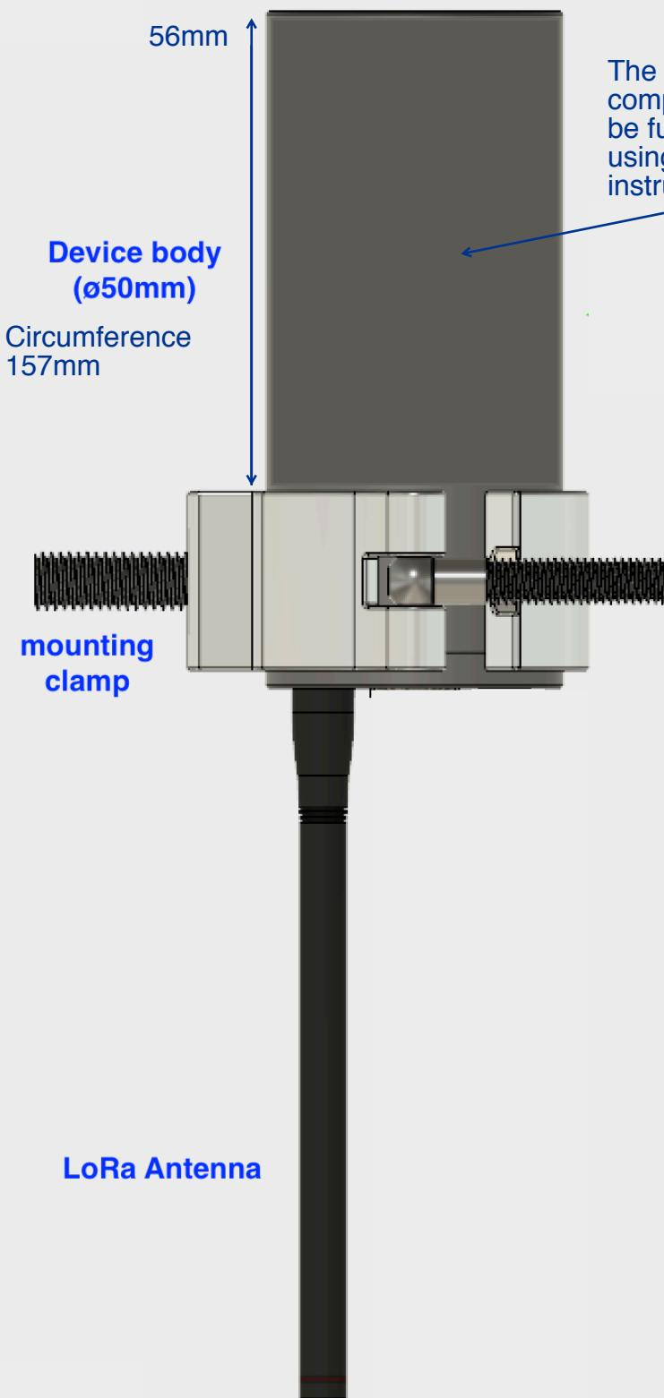
The compliance label will wrap around the complete circumference of the cylinder. It will be fully visible when the device is installed using the supplied mounting clamp, as per the instructions in the User Manual.
