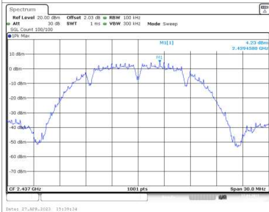
Tx. Spurious NVNT b 2437MHz Ant1 Emission
