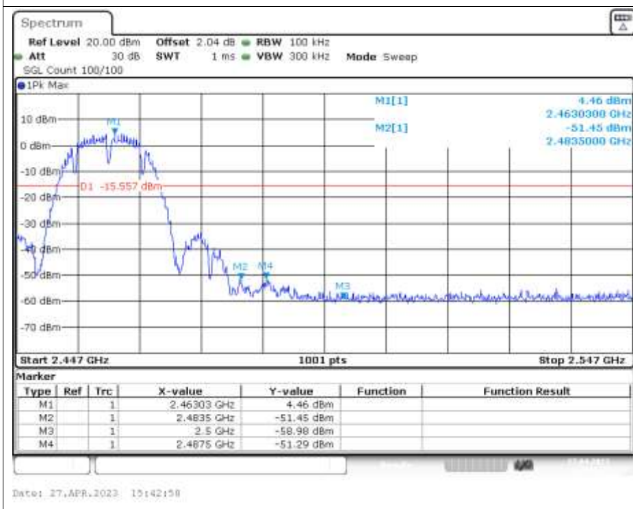
Band Edge NVNT b 2462MHz Ant1 Emission
