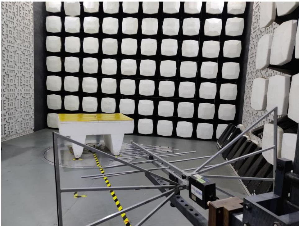
**1.3 Radiated Spurious Emissions Test Setup(Above 1GHz)**
