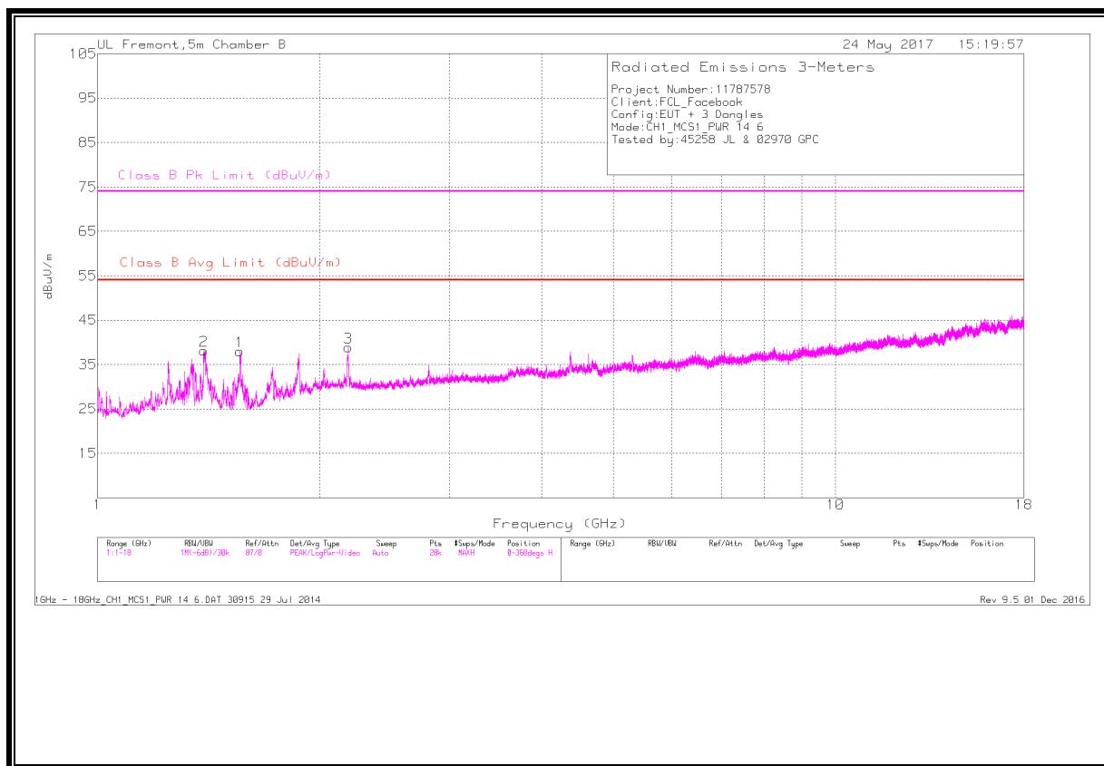
**CHANNEL 1 – TX SPURIOUS EMISSION 1-18 GHz (VERTICAL PLOT)**
