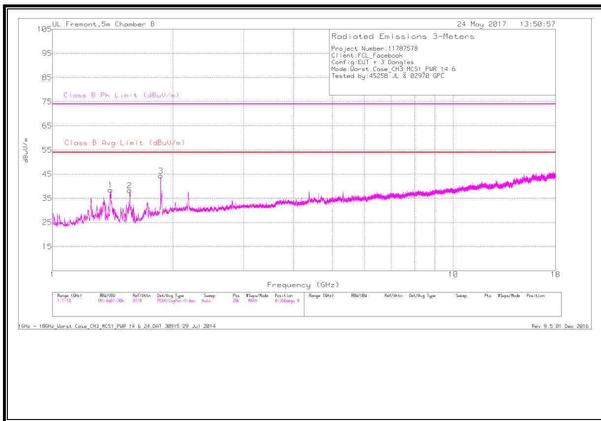
**CHANNEL 3 – TX SPURIOUS EMISSION 1 - 18 GHz (VERTICAL PLOT)**
