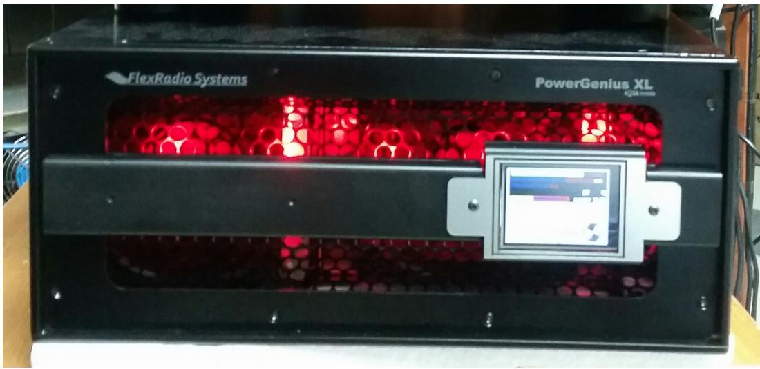
The red backlight indicates the amplifier is in **TX** mode.
