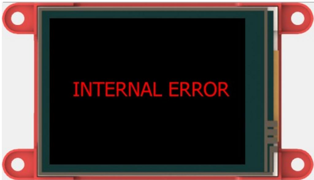
In case the display module loses communication with the main processor. Try rebooting the amplifier.
