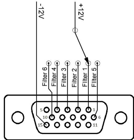
**BCD input** – Uses BCD signal (+12V) signal to select the proper filter. Pins are isolated with optocouplers.
