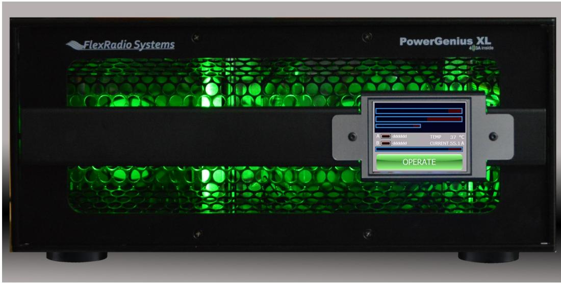
The green backlight indicates the amplifier is in **OPERATE** mode.
