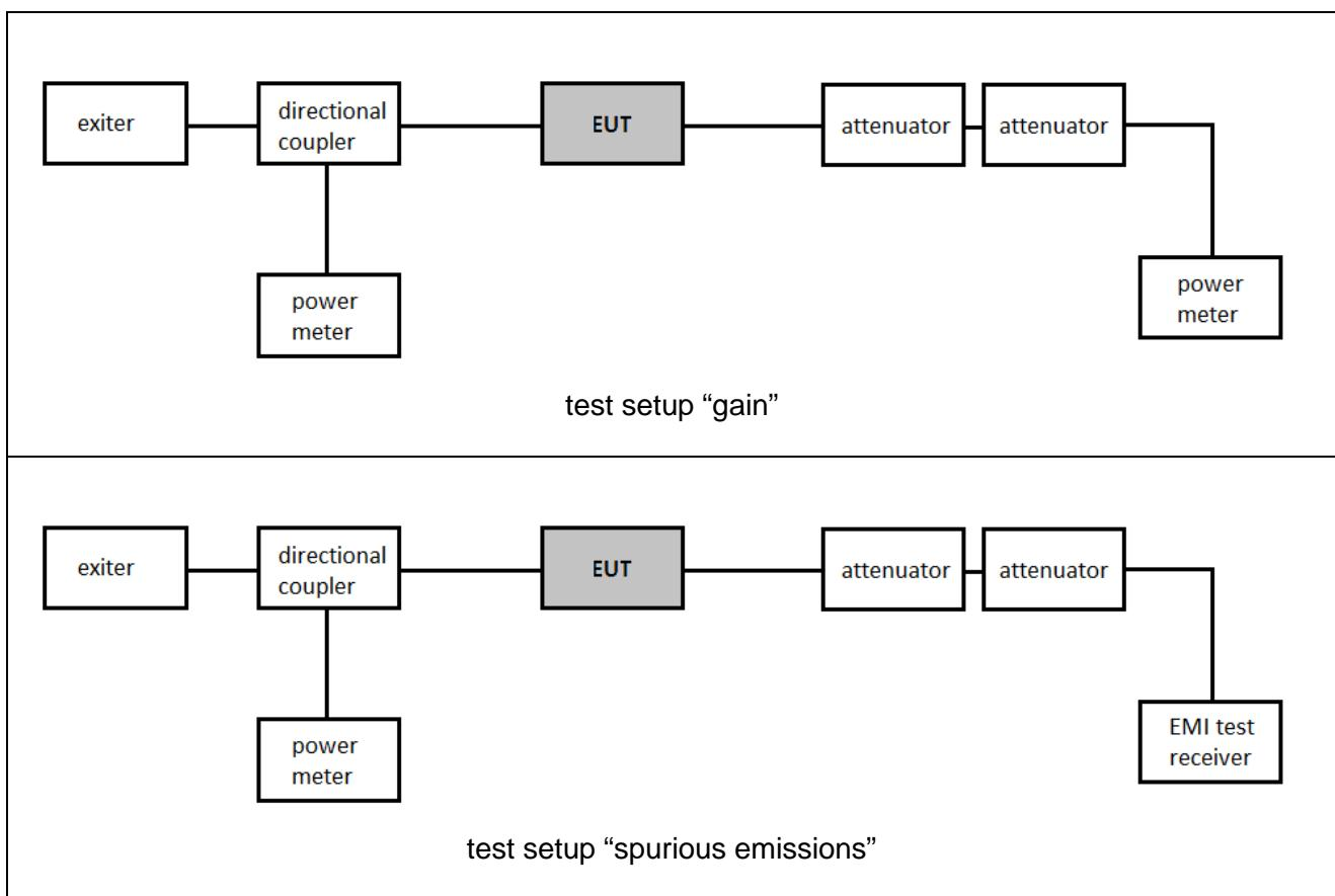
Test of SKY SAT d.o.o. Genius Power XL to 47 CFR §§ 15.107, 15.109, 97.307, 97.317
