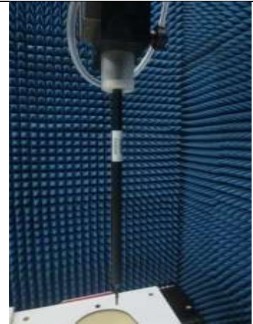
Fig. 8.2 Photo of E-Field Probe
