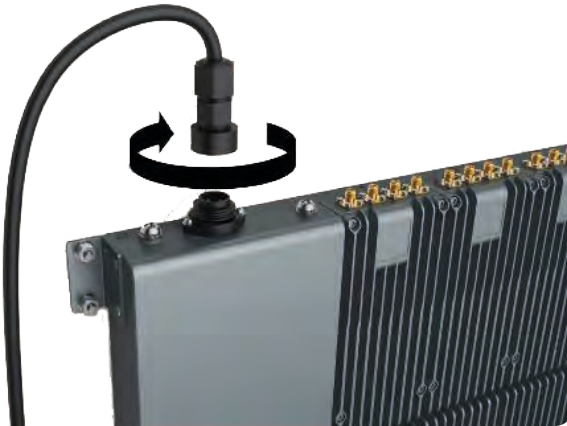
Fig. 17: Connect power cable at rear side
