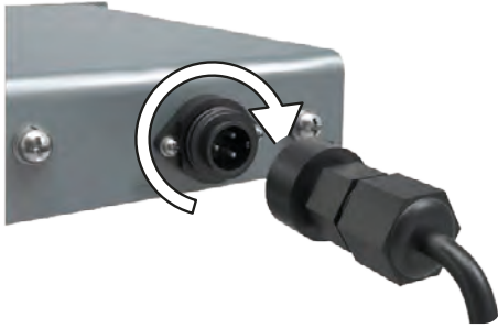
Fig. 12: Connect power cable at rear side
