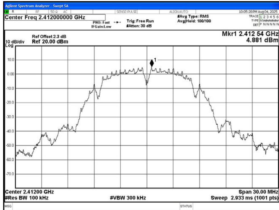
Band Edge NVNT b 2412MHz Ant1 Emission
