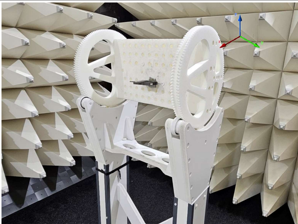
Test setup - Antenna position to the axis - Measuring antenna horizontal
