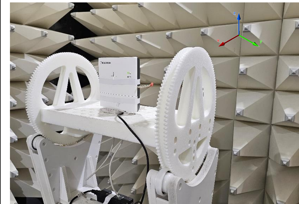
Test setup - Antenna position to the axis - Measuring antenna vertical
