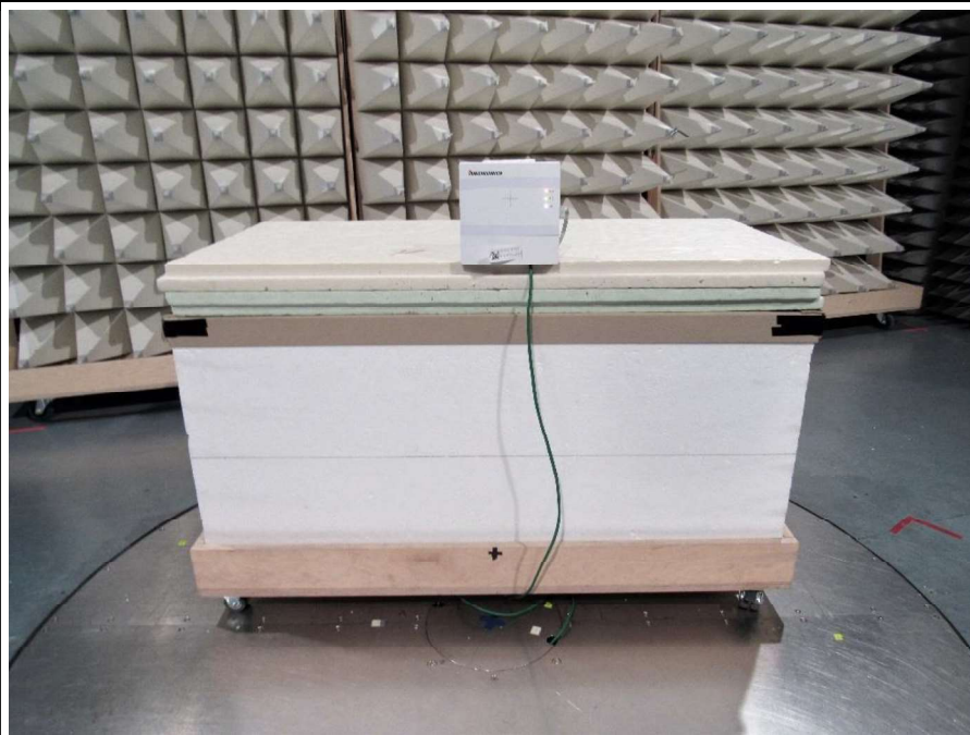
EUT setup below 1 GHz
