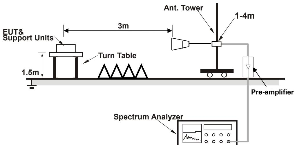
**For radiated test above 18GHz**
