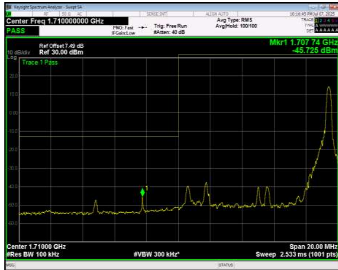
Band4 QPSK BW=10MHz Channel=20000 RB Size=50 Position=#0 Extended
