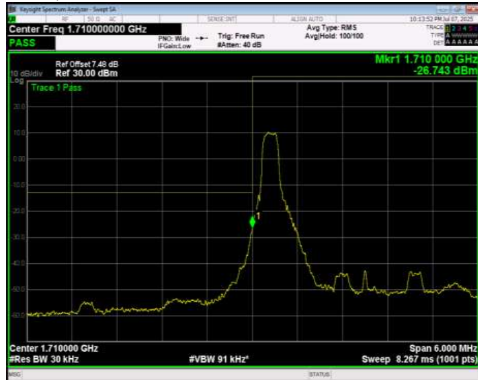
Band4 QPSK BW=3MHz Channel=19965 RB Size=1 Position=#Max Extended
