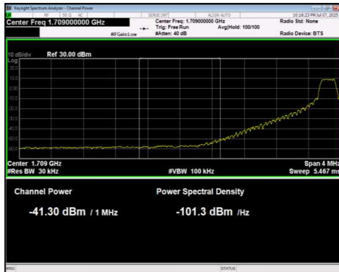
Band4 16QAM BW=15MHz Channel=20025 RB Size=1 Position=#0 Normal
