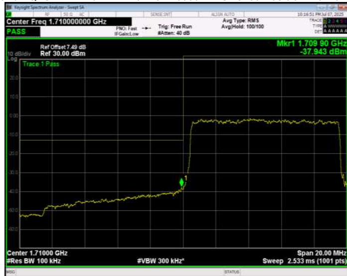
Band4 QPSK BW=10MHz Channel=20350 RB Size=1 Position=#0 Extended
