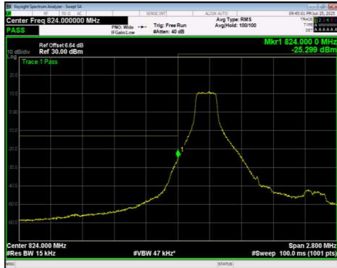
Band5 16QAM BW=1.4MHz Channel=20407 RB Size=1 Position=#Max Extended
