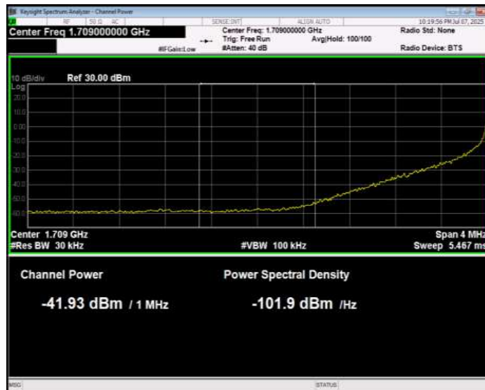
Band4 16QAM BW=20MHz Channel=20050 RB Size=1 Position=#0 Normal
