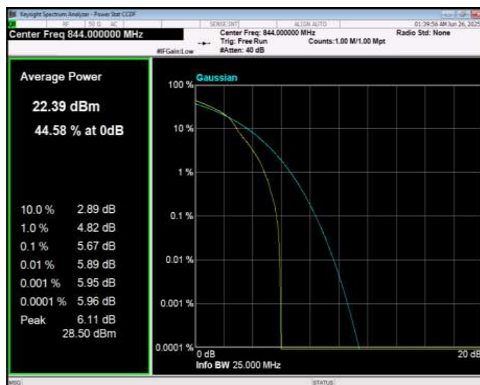
Band26(824-849) 16QAM BW=15MHz Channel=26865 RB Size=1 Position=#0
