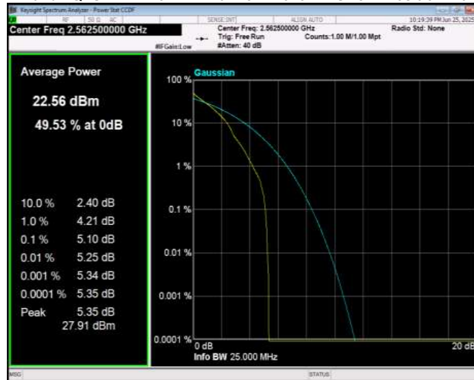
Band7 QPSK BW=20MHz Channel=20850 RB Size=1 Position=#0
