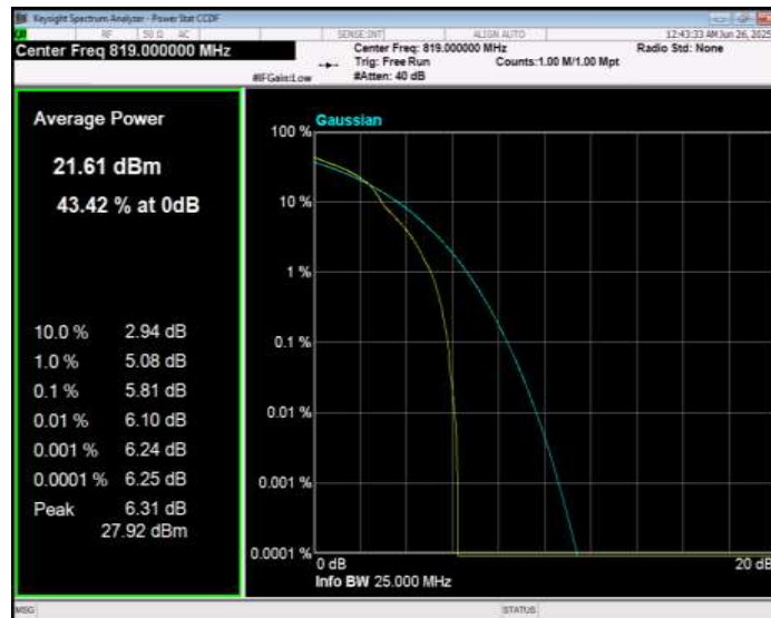
Band26(814-824) 16QAM BW=1.4MHz Channel=26783 RB Size=1 Position=#0
