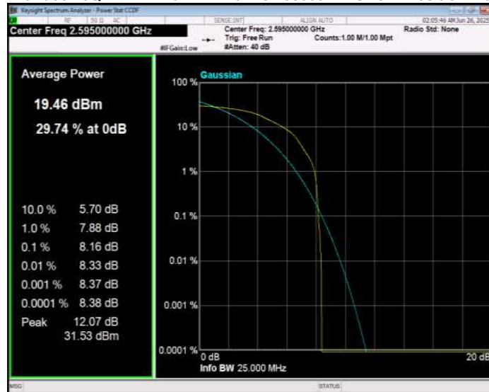
Band38 16QAM BW=10MHz Channel=38200 RB Size=1 Position=#0
