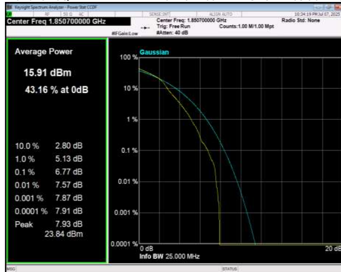
Band25 16QAM BW=1.4MHz Channel=26365 RB Size=1 Position=#0
