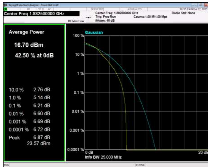
Band25 16QAM BW=5MHz Channel=26665 RB Size=1 Position=#0
