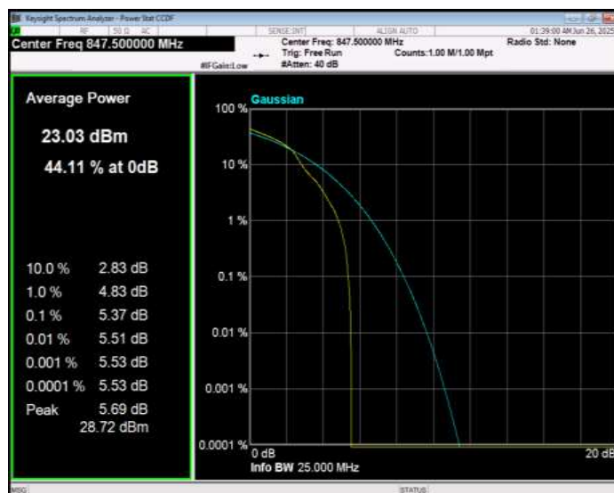
Band26(824-849) 16QAM BW=5MHz Channel=26815 RB Size=1 Position=#0
