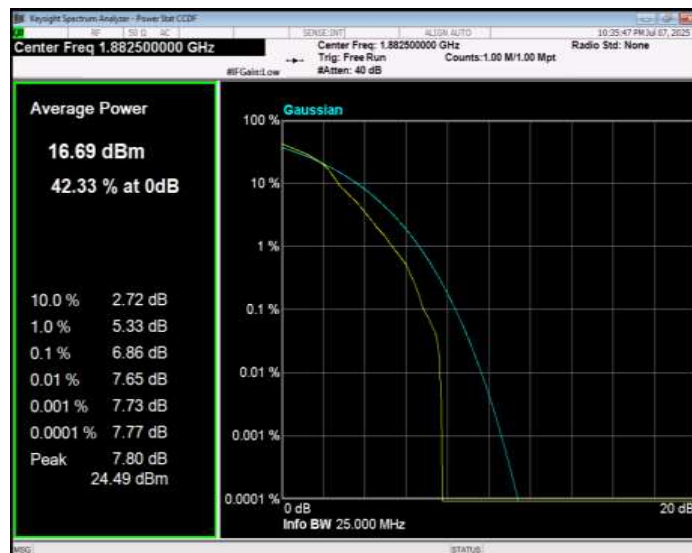
Band25 16QAM BW=10MHz Channel=26640 RB Size=1 Position=#0
