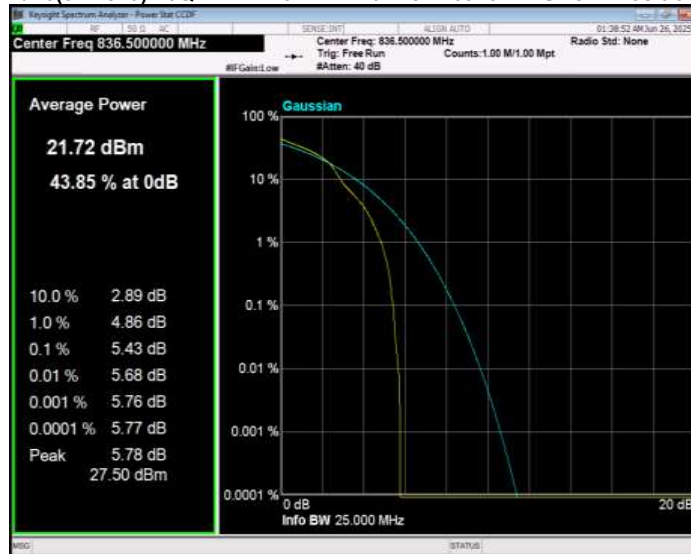
Band26(824-849) 16QAM BW=3MHz Channel=27025 RB Size=1 Position=#0
