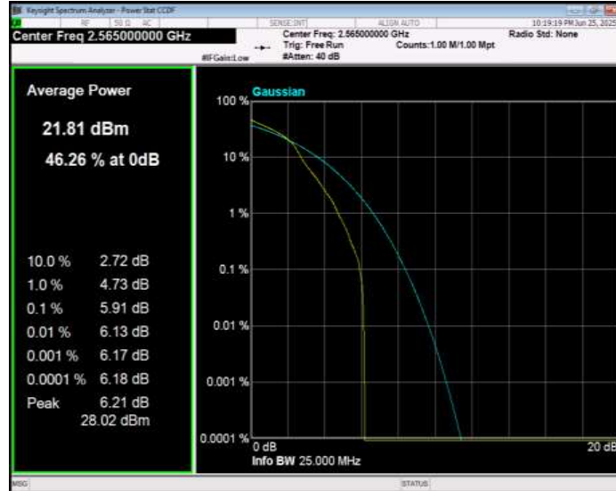
Band7 16QAM BW=15MHz Channel=20825 RB Size=1 Position=#0
