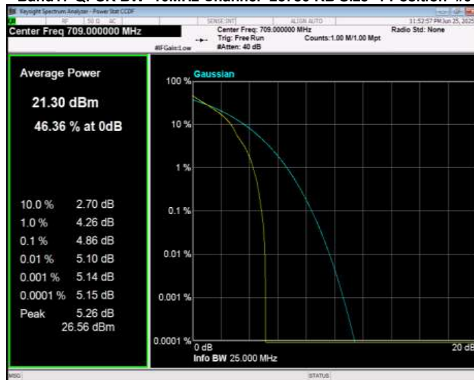
Band17 QPSK BW=10MHz Channel=23790 RB Size=1 Position=#0
