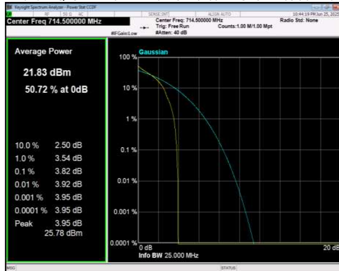
Band12 QPSK BW=5MHz Channel=23035 RB Size=1 Position=#0
