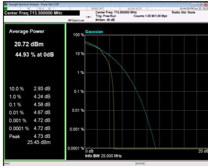
Band12 QPSK BW=1.4MHz Channel=23017 RB Size=1 Position=#0
