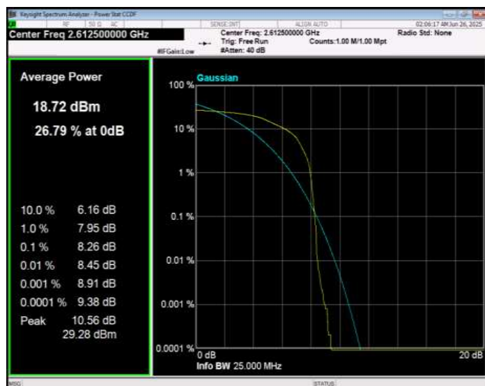
Band38 16QAM BW=20MHz Channel=37850 RB Size=1 Position=#0
