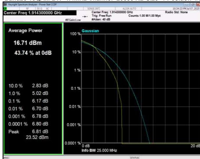
Band25 16QAM BW=10MHz Channel=26090 RB Size=1 Position=#0
