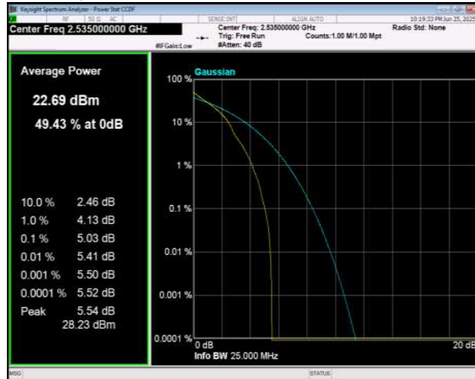
Band7 QPSK BW=15MHz Channel=21375 RB Size=1 Position=#0
