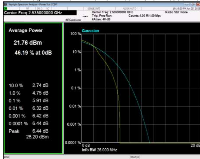
Band7 16QAM BW=15MHz Channel=21375 RB Size=1 Position=#0
