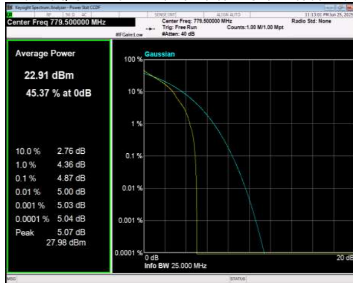
Band13 QPSK BW=5MHz Channel=23230 RB Size=1 Position=#0
