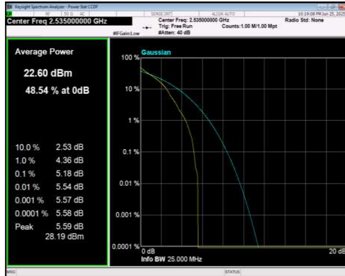
Band7 QPSK BW=10MHz Channel=21400 RB Size=1 Position=#0
