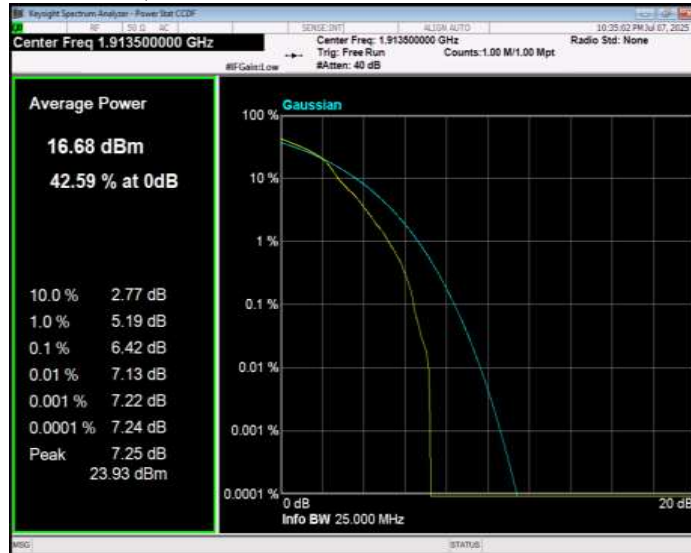
Band25 16QAM BW=5MHz Channel=26065 RB Size=1 Position=#0
