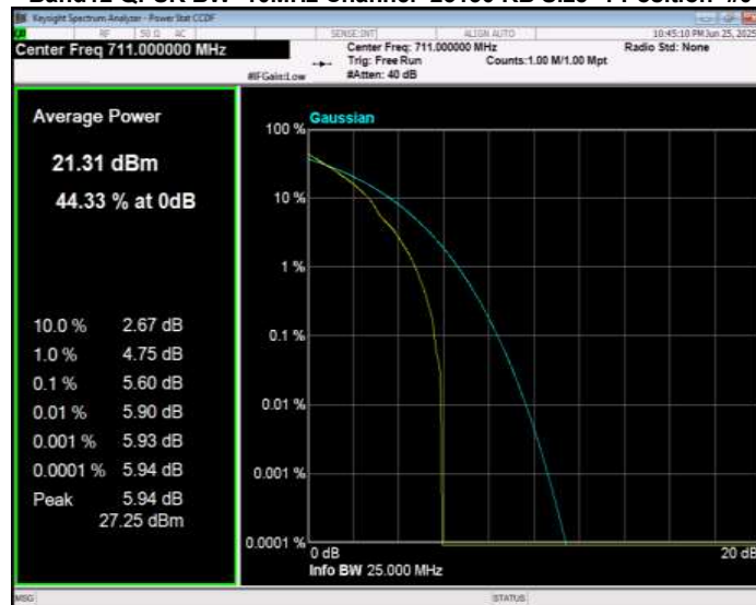
Band12 QPSK BW=3MHz Channel=23025 RB Size=1 Position=#0
