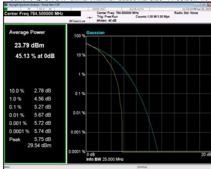
Band17 16QAM BW=10MHz Channel=23780 RB Size=1 Position=#0
