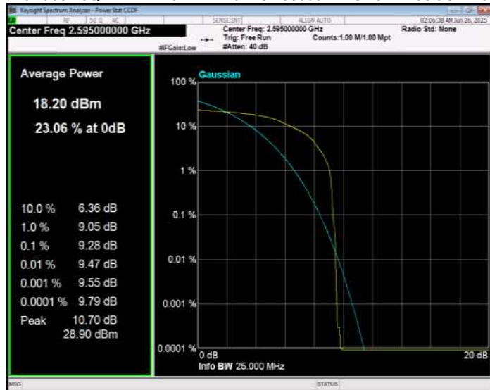
Band38 16QAM BW=20MHz Channel=38150 RB Size=1 Position=#0
