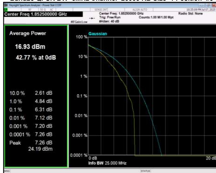
Band25 QPSK BW=5MHz Channel=26365 RB Size=1 Position=#0
