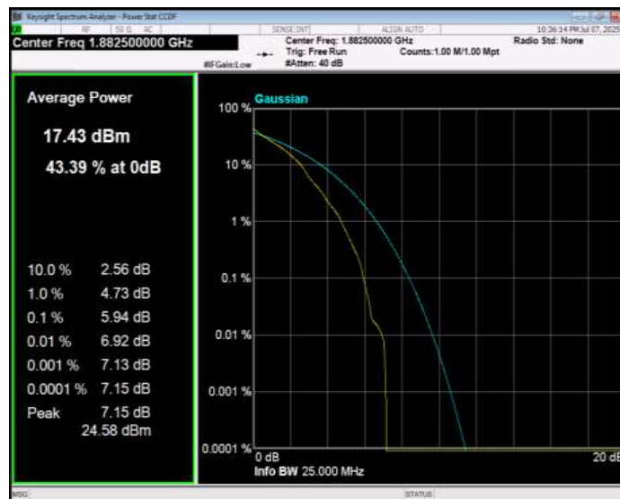
Band25 QPSK BW=15MHz Channel=26615 RB Size=1 Position=#0
