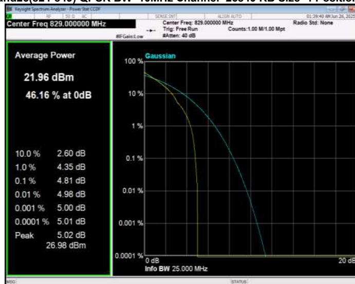
Band26(824-849) QPSK BW=10MHz Channel=26915 RB Size=1 Position=#0
