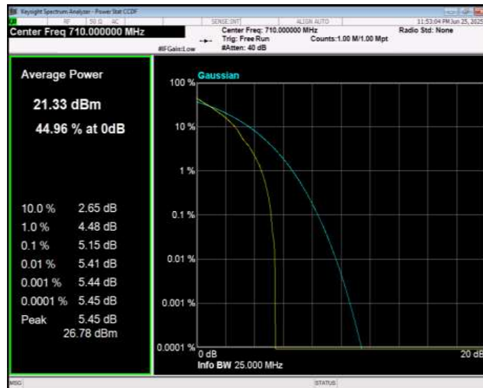
Band17 QPSK BW=10MHz Channel=23800 RB Size=1 Position=#0
