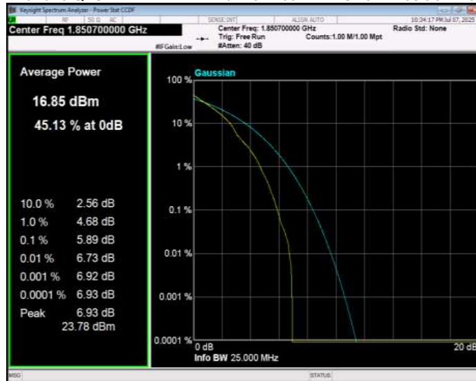
Band25 QPSK BW=1.4MHz Channel=26365 RB Size=1 Position=#0
