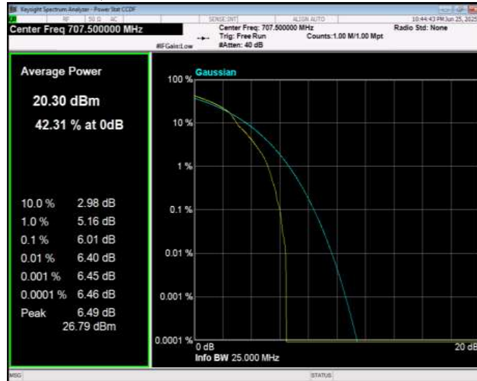
Band12 16QAM BW=5MHz Channel=23155 RB Size=1 Position=#0
