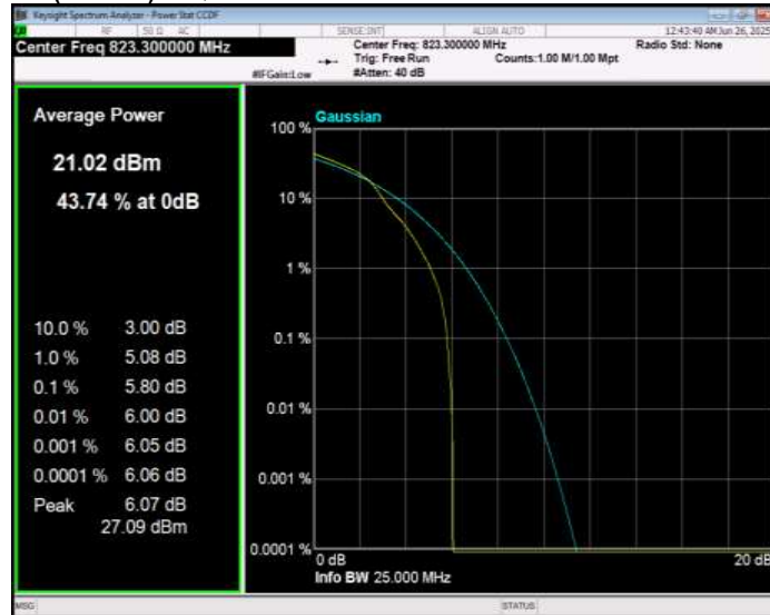
Band26(814-824) 16QAM BW=10MHz Channel=26740 RB Size=1 Position=#0
