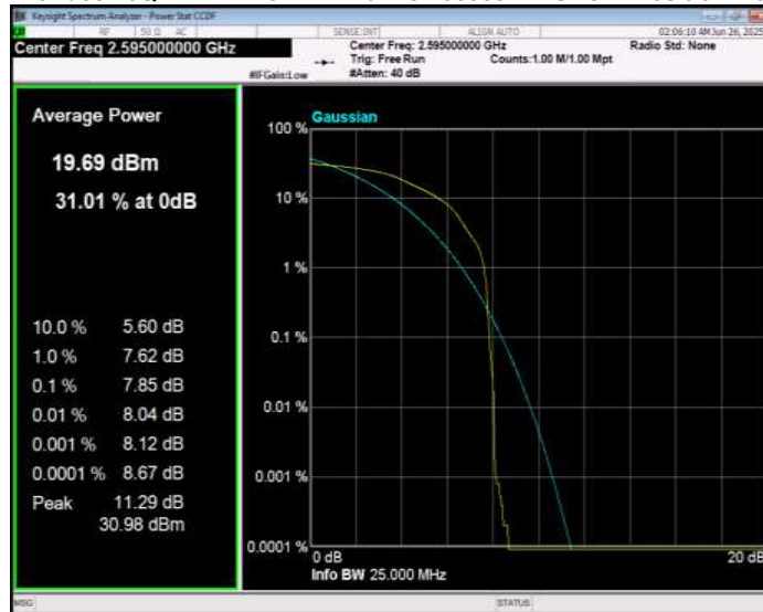
Band38 16QAM BW=15MHz Channel=38175 RB Size=1 Position=#0
