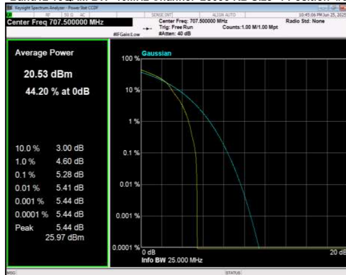
Band12 16QAM BW=10MHz Channel=23130 RB Size=1 Position=#0
