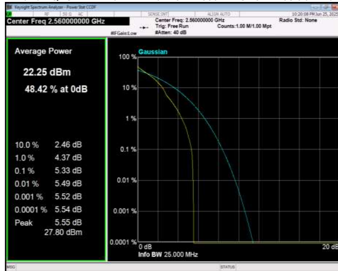
Band7 QPSK BW=5MHz Channel=20775 RB Size=1 Position=#0
