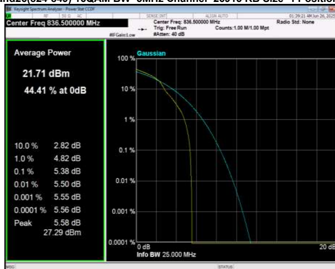
Band26(824-849) 16QAM BW=5MHz Channel=27015 RB Size=1 Position=#0
