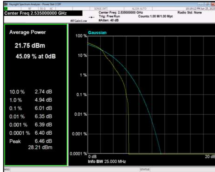
Band7 16QAM BW=10MHz Channel=21400 RB Size=1 Position=#0
