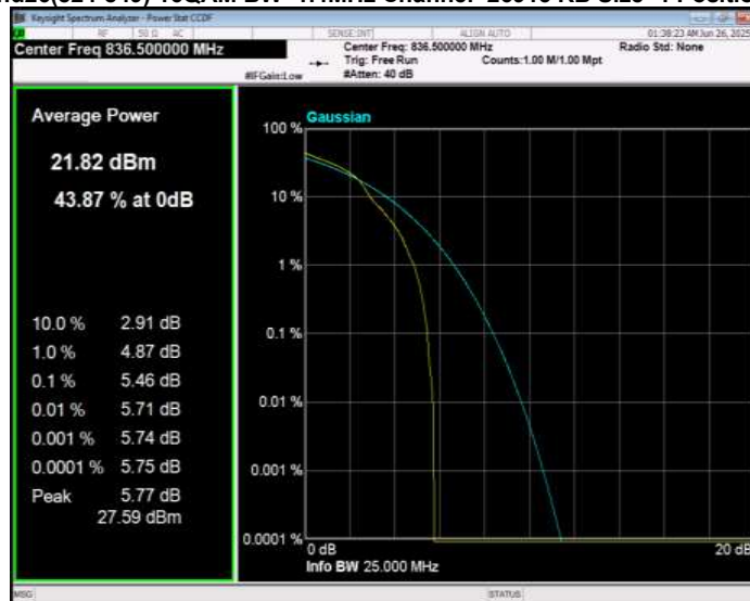
Band26(824-849) 16QAM BW=1.4MHz Channel=27033 RB Size=1 Position=#0
