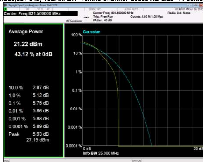
Band26(824-849) 16QAM BW=15MHz Channel=26915 RB Size=1 Position=#0
