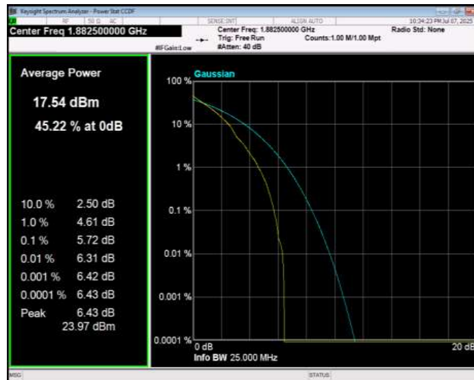
Band25 QPSK BW=1.4MHz Channel=26683 RB Size=1 Position=#0
