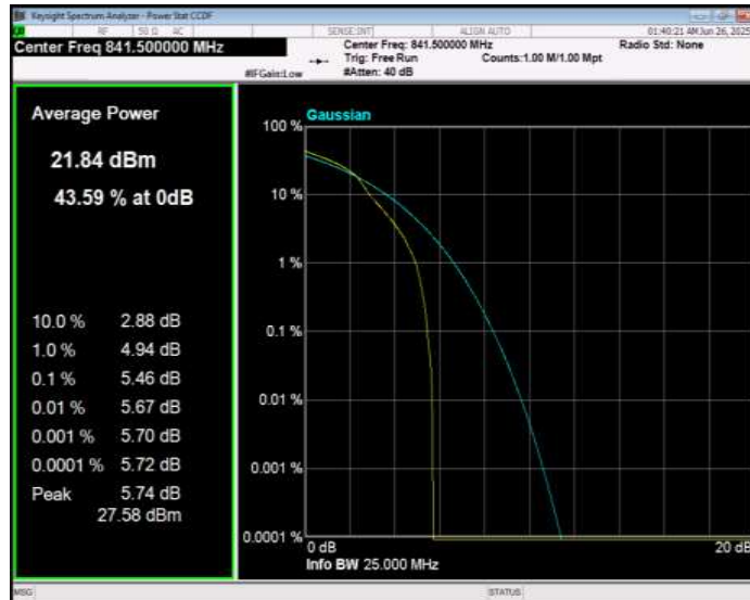
Band26(824-849) 16QAM BW=3MHz Channel=26805 RB Size=1 Position=#0
