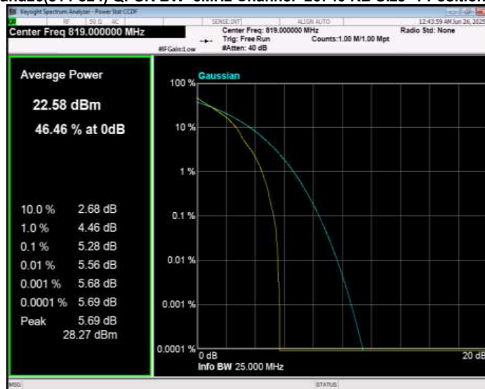
Band26(814-824) QPSK BW=3MHz Channel=26775 RB Size=1 Position=#0
