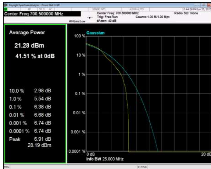
Band12 16QAM BW=3MHz Channel=23095 RB Size=1 Position=#0
