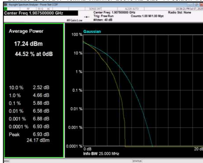
Band25 QPSK BW=20MHz Channel=26140 RB Size=1 Position=#0
