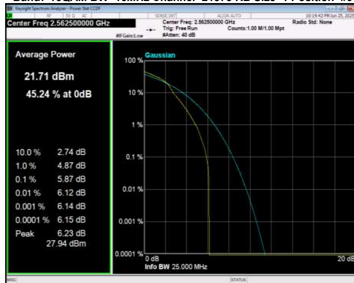
Band7 16QAM BW=20MHz Channel=20850 RB Size=1 Position=#0
