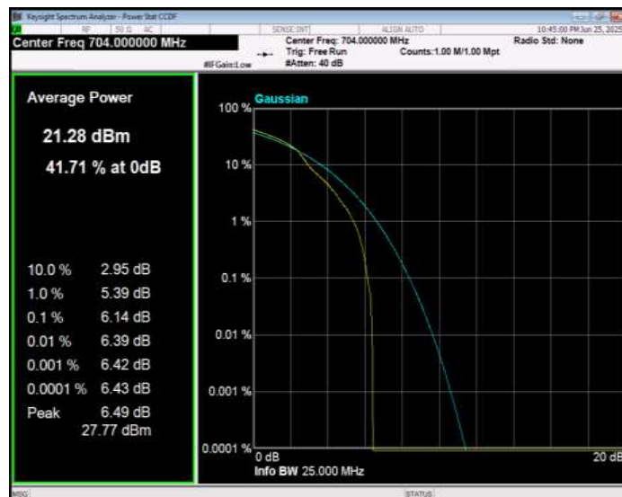
Band12 16QAM BW=10MHz Channel=23095 RB Size=1 Position=#0
