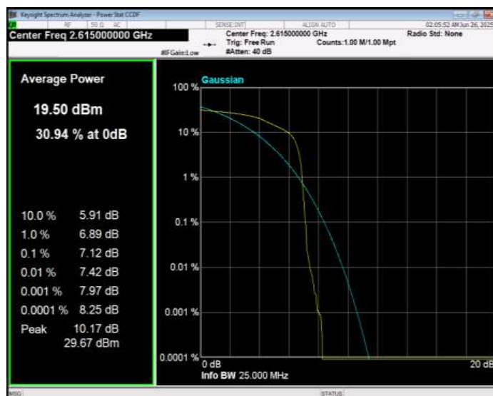
Band38 16QAM BW=15MHz Channel=37825 RB Size=1 Position=#0
