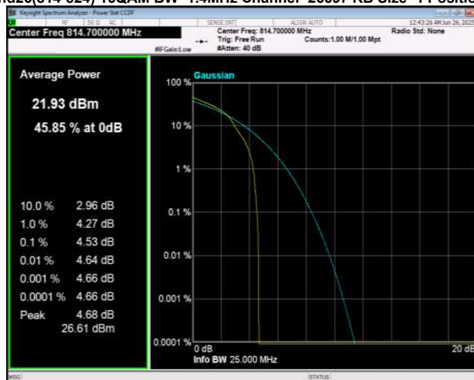
Band26(814-824) 16QAM BW=1.4MHz Channel=26740 RB Size=1 Position=#0
