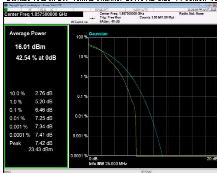
Band25 16QAM BW=15MHz Channel=26365 RB Size=1 Position=#0
