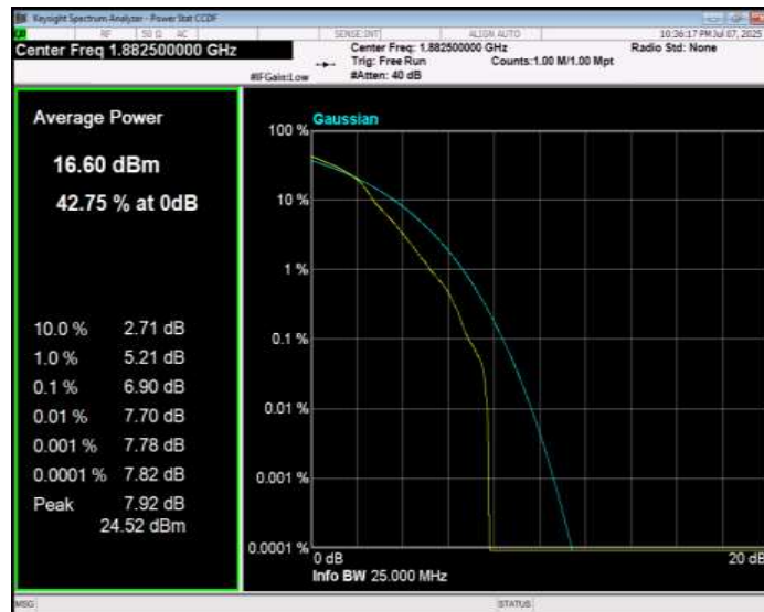
Band25 16QAM BW=15MHz Channel=26615 RB Size=1 Position=#0
