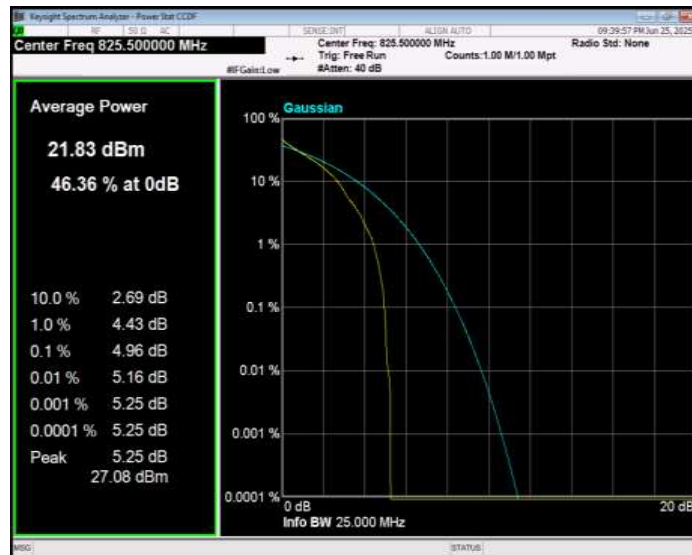
Band5 QPSK BW=3MHz Channel=20525 RB Size=1 Position=#0
