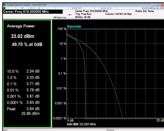
Band26(814-824) QPSK BW=3MHz Channel=26705 RB Size=1 Position=#0
