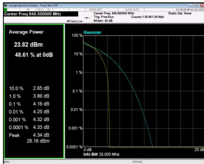
Band38 16QAM BW=10MHz Channel=37800 RB Size=1 Position=#0
