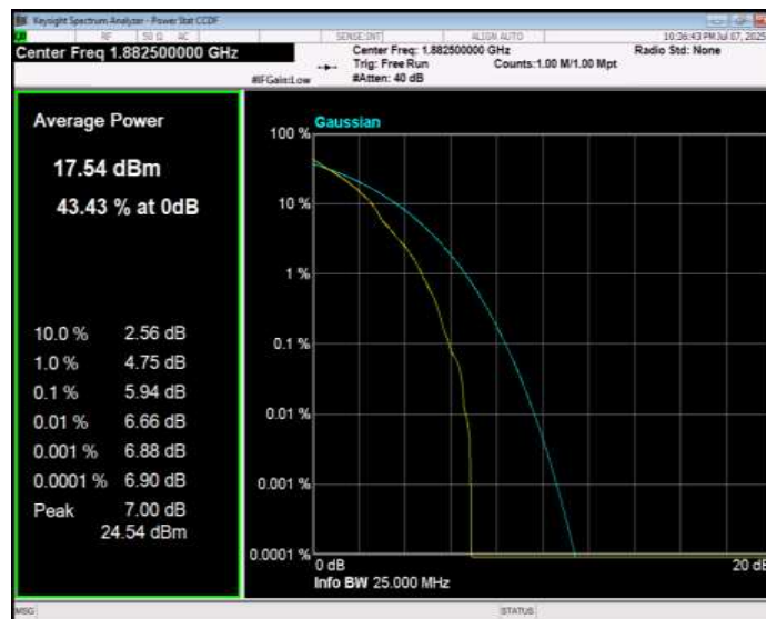
Band25 QPSK BW=20MHz Channel=26590 RB Size=1 Position=#0
