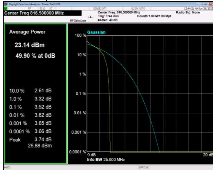
Band26(814-824) QPSK BW=5MHz Channel=26740 RB Size=1 Position=#0
