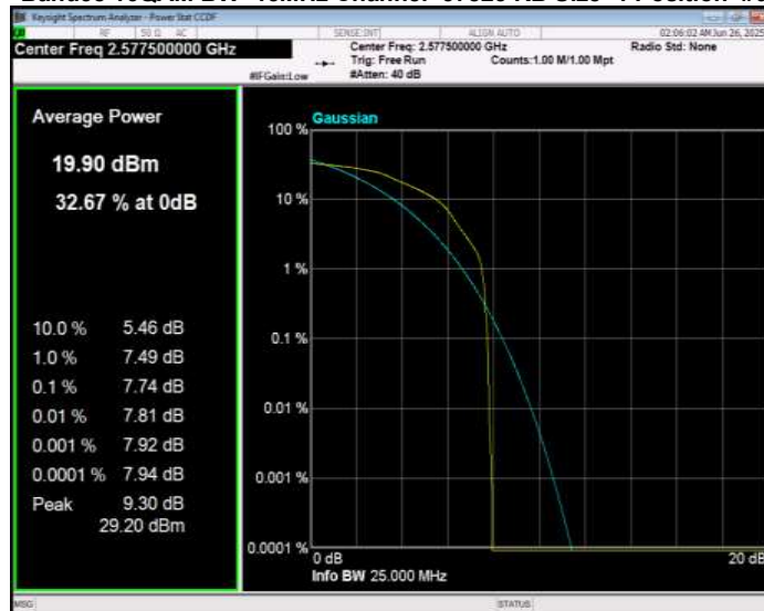
Band38 16QAM BW=15MHz Channel=38000 RB Size=1 Position=#0
