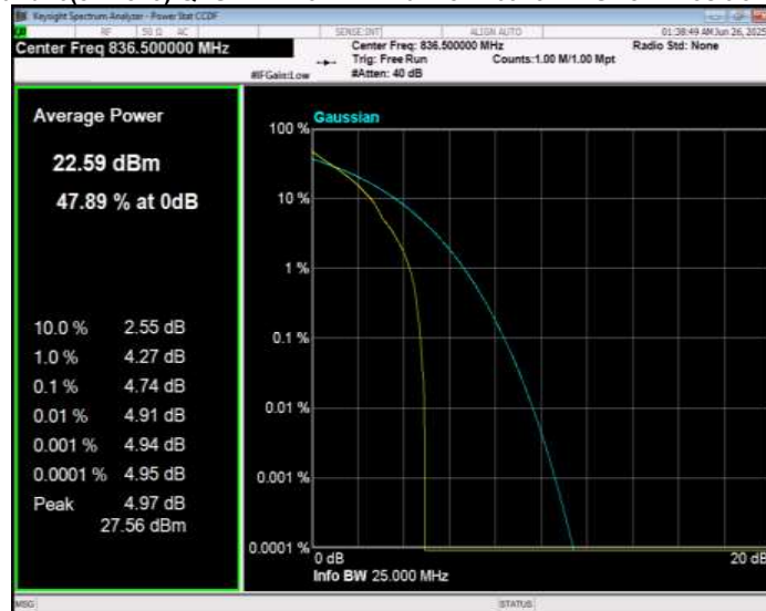
Band26(824-849) QPSK BW=3MHz Channel=27025 RB Size=1 Position=#0
