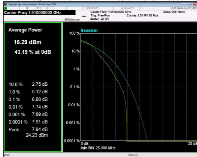
Band25 16QAM BW=15MHz Channel=26115 RB Size=1 Position=#0
