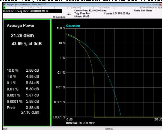
Band26(814-824) 16QAM BW=5MHz Channel=26715 RB Size=1 Position=#0
