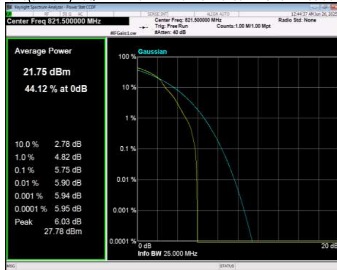
Band26(814-824) QPSK BW=1.4MHz Channel=26697 RB Size=1 Position=#0
