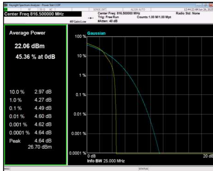
Band26(814-824) 16QAM BW=5MHz Channel=26740 RB Size=1 Position=#0
