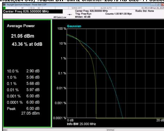
Band26(824-849) 16QAM BW=5MHz Channel=26915 RB Size=1 Position=#0
