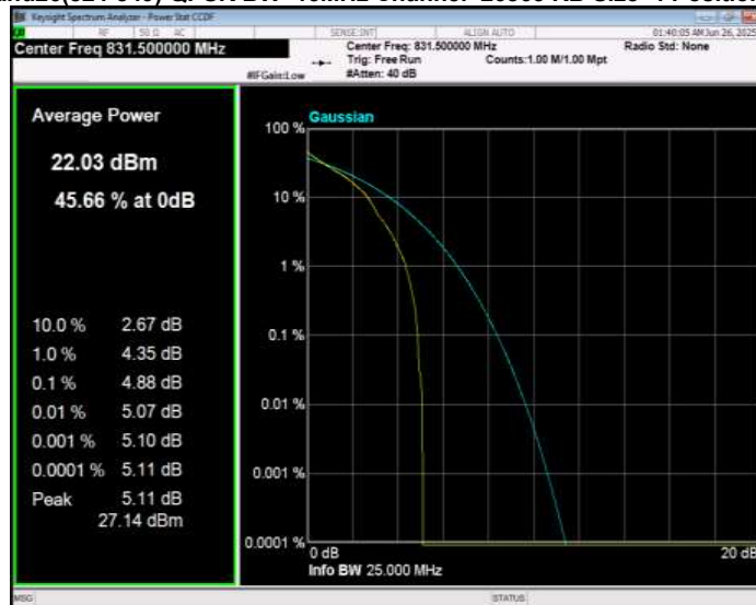
Band26(824-849) QPSK BW=15MHz Channel=26915 RB Size=1 Position=#0
