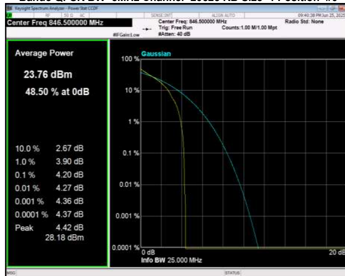
Band7 16QAM BW=10MHz Channel=20800 RB Size=1 Position=#0
