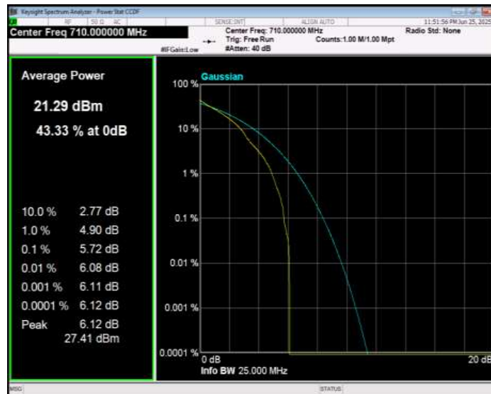
Band17 QPSK BW=5MHz Channel=23825 RB Size=1 Position=#0
