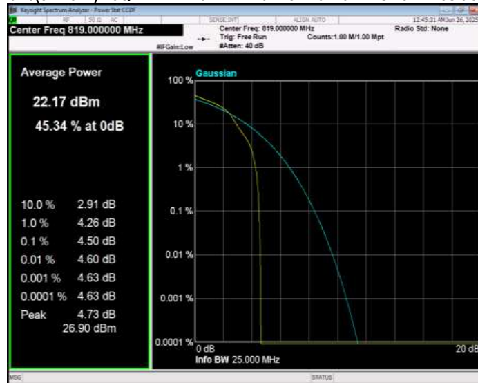
Band26(814-824) 16QAM BW=3MHz Channel=26705 RB Size=1 Position=#0
