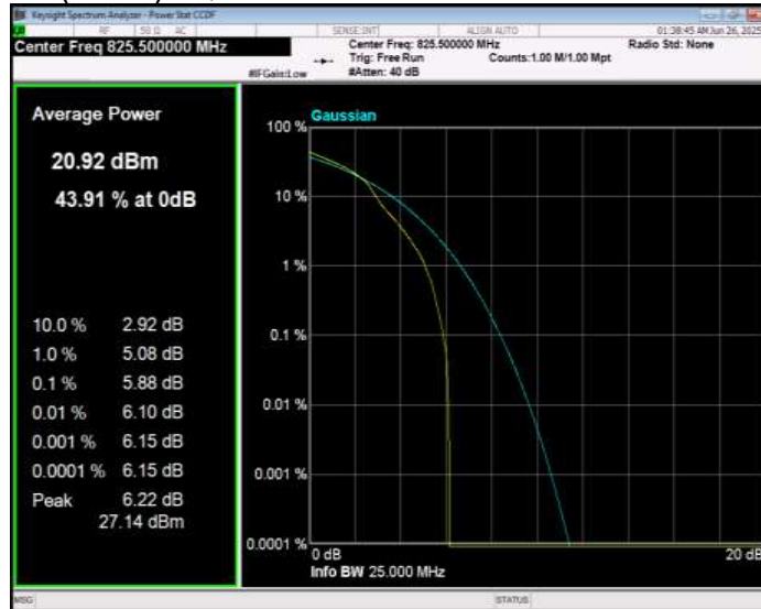
Band26(824-849) 16QAM BW=3MHz Channel=26915 RB Size=1 Position=#0
