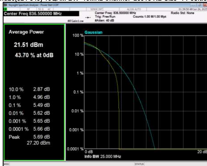
Band26(824-849) 16QAM BW=10MHz Channel=26990 RB Size=1 Position=#0
