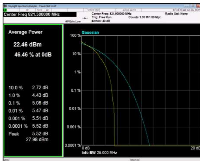
Band26(824-849) 16QAM BW=1.4MHz Channel=26797 RB Size=1 Position=#0
