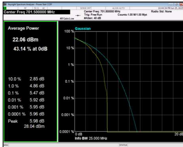
Band12 QPSK BW=5MHz Channel=23095 RB Size=1 Position=#0
