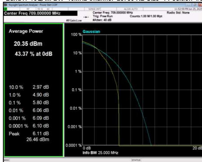
Band17 16QAM BW=10MHz Channel=23790 RB Size=1 Position=#0
