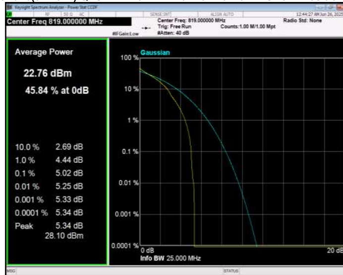
Band26(814-824) QPSK BW=5MHz Channel=26765 RB Size=1 Position=#0
