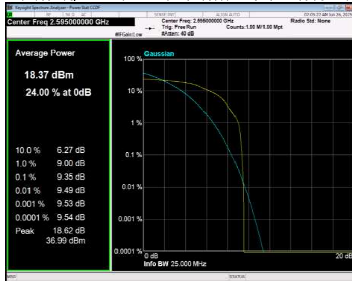
Band38 16QAM BW=5MHz Channel=38225 RB Size=1 Position=#0
