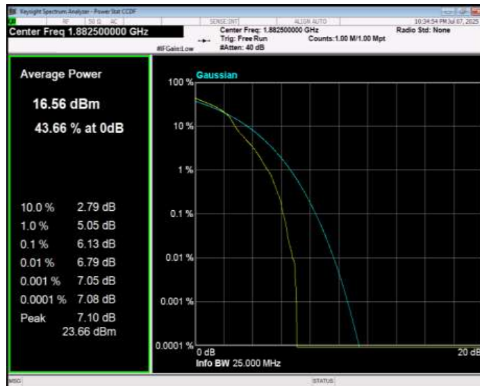
Band25 16QAM BW=3MHz Channel=26675 RB Size=1 Position=#0
