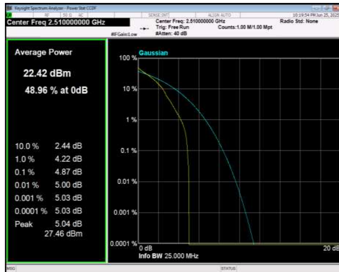
Band7 QPSK BW=20MHz Channel=21100 RB Size=1 Position=#0
