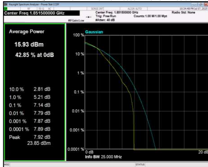
Band25 16QAM BW=3MHz Channel=26365 RB Size=1 Position=#0
