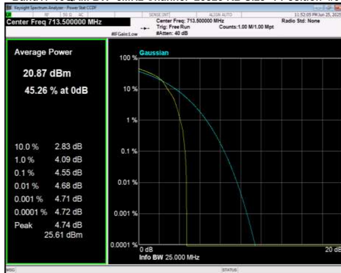
Band17 QPSK BW=10MHz Channel=23780 RB Size=1 Position=#0
