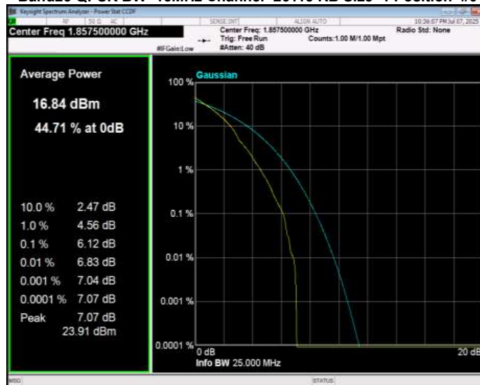
Band25 QPSK BW=15MHz Channel=26365 RB Size=1 Position=#0
