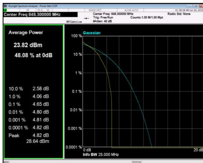
Band26(824-849) QPSK BW=10MHz Channel=26840 RB Size=1 Position=#0
