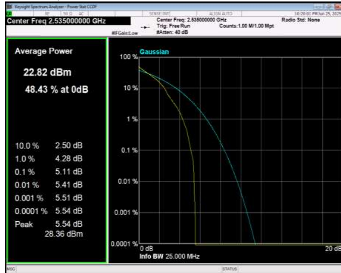
Band7 QPSK BW=20MHz Channel=21350 RB Size=1 Position=#0
