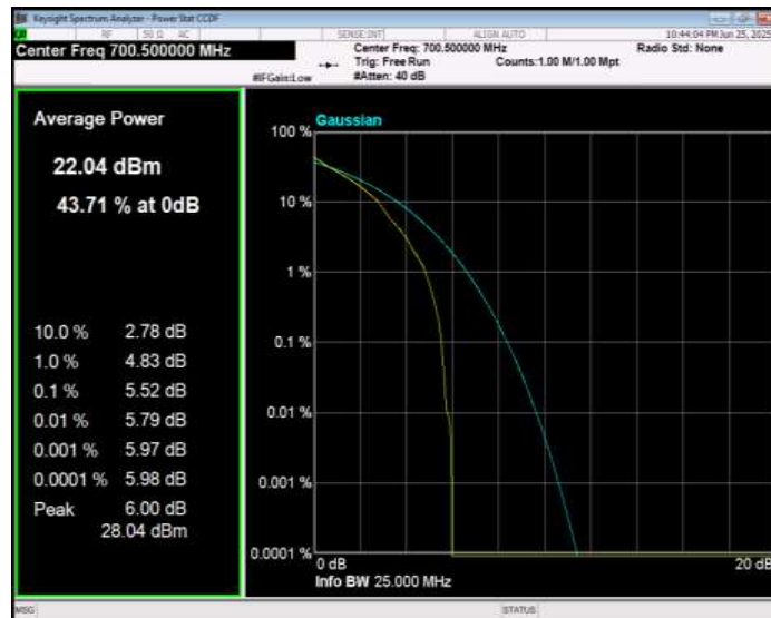
Band12 QPSK BW=3MHz Channel=23095 RB Size=1 Position=#0
