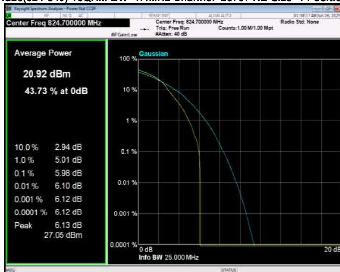
Band26(824-849) 16QAM BW=1.4MHz Channel=26915 RB Size=1 Position=#0
