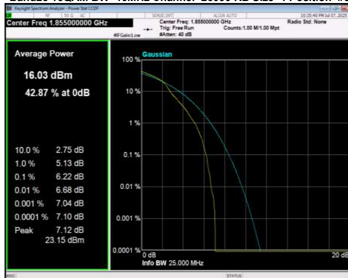
Band25 16QAM BW=10MHz Channel=26365 RB Size=1 Position=#0
