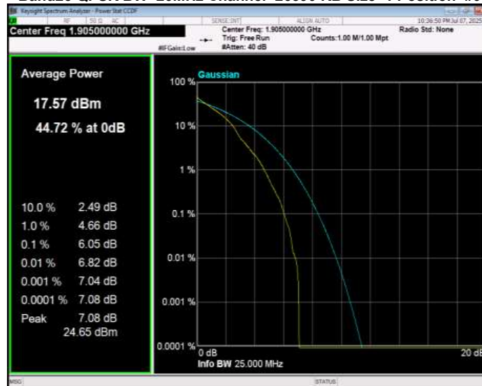
Band25 QPSK BW=3MHz Channel=26055 RB Size=1 Position=#0
