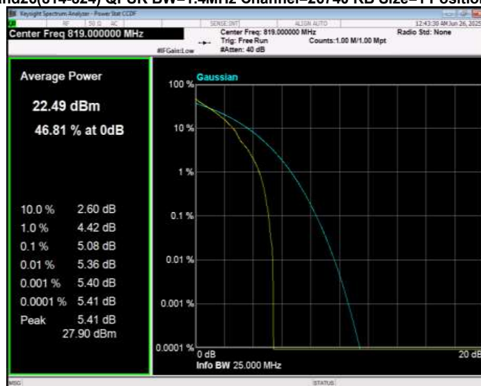
Band26(814-824) QPSK BW=1.4MHz Channel=26783 RB Size=1 Position=#0
