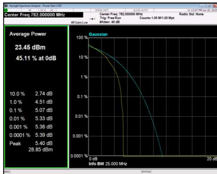
Band13 QPSK BW=5MHz Channel=23255 RB Size=1 Position=#0
