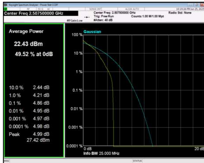
Band7 QPSK BW=15MHz Channel=21100 RB Size=1 Position=#0
