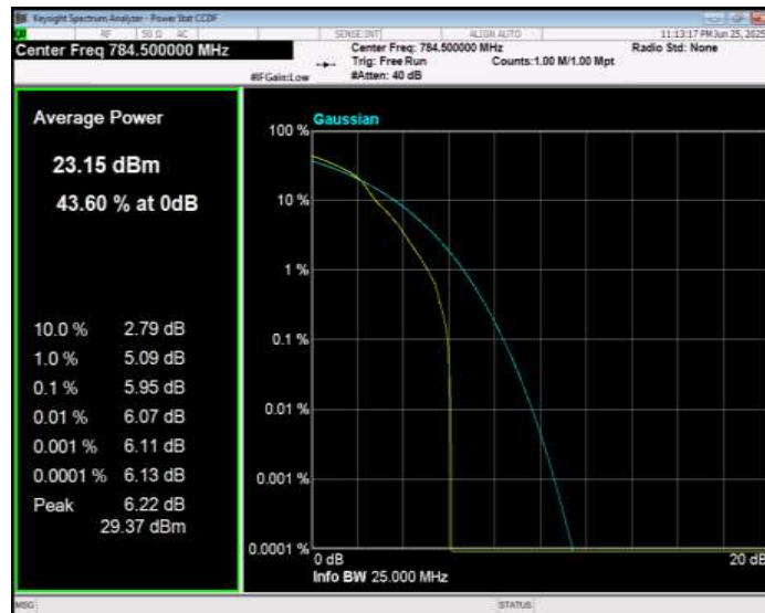
Band13 QPSK BW=10MHz Channel=23230 RB Size=1 Position=#0
