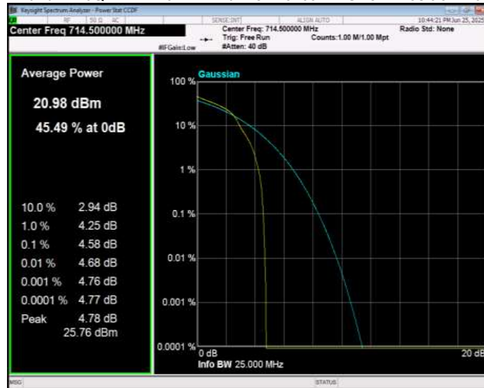
Band12 16QAM BW=5MHz Channel=23035 RB Size=1 Position=#0
