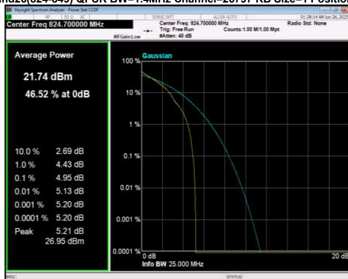
Band26(824-849) QPSK BW=1.4MHz Channel=26915 RB Size=1 Position=#0
