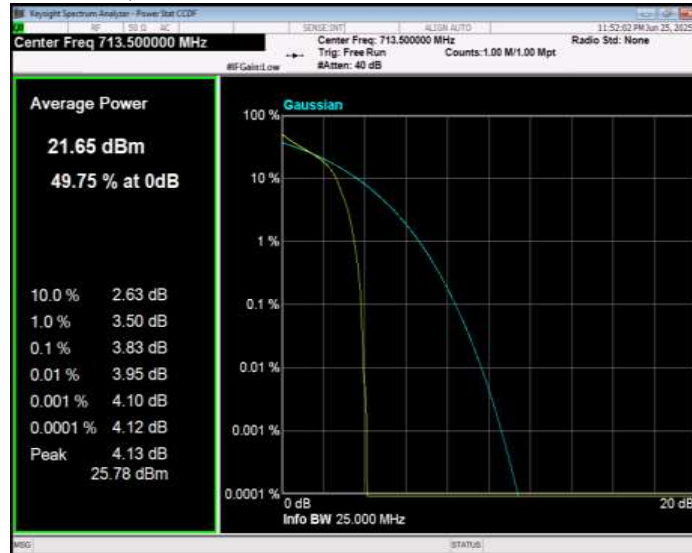
Band25 16QAM BW=1.4MHz Channel=26047 RB Size=1 Position=#0
