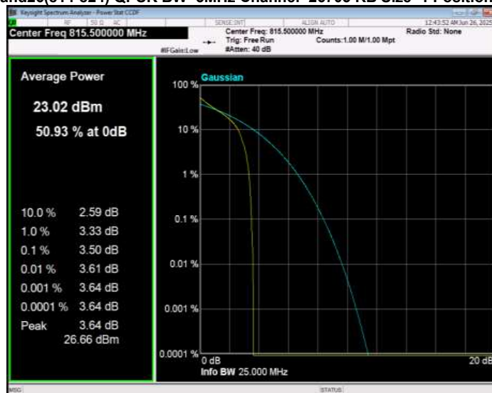
Band26(814-824) QPSK BW=3MHz Channel=26740 RB Size=1 Position=#0
