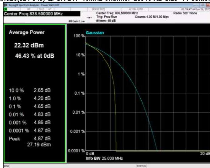
Band26(824-849) QPSK BW=10MHz Channel=26990 RB Size=1 Position=#0
