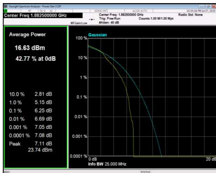
Band25 16QAM BW=1.4MHz Channel=26683 RB Size=1 Position=#0
