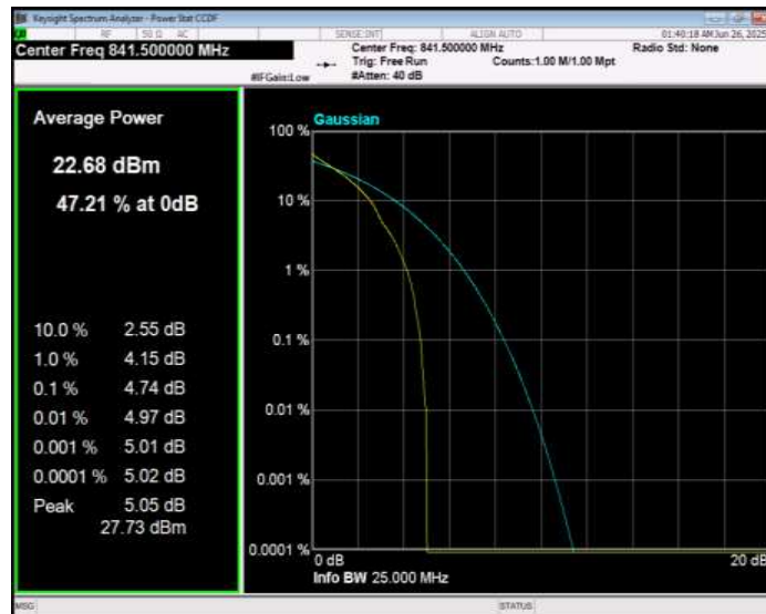
Band26(824-849) QPSK BW=3MHz Channel=26805 RB Size=1 Position=#0
