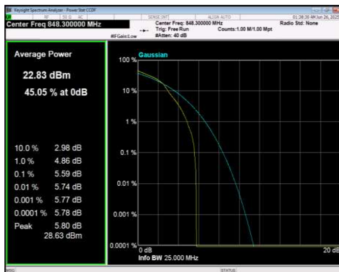
Band26(824-849) 16QAM BW=10MHz Channel=26840 RB Size=1 Position=#0
