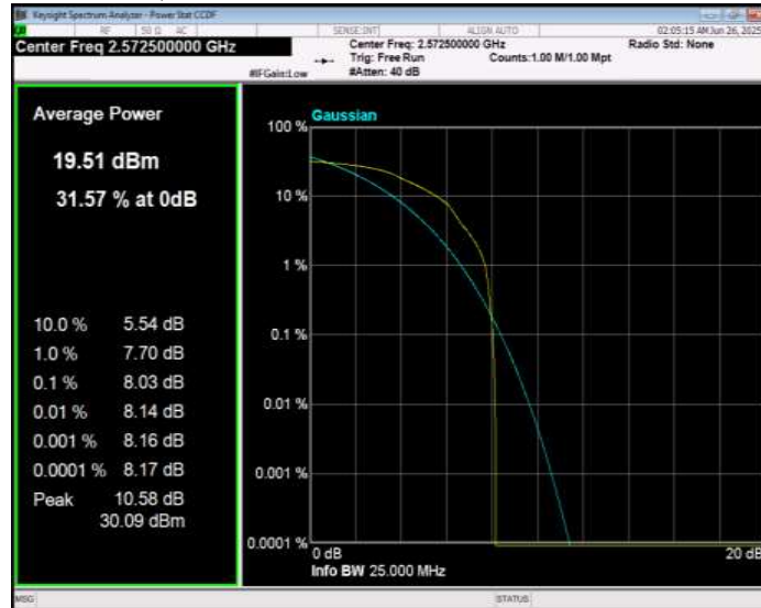
Band38 16QAM BW=5MHz Channel=38000 RB Size=1 Position=#0
