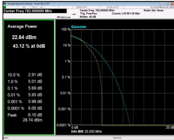
Band13 16QAM BW=5MHz Channel=23255 RB Size=1 Position=#0
