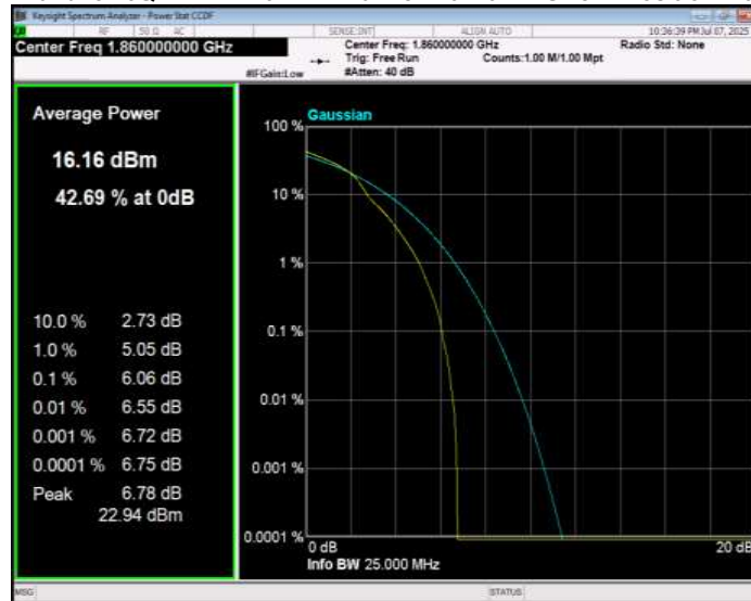
Band25 16QAM BW=20MHz Channel=26365 RB Size=1 Position=#0
