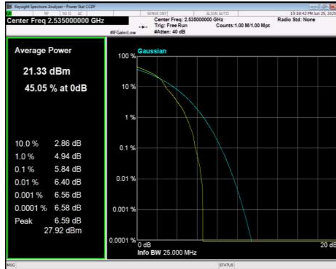
Band7 16QAM BW=5MHz Channel=21425 RB Size=1 Position=#0
