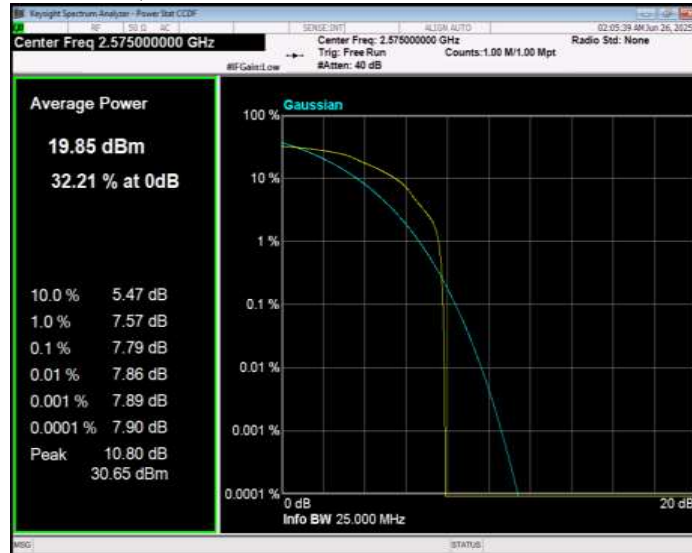
Band38 16QAM BW=10MHz Channel=38000 RB Size=1 Position=#0
