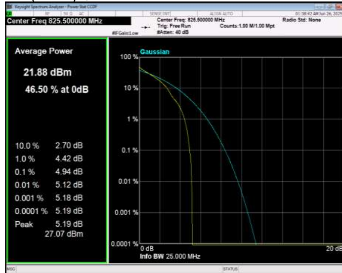
Band26(824-849) QPSK BW=3MHz Channel=26915 RB Size=1 Position=#0
