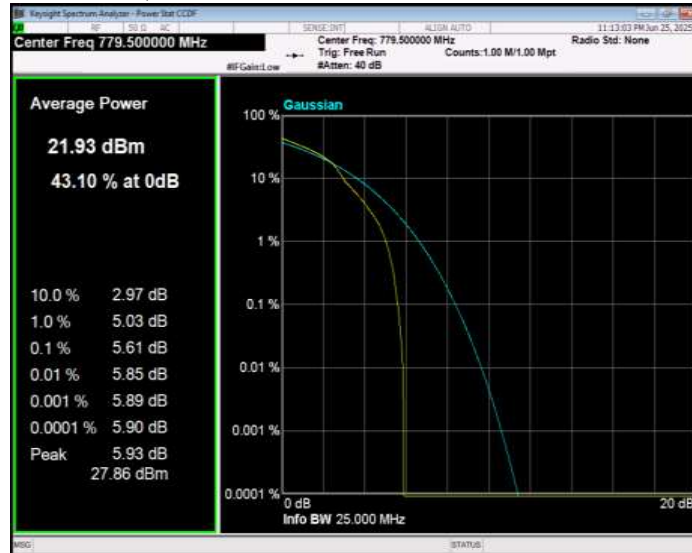
Band13 16QAM BW=5MHz Channel=23230 RB Size=1 Position=#0
