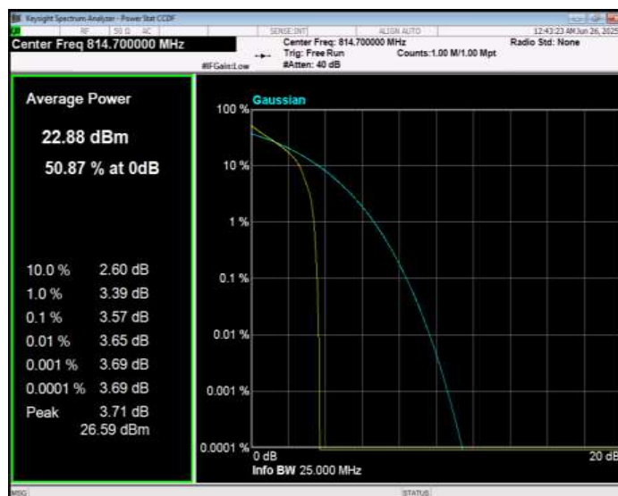
Band26(814-824) QPSK BW=1.4MHz Channel=26740 RB Size=1 Position=#0
