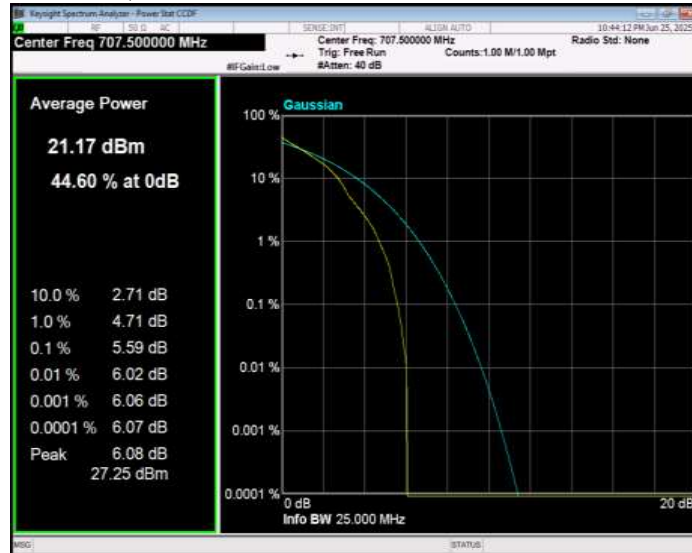
Band12 QPSK BW=3MHz Channel=23165 RB Size=1 Position=#0
