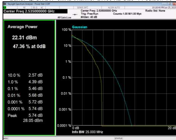
Band7 QPSK BW=5MHz Channel=21425 RB Size=1 Position=#0
