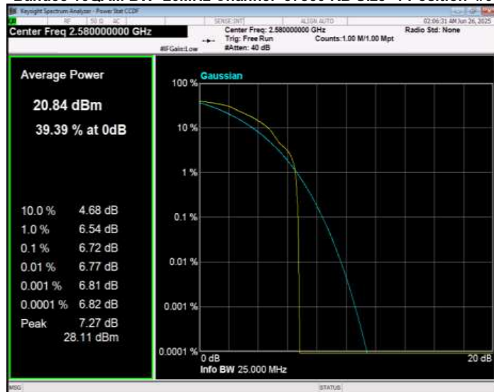
Band38 16QAM BW=20MHz Channel=38000 RB Size=1 Position=#0
