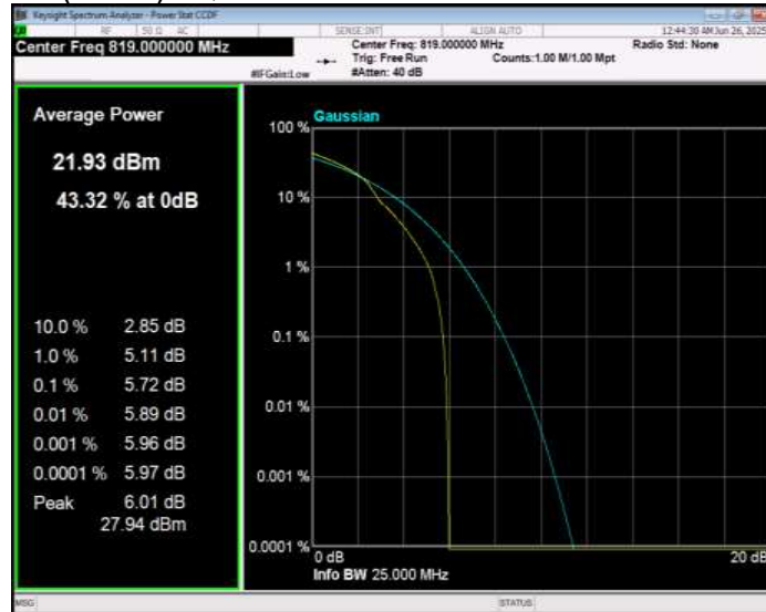
Band26(814-824) 16QAM BW=5MHz Channel=26765 RB Size=1 Position=#0
