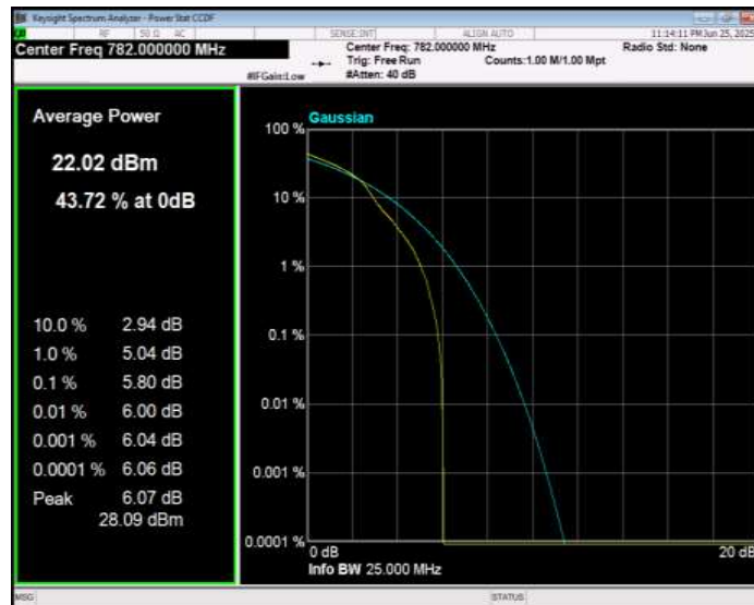
Band13 16QAM BW=5MHz Channel=23205 RB Size=1 Position=#0
