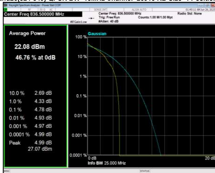
Band26(824-849) QPSK BW=15MHz Channel=26965 RB Size=1 Position=#0
