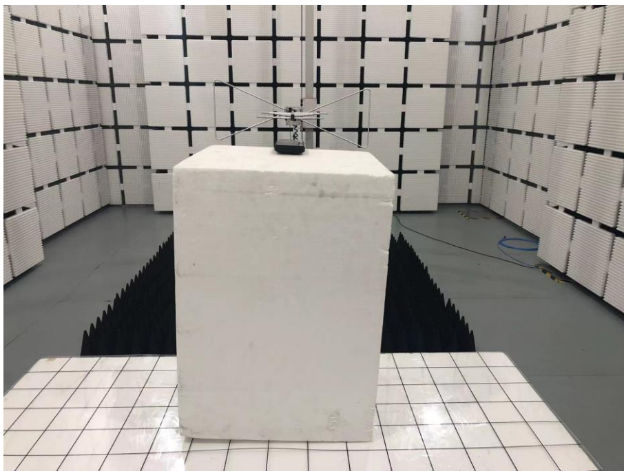
Radiated Spurious Emission Test Setup Photo - Below 1GHz(30MHz- 1000MHz)
