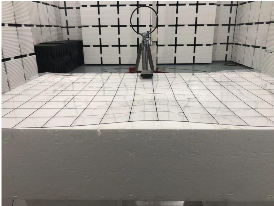
Radiated Spurious Emission Test Setup Photo - Below 1GHz(30MHz- 1000MHz)
