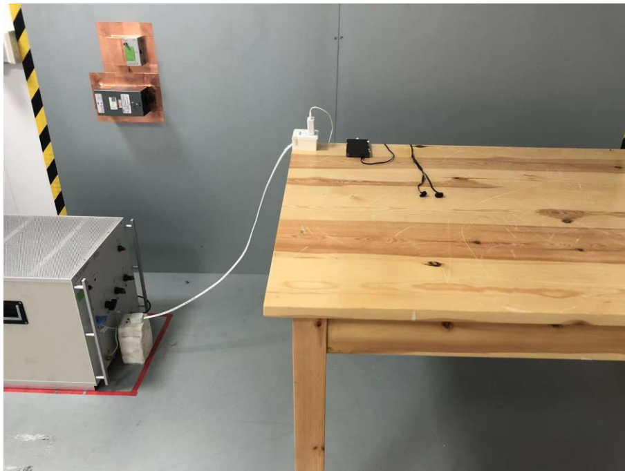
Conducted Emission Test Setup Photo
