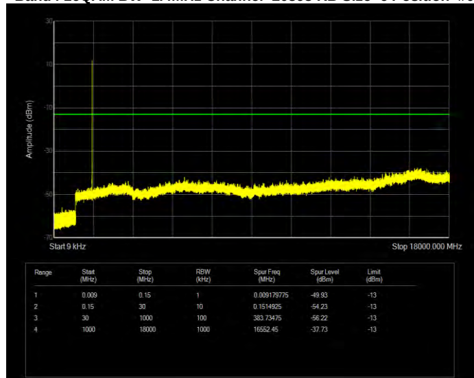
Band4 16QAM BW=1.4MHz Channel=20393 RB Size=6 Position=#0
