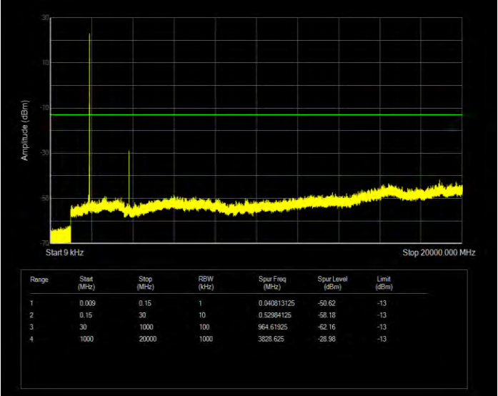
Band25 16QAM BW=10MHz Channel=26090 RB Size=50 Position=#0
