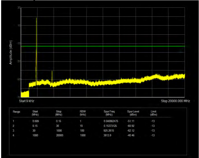
Band25 16QAM BW=3MHz Channel=26055 RB Size=15 Position=#0
