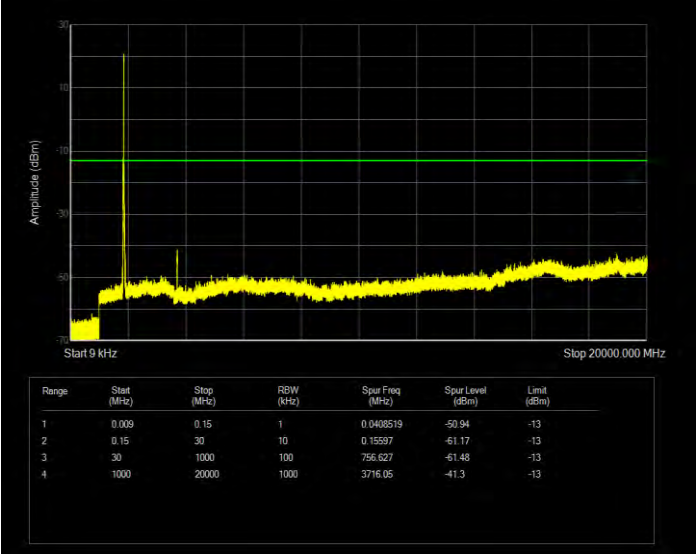
Band25 16QAM BW=10MHz Channel=26090 RB Size=50 Position=#0
