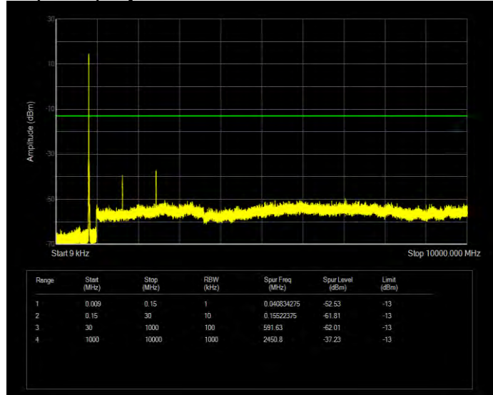
Band26(814-824) 16QAM BW=5MHz Channel=26740 RB Size=25 Position=#0
