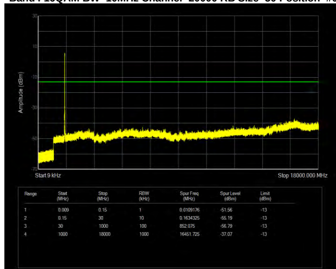
Band4 16QAM BW=10MHz Channel=20175 RB Size=50 Position=#0
