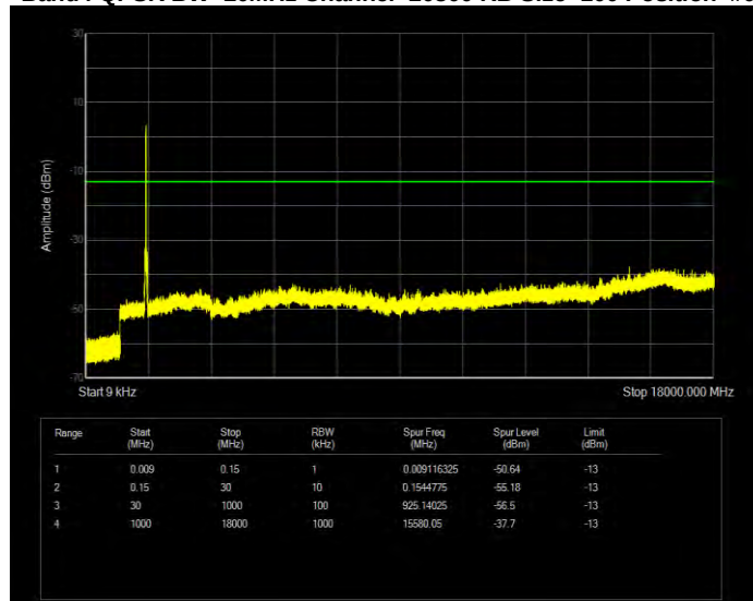
Band4 QPSK BW=20MHz Channel=20300 RB Size=100 Position=#0
