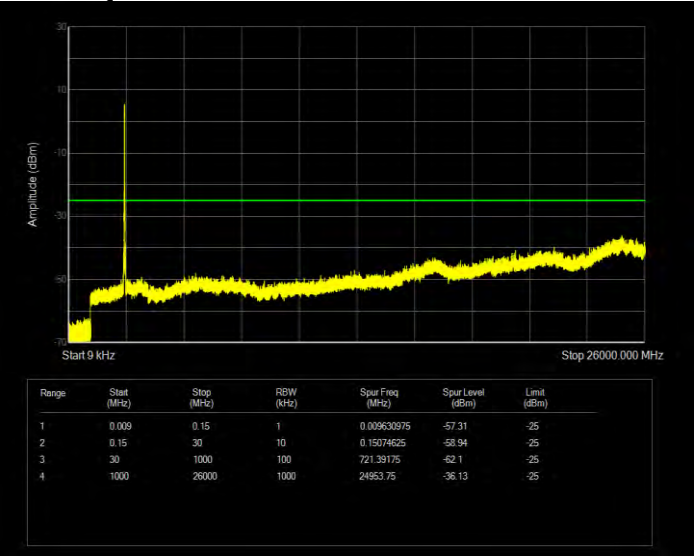
Band7 16QAM BW=20MHz Channel=21350 RB Size=100 Position=#0
