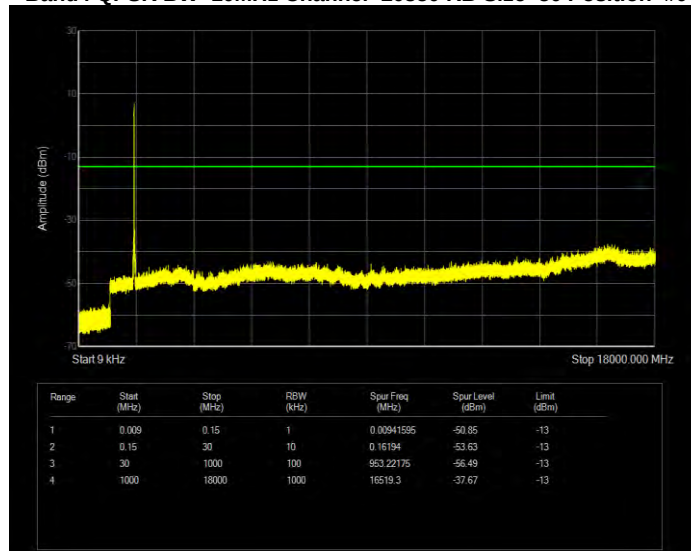
Band4 QPSK BW=10MHz Channel=20350 RB Size=50 Position=#0
