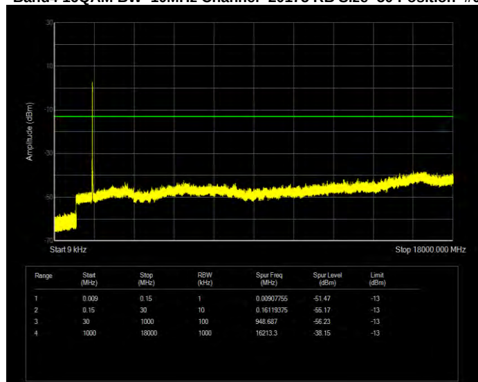
Band4 16QAM BW=10MHz Channel=20350 RB Size=50 Position=#0
