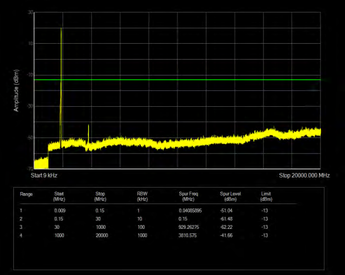
Band25 QPSK BW=3MHz Channel=26055 RB Size=15 Position=#0
