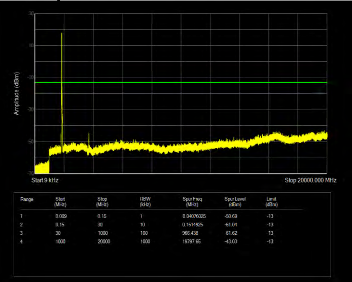
Band25 16QAM BW=20MHz Channel=26140 RB Size=100 Position=#0
