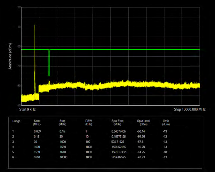
Band13 16QAM BW=5MHz Channel=23205 RB Size=25 Position=#0
