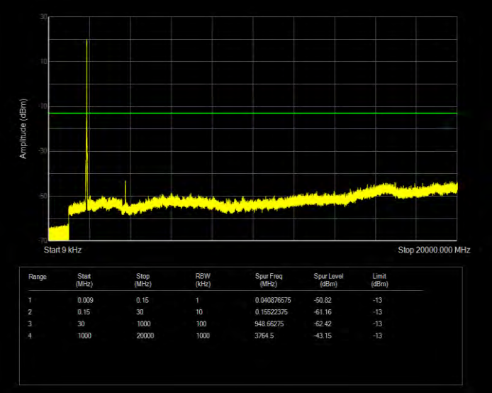
Band25 16QAM BW=10MHz Channel=26640 RB Size=50 Position=#0
