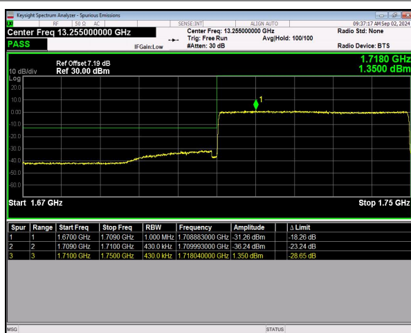
n66 SCS=15kHz CP_QPSK BW=40MHz LowChannel=346000 RB=216@0 NVNT
