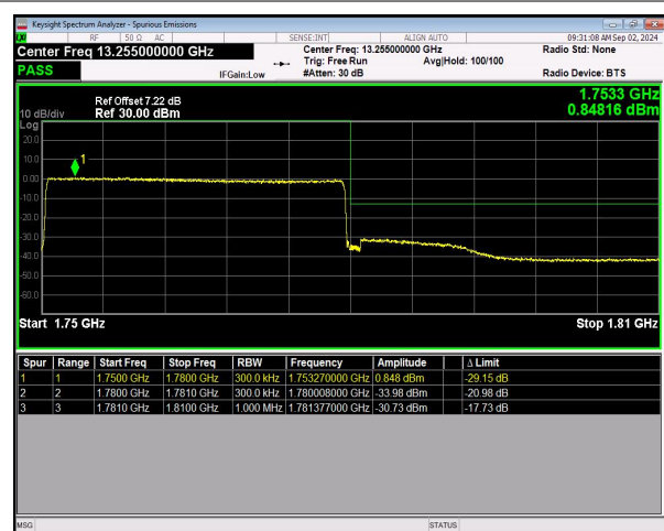
n66 SCS=15kHz CP_QPSK BW=30MHz HighChannel=353000 RB=160@0 NVNT
