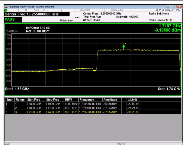
n66 SCS=15kHz DFT_256QAM BW=30MHz LowChannel=345000 RB=160@0 NVNT
