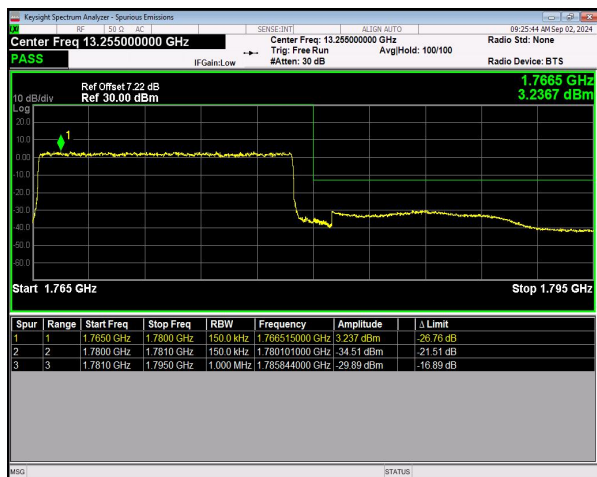
n66 SCS=15kHz DFT_BPSK BW=15MHz HighChannel=354500 RB=75@0 NVNT
