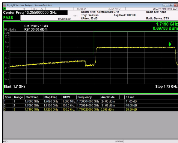
n66 SCS=15kHz CP_QPSK BW=10MHz LowChannel=343000 RB=52@0 NVNT
