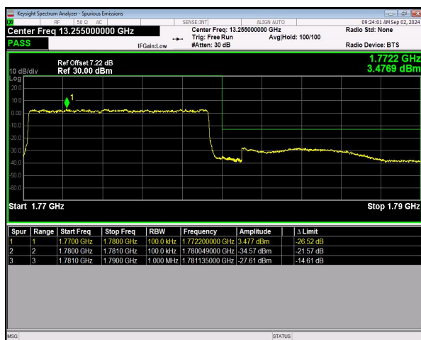
n66 SCS=15kHz DFT_BPSK BW=10MHz HighChannel=355000 RB=50@0 NVNT
