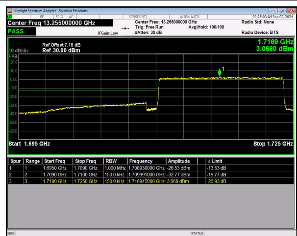
n66 SCS=15kHz DFT_QPSK BW=15MHz LowChannel=343500 RB=75@0 NVNT
