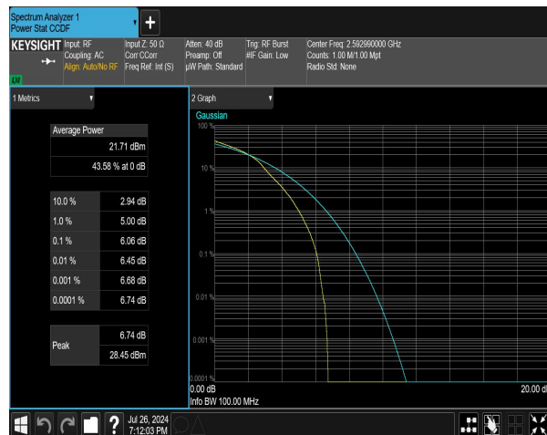
n41 SCS=30kHz DFT_16QAM BW=15MHz Channel=518598 RB=36@0 NVNT
