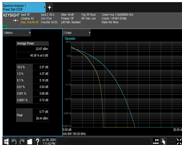
n41 SCS=30kHz DFT_QPSK BW=10MHz Channel=518598 RB=24@0 NVNT
