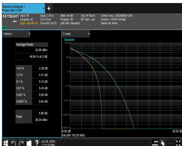
n41 SCS=30kHz DFT_QPSK BW=30MHz Channel=518598 RB=75@0 NVNT
