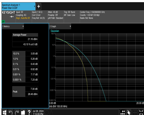
n41 SCS=30kHz DFT_64QAM BW=15MHz Channel=518598 RB=36@0 NVNT
