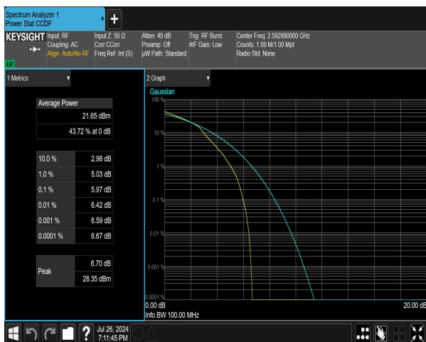
n41 SCS=30kHz DFT_16QAM BW=10MHz Channel=518598 RB=24@0 NVNT
