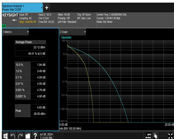
n41 SCS=30kHz DFT_BPSK BW=40MHz Channel=518598 RB=100@0 NVNT
