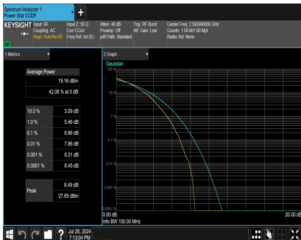
n41 SCS=30kHz DFT_256QAM BW=40MHz Channel=518598 RB=100@0 NVNT
