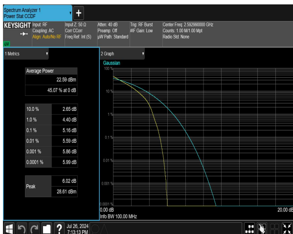
n41 SCS=30kHz DFT_QPSK BW=50MHz Channel=518598 RB=128@0 NVNT
