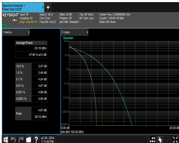
n41 SCS=30kHz DFT_BPSK BW=10MHz Channel=518598 RB=24@0 NVNT
