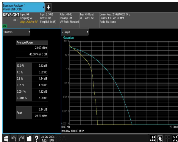
n41 SCS=30kHz DFT_BPSK BW=50MHz Channel=518598 RB=128@0 NVNT
