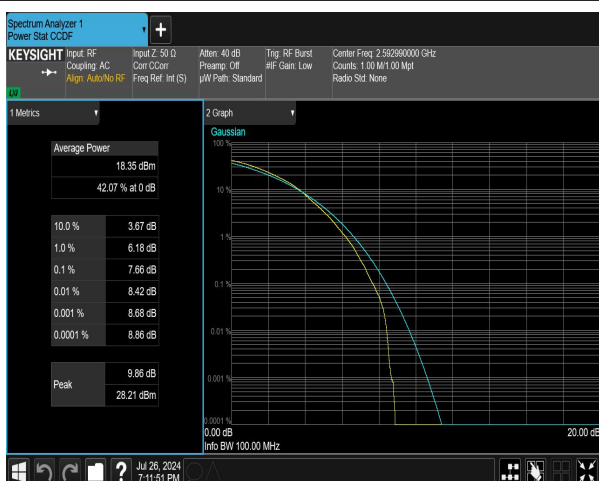
n41 SCS=30kHz DFT_256QAM BW=10MHz Channel=518598 RB=24@0 NVNT
