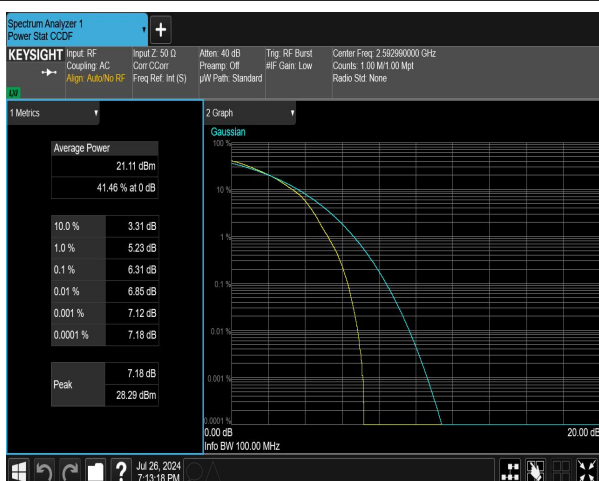
n41 SCS=30kHz DFT_64QAM BW=50MHz Channel=518598 RB=128@0 NVNT
