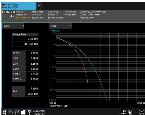
n41 SCS=30kHz DFT_64QAM BW=30MHz Channel=518598 RB=75@0 NVNT
