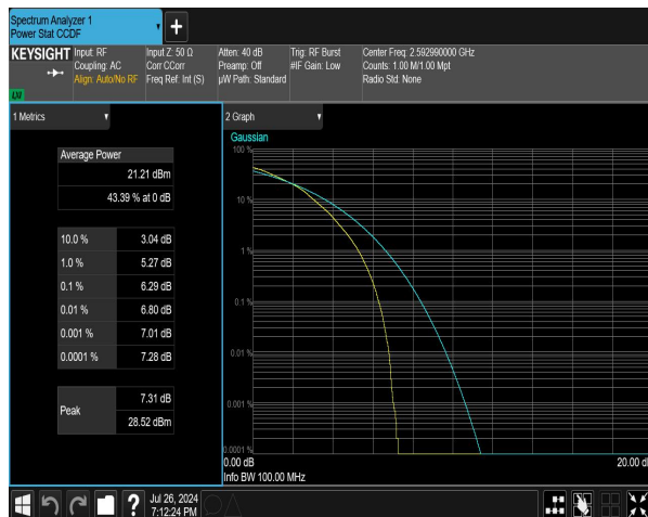
n41 SCS=30kHz DFT_64QAM BW=20MHz Channel=518598 RB=50@0 NVNT
