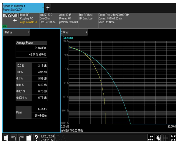
n41 SCS=30kHz DFT_16QAM BW=50MHz Channel=518598 RB=128@0 NVNT
