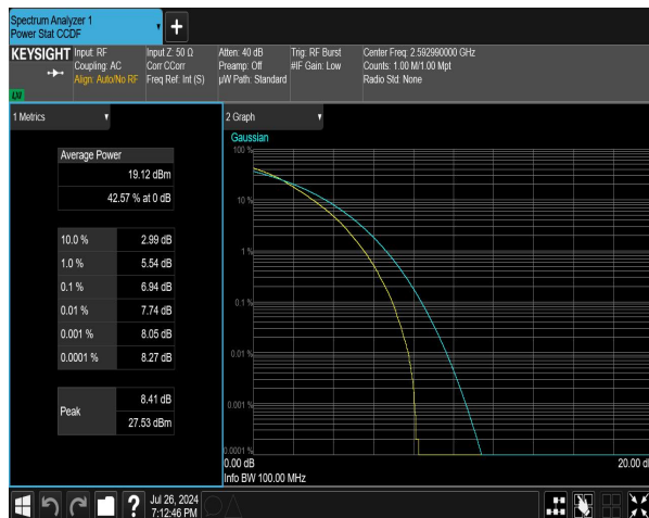
n41 SCS=30kHz DFT_256QAM BW=30MHz Channel=518598 RB=75@0 NVNT
