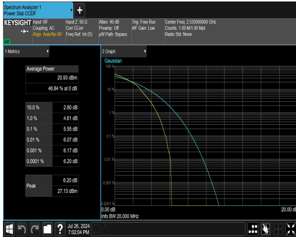
n7 SCS=15kHz DFT_16QAM BW=15MHz Channel=507000 RB=75@0 NVNT
