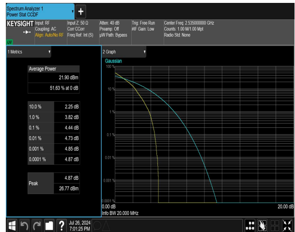
n7 SCS=15kHz DFT_QPSK BW=5MHz Channel=507000
