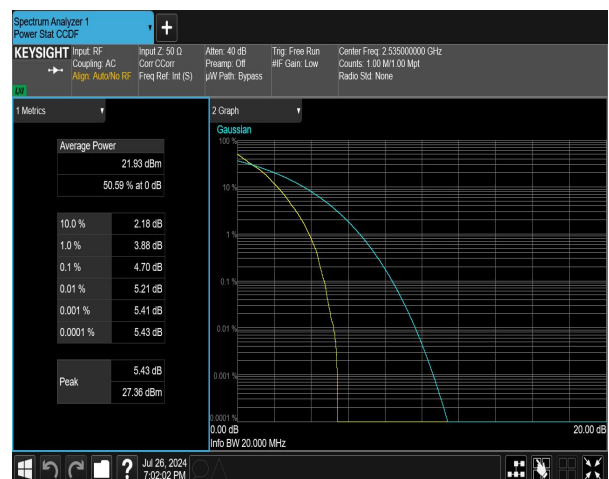
n7 SCS=15kHz DFT_QPSK BW=15MHz Channel=507000 RB=75@0 NVNT
