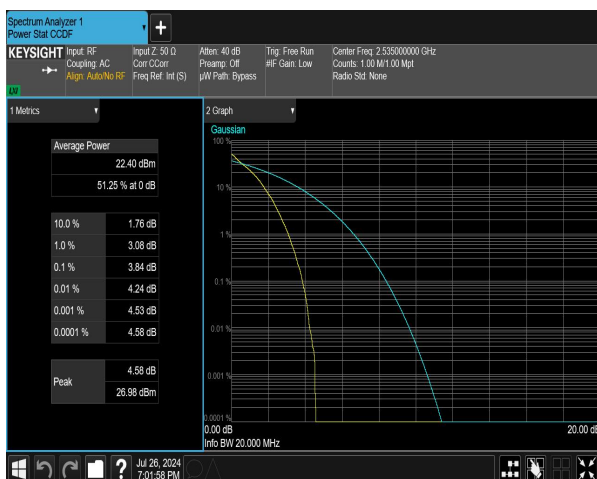
n7 SCS=15kHz DFT_BPSK BW=15MHz Channel=507000 RB=75@0 NVNT
