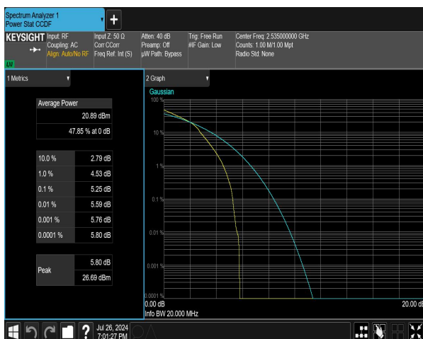
n7 SCS=15kHz DFT_16QAM BW=5MHz Channel=507000
