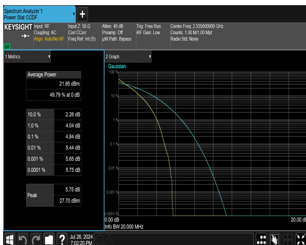
n7 SCS=15kHz DFT_QPSK BW=20MHz Channel=507000 RB=100@0 NVNT
