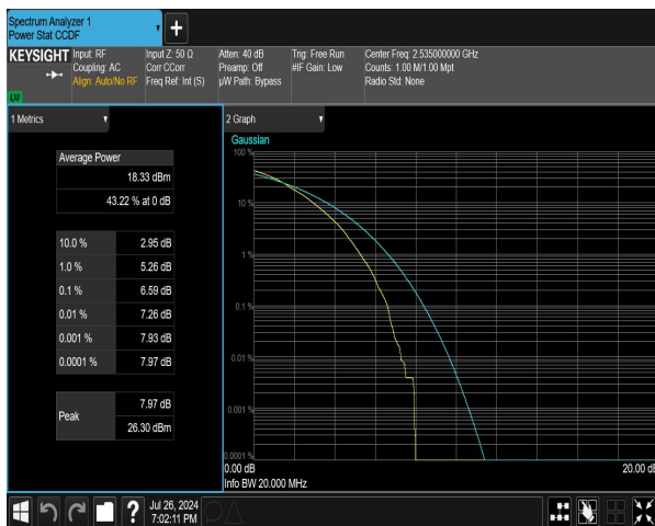
n7 SCS=15kHz DFT_256QAM BW=15MHz Channel=507000 RB=75@0 NVNT
