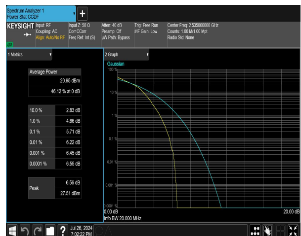
n7 SCS=15kHz DFT_16QAM BW=20MHz Channel=507000 RB=100@0 NVNT
