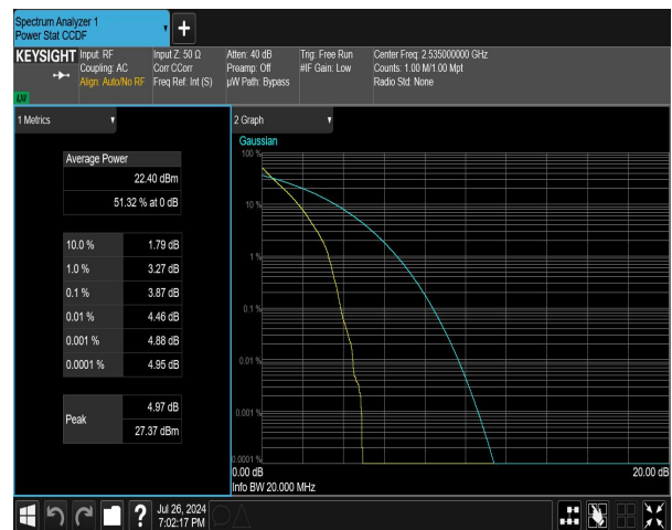
n7 SCS=15kHz DFT_BPSK BW=20MHz Channel=507000 RB=100@0 NVNT
