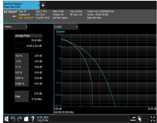
n7 SCS=15kHz DFT_64QAM BW=15MHz Channel=507000 RB=75@0 NVNT
