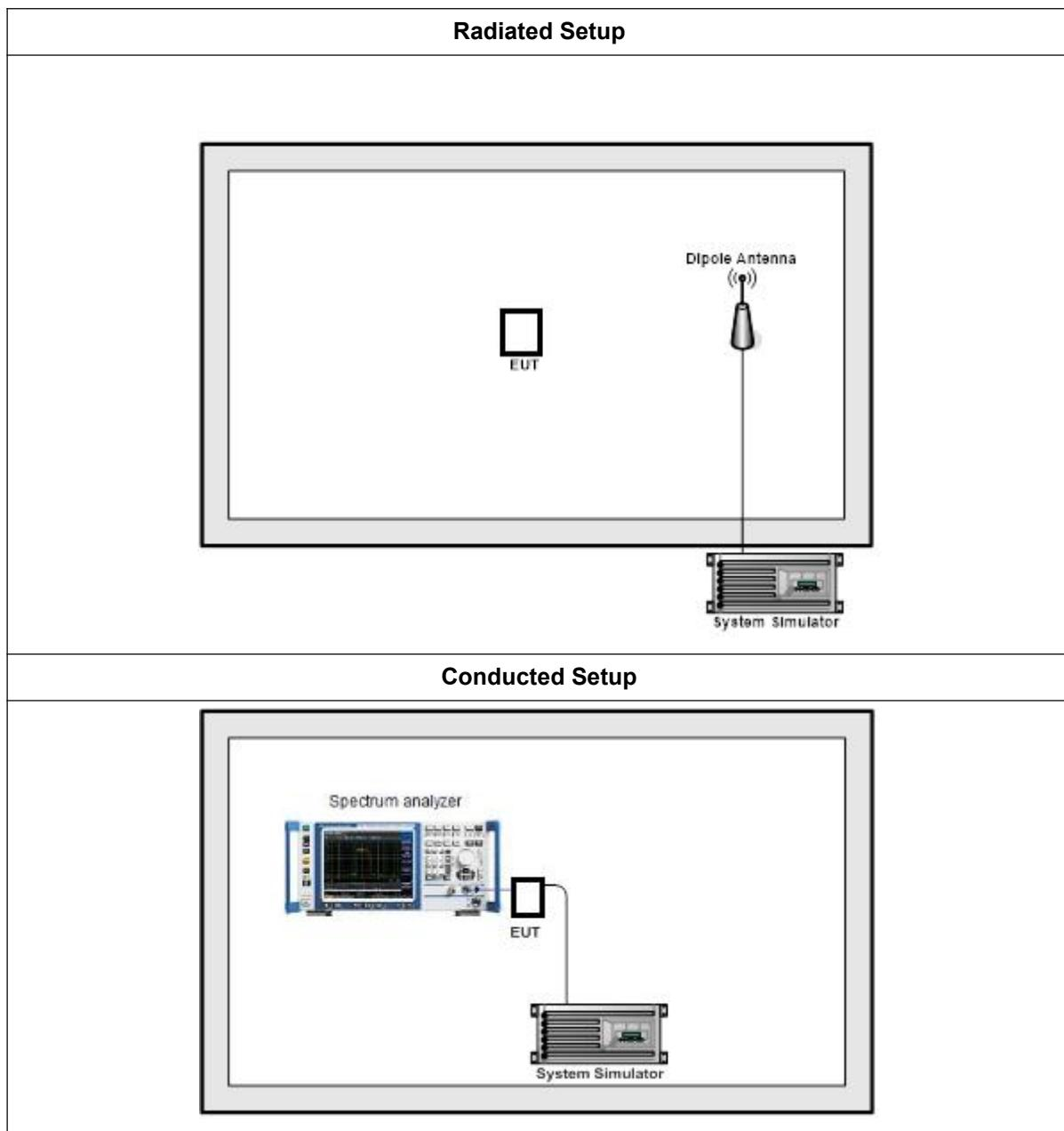
**Note:** This example is connection diagram of EUT test configurations. For detail, please refer to test mode configuration and setup photographs for each test item.
