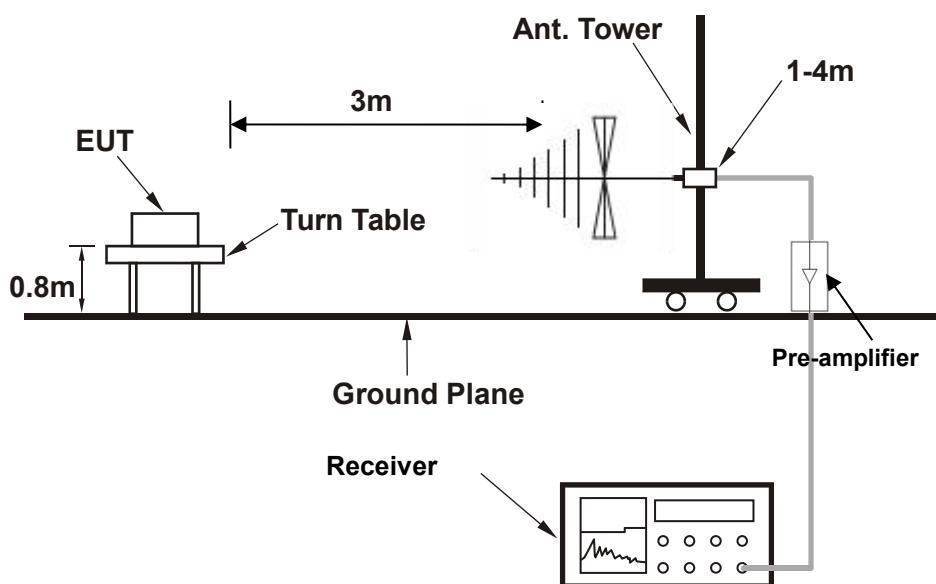
**For radiated test from 1GHz to 18GHz**
