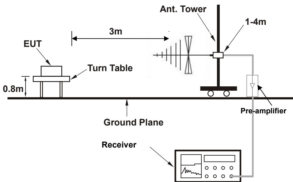
**For radiated test from 1GHz to 18GHz**
