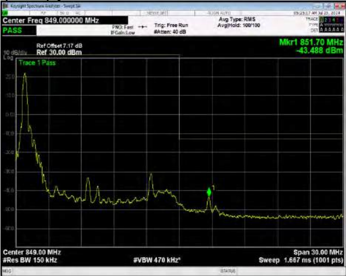
Band26(824-849) QPSK BW=15MHz Channel=26965 RB Size=1 Position=#Max Extended
