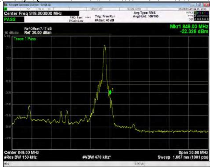
Band26(824-849) 16QAM BW=15MHz Channel=26965 RB Size=75 Position=#0 Extended
