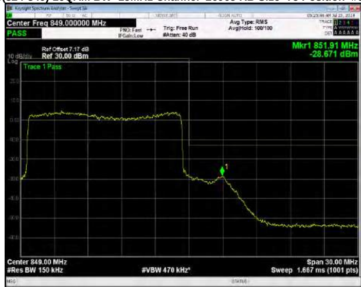
Band26(824-849) 16QAM BW=15MHz Channel=26965 RB Size=75 Position=#0 Normal
