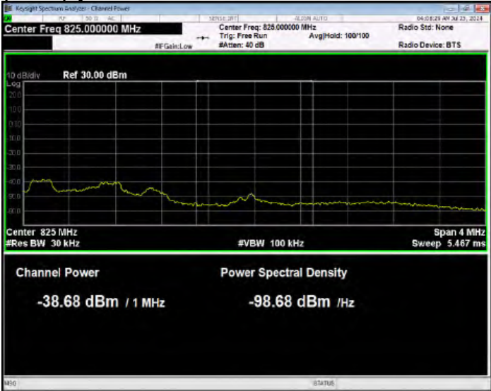
Band26(814-824) QPSK BW=3MHz Channel=26775 RB Size=1 Position=#0 Normal
