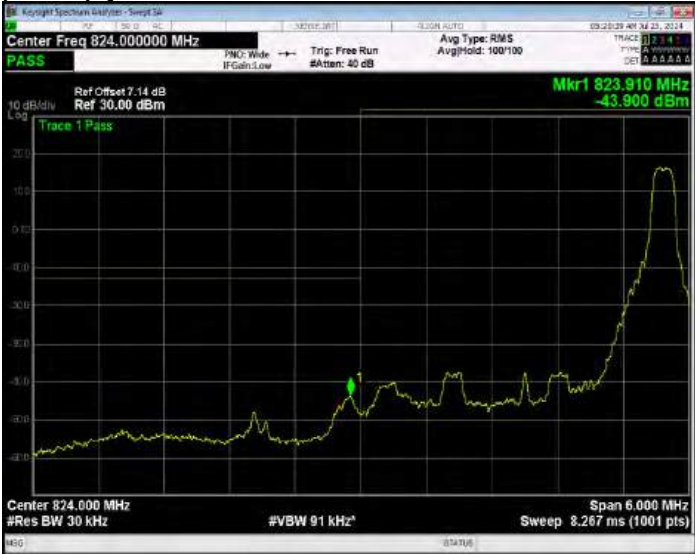
Band26(824-849) QPSK BW=3MHz Channel=26805 RB Size=15 Position=#0 Extended
