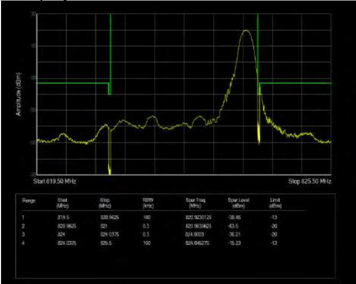
Band26(814-824) 16QAM BW=3MHz Channel=26775 RB Size=15 Position=#0 Extended
