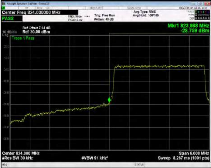
Band26(824-849) QPSK BW=3MHz Channel=26805 RB Size=15 Position=#0 Normal
