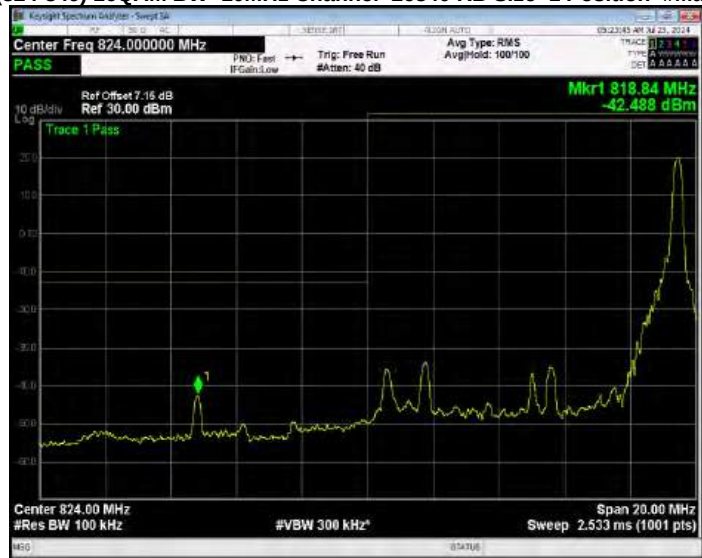
Band26(824-849) 16QAM BW=10MHz Channel=26840 RB Size=50 Position=#0 Extended
