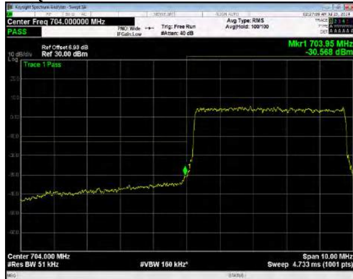
Band17 QPSK BW=5MHz Channel=23755 RB Size=25 Position=#0 Normal
