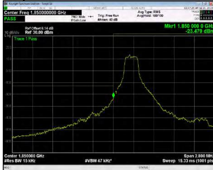
Band25 QPSK BW=1.4MHz Channel=26047 RB Size=1 Position=#Max Extended
