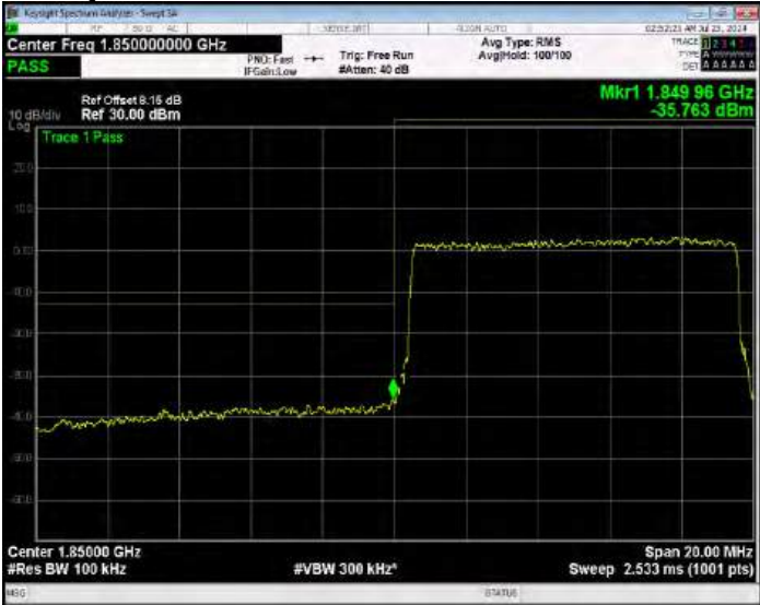
Band25 16QAM BW=10MHz Channel=26090 RB Size=50 Position=#0 Normal
