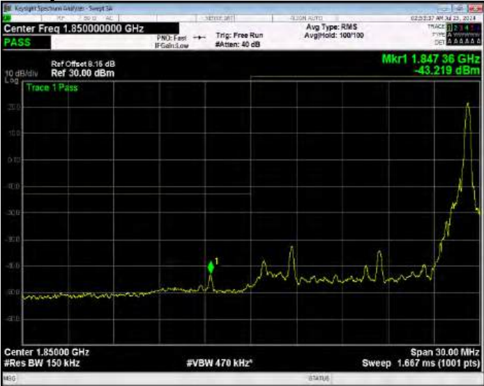
Band25 16QAM BW=15MHz Channel=26115 RB Size=75 Position=#0 Extended
