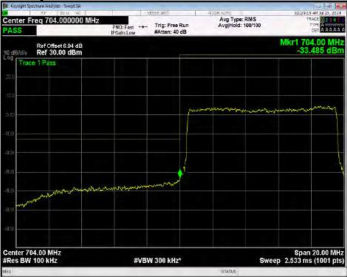
Band17 16QAM BW=10MHz Channel=23780 RB Size=50 Position=#0 Normal
