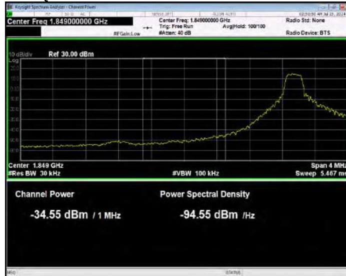
Band25 16QAM BW=5MHz Channel=26065 RB Size=1 Position=#0 Normal
