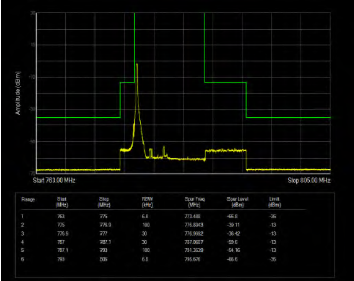
Band13 QPSK BW=5MHz Channel=23205 RB Size=1 Position=#Max Extended
