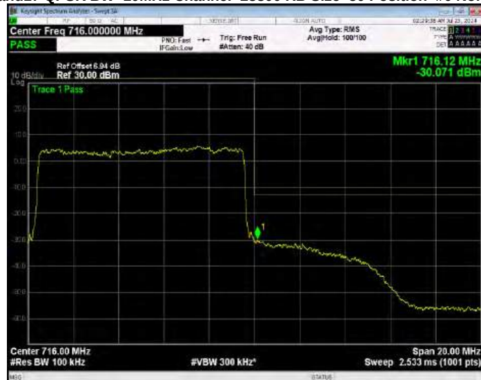
Band17 QPSK BW=10MHz Channel=23800 RB Size=50 Position=#0 Normal
