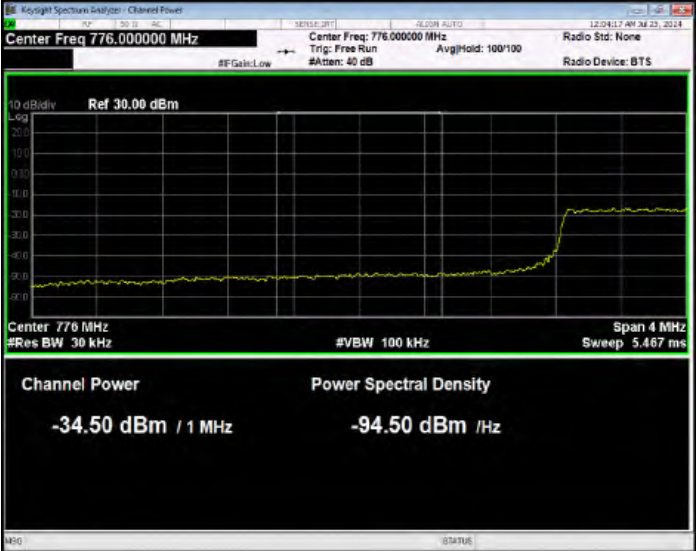
Band13 QPSK BW=5MHz Channel=23205 RB Size=25 Position=#0 Normal
