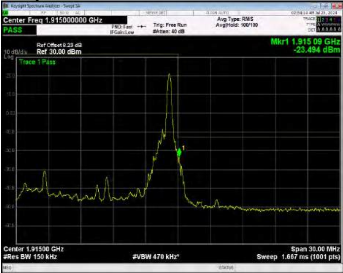
Band25 16QAM BW=15MHz Channel=26615 RB Size=75 Position=#0 Extended
