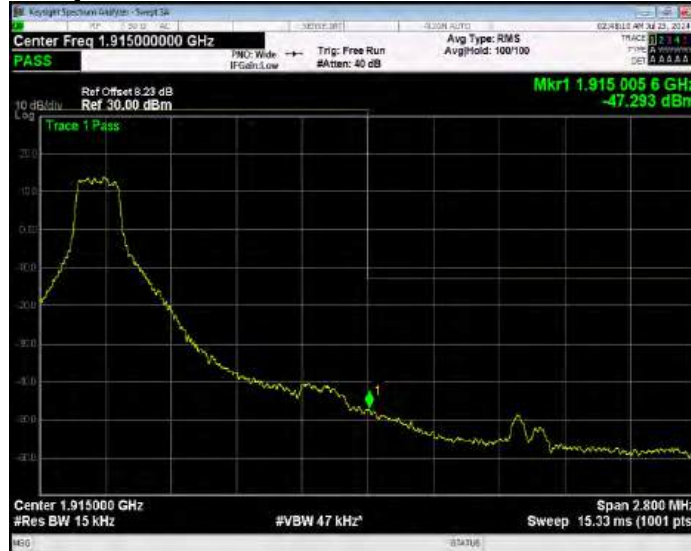
Band25 QPSK BW=1.4MHz Channel=26683 RB Size=1 Position=#Max Extended
