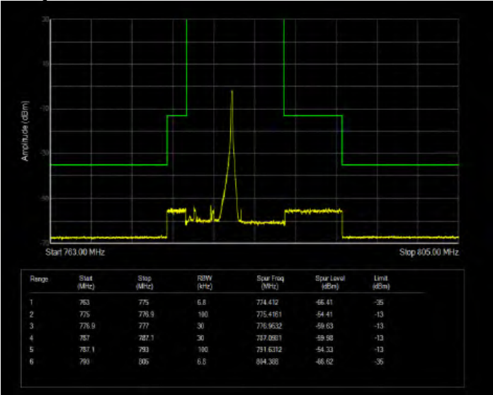
Band13 QPSK BW=5MHz Channel=23205 RB Size=25 Position=#0 Extended
