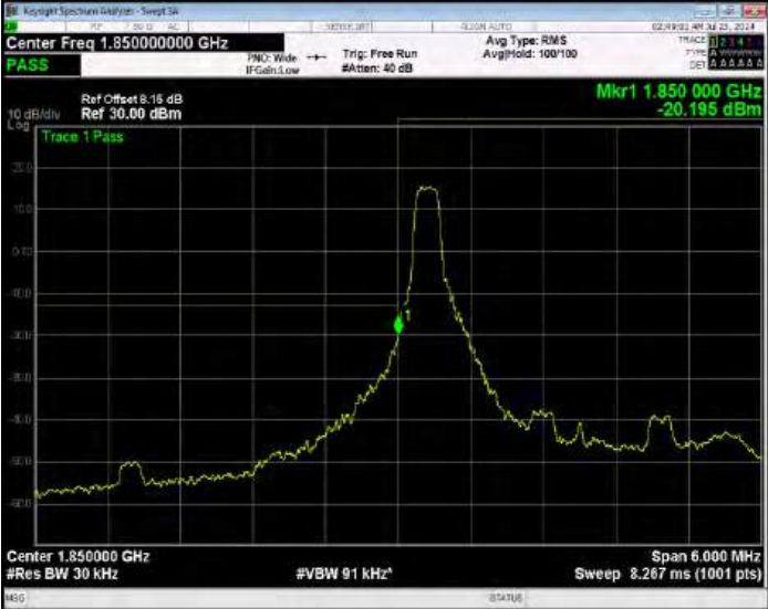
Band25 QPSK BW=3MHz Channel=26055 RB Size=1 Position=#Max Extended
