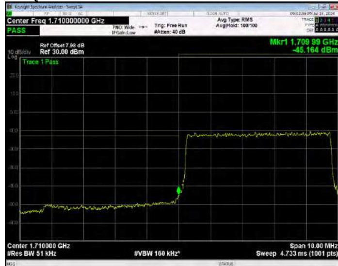
Band4 QPSK BW=5MHz Channel=19975 RB Size=25 Position=#0 Normal
