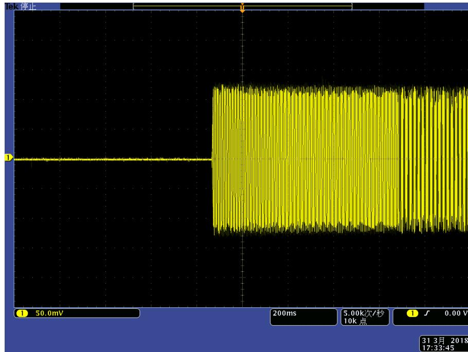
Transmitter Frequency Behaviour @ 12.5 KHz Channel Separation-----On – Off
