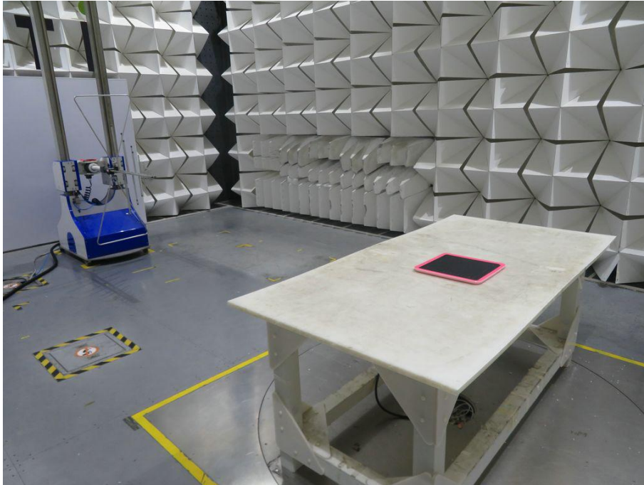
Radiated spurious emission Test Setup-1(Below 1GHz)
