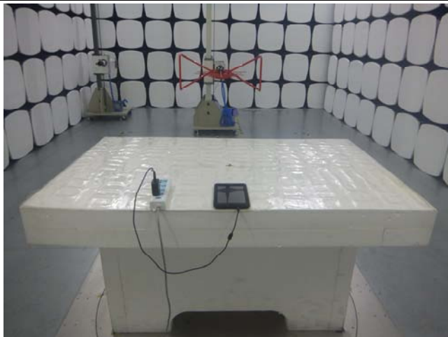
Radiated Spurious Emissions Test Setup Below 1GHz
