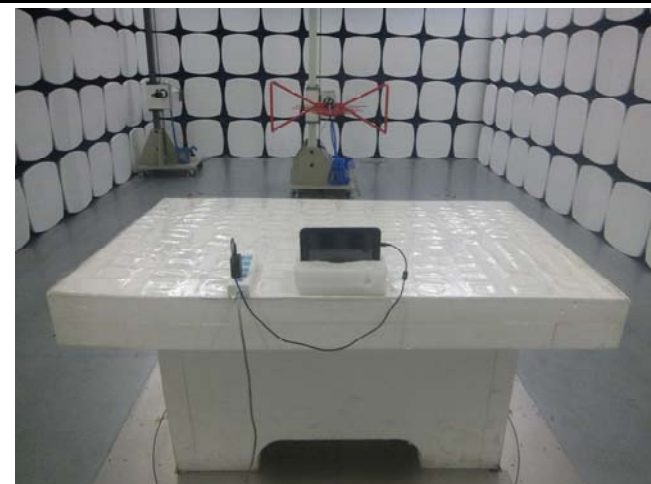
Conducted Emissions Test Setup Front View
