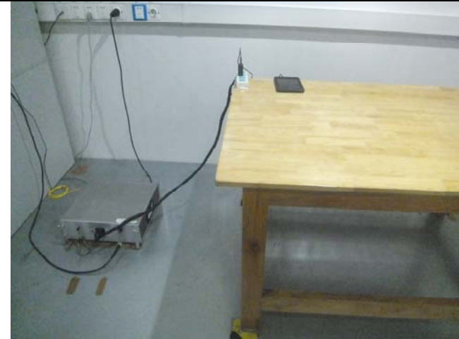
Conducted Emissions Test Setup Front View
