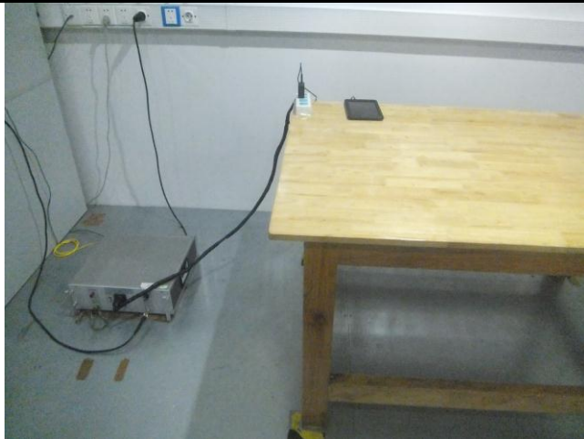
Conducted Emissions Test Setup Front View
