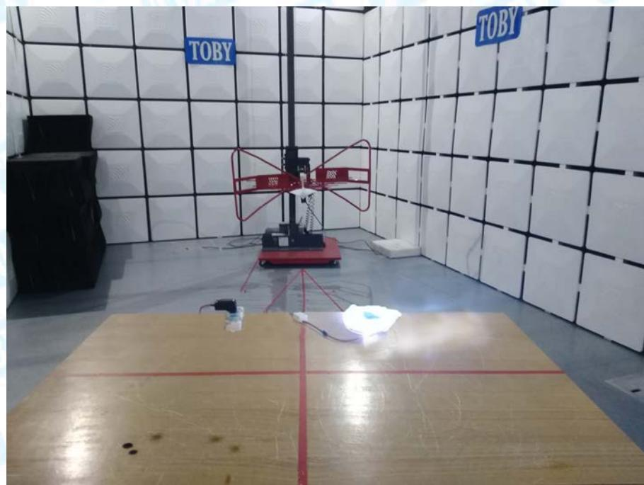
**Photo of Setup for Conduct Emission**
