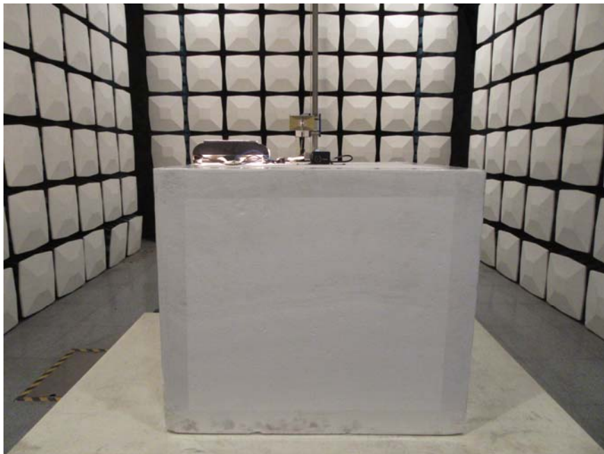
Radiated Disturbance Test Setup View (Above 1GHz)
